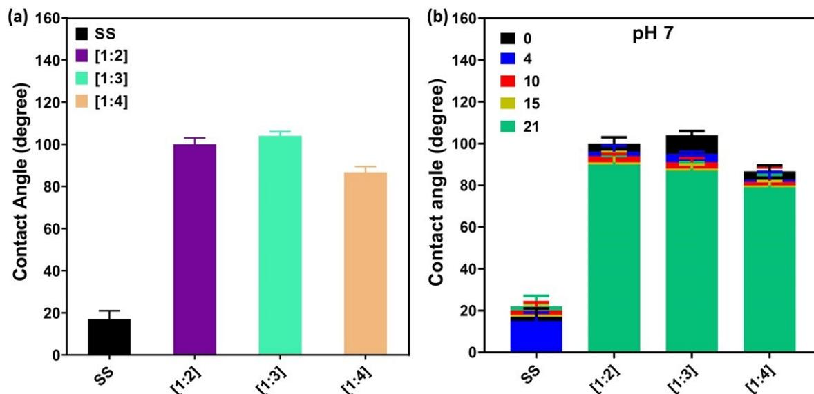
**Figure 10. (a)** Contact angles of uncoated and polymer coated SS surfaces. **(b)** Long-term stability study of copolymers coated SS along with uncoated SS surfaces (control) as measured by their static contact angles under the water rinsing conditions: neutral solution (milli-Q water). The SCA was measured after formation (black), and water rinsing after 4 days (blue), 10 days (red), 15 days (yellow), and 21 days (green). Data are presented as mean  $\pm$  standard deviation (N=3).
