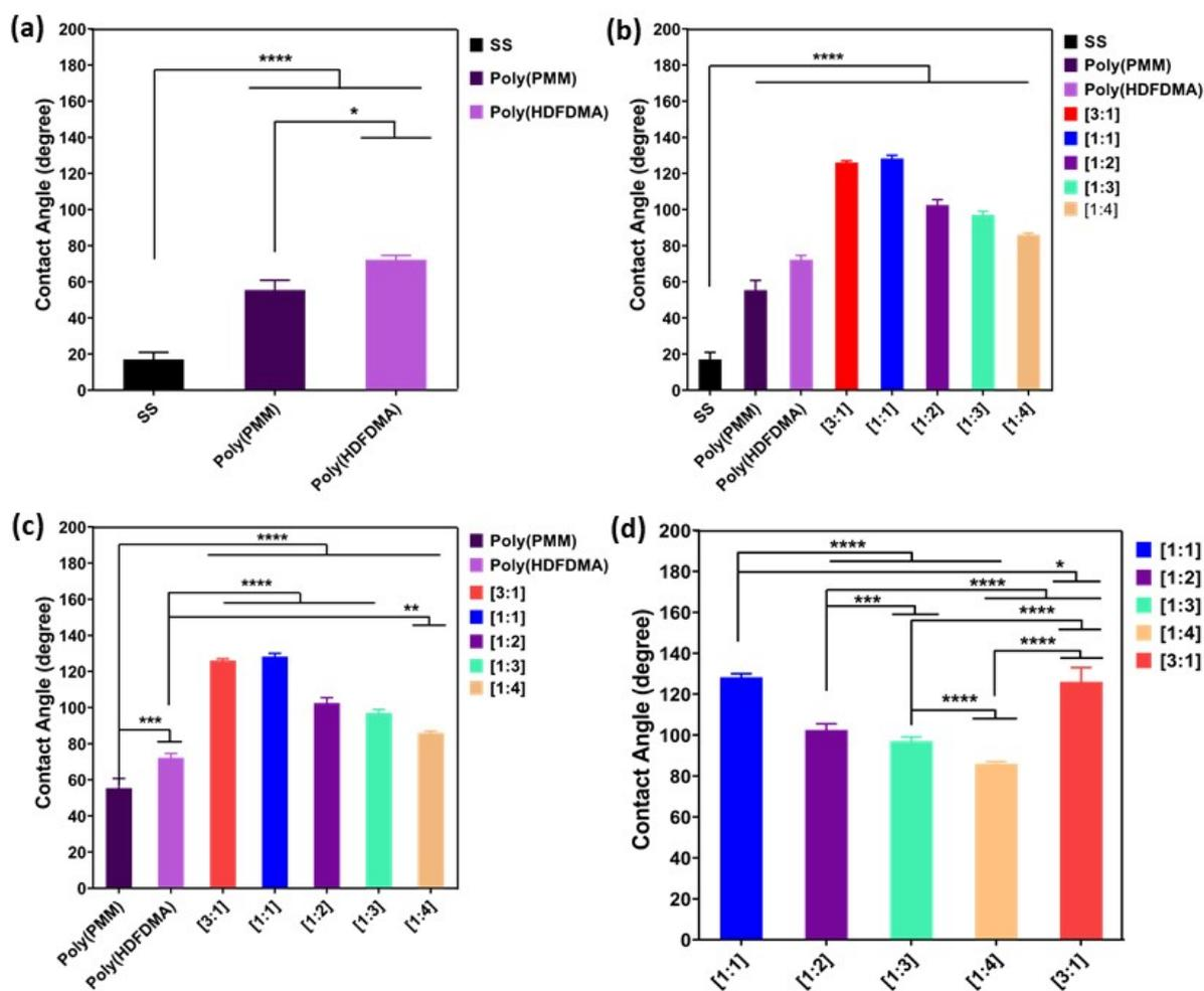
**Figure S9.** Contact angles of uncoated and polymer coated SS surfaces. The films were deposited from TFA at a concentration of 1 wt. % of the polymer solution. \*\*\*\*  $P < 0.0001$ , \*\*\*  $P = 0.001$ , \*\*  $P < 0.01$ , \*  $P < 0.05$ . Data are presented as mean  $\pm$  standard deviation (N=3).
