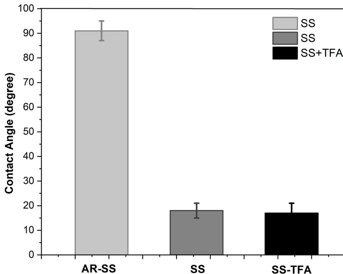
**Figure S8.** Water contact angles on as-received (AR-SS) surface, chromic acid cleaned (SS) surface, and chromic acid cleaned and immersed in TFA for 30 minutes (SS-TFA) surfaces. Data are presented as mean  $\pm$  standard deviation (N=3).
