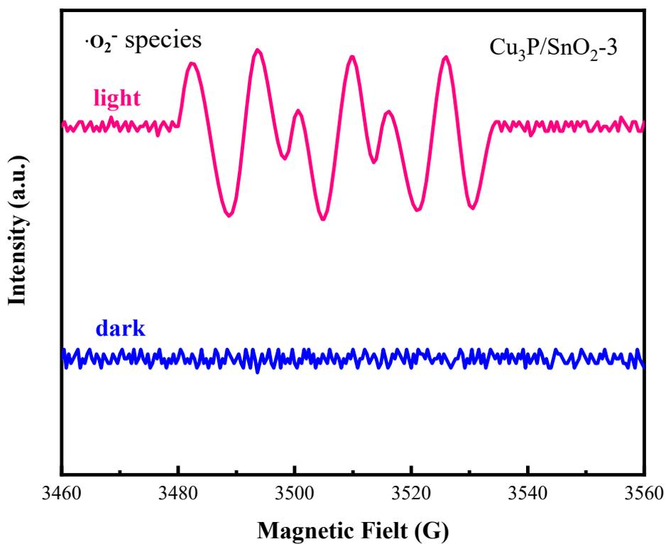
Fig. S2 ESR tests for the  $\cdot\text{O}_2^-$  species during different catalytic processes
