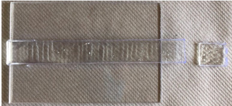
Fig. S2: Failed representative specimen of cured resin on methacryloxypropyltriethoxysilane (MAPTES)-functionalized surfaces during 90° peel test.
