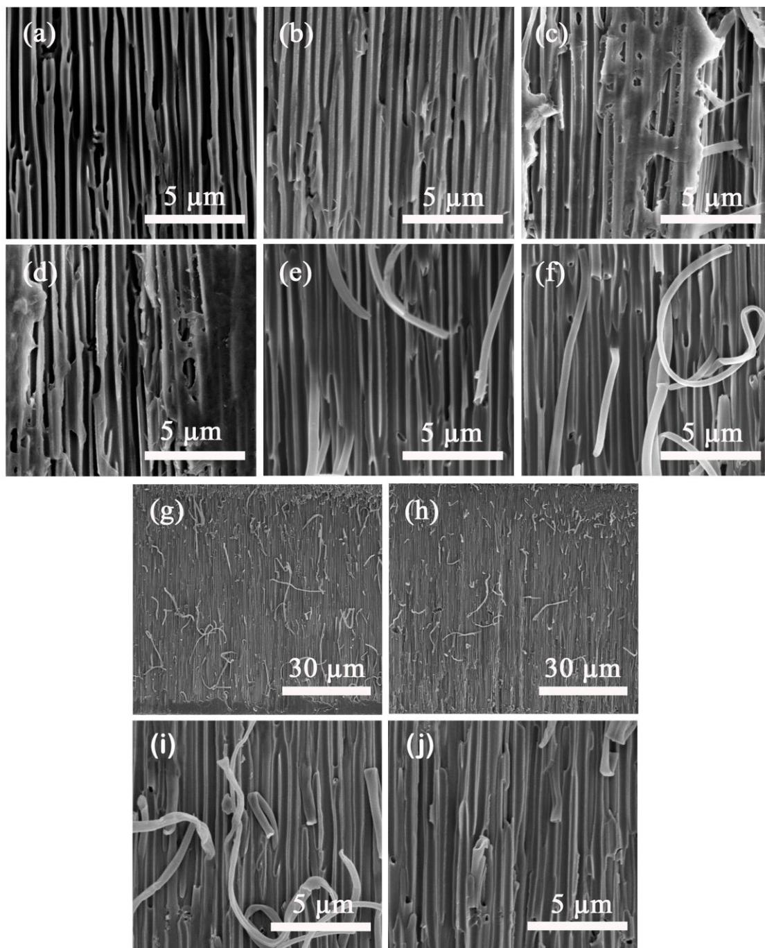
Figure S1 SEM images of TpBD COF/AAO membrane synthesized by Tp and BD under different reaction times. (a) 1 h. (b) 2 h. (c) 3 h. (d) 4 h. (e) 5 h. (f) 6 h. (g) and (i) 7 h. (h) and (j) 8 h.
