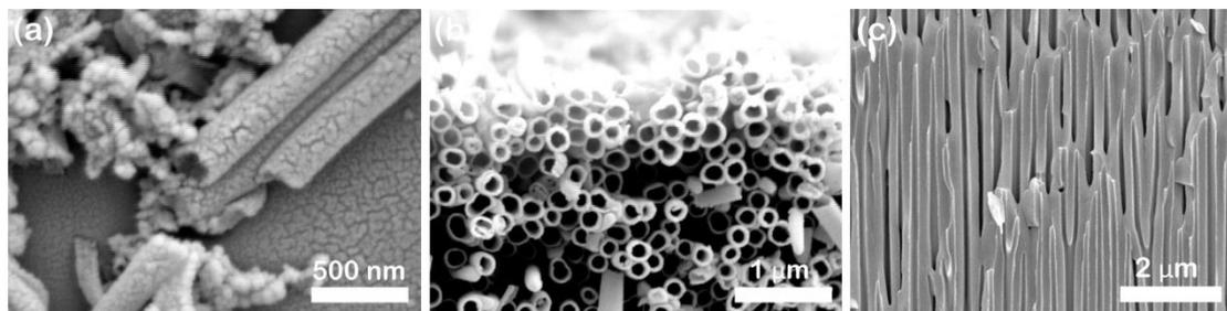
Figure S2 (a) The diameter of TpBD COF/AAO tubes; (b) The structure of COF tubes by removal AAO membrane in 0.1 M NaOH solution; (c) SEM images of AAO membrane.
