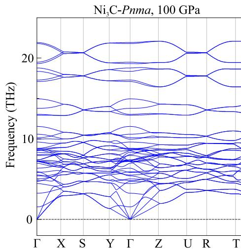
Figure S5: Phonon dispersion curves of  $\text{Ni}_3\text{C}$ - $Pnma$ .
