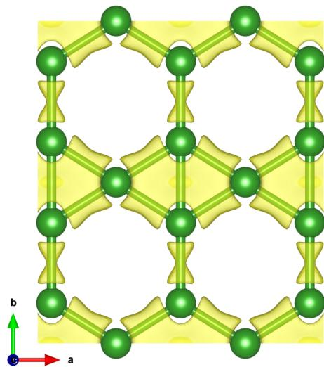
Figure S8: Electronic charge density distribution in infinite  $(001)$  layer of B atoms in the  $\text{Ni}_2\text{B}_3$  structure.
