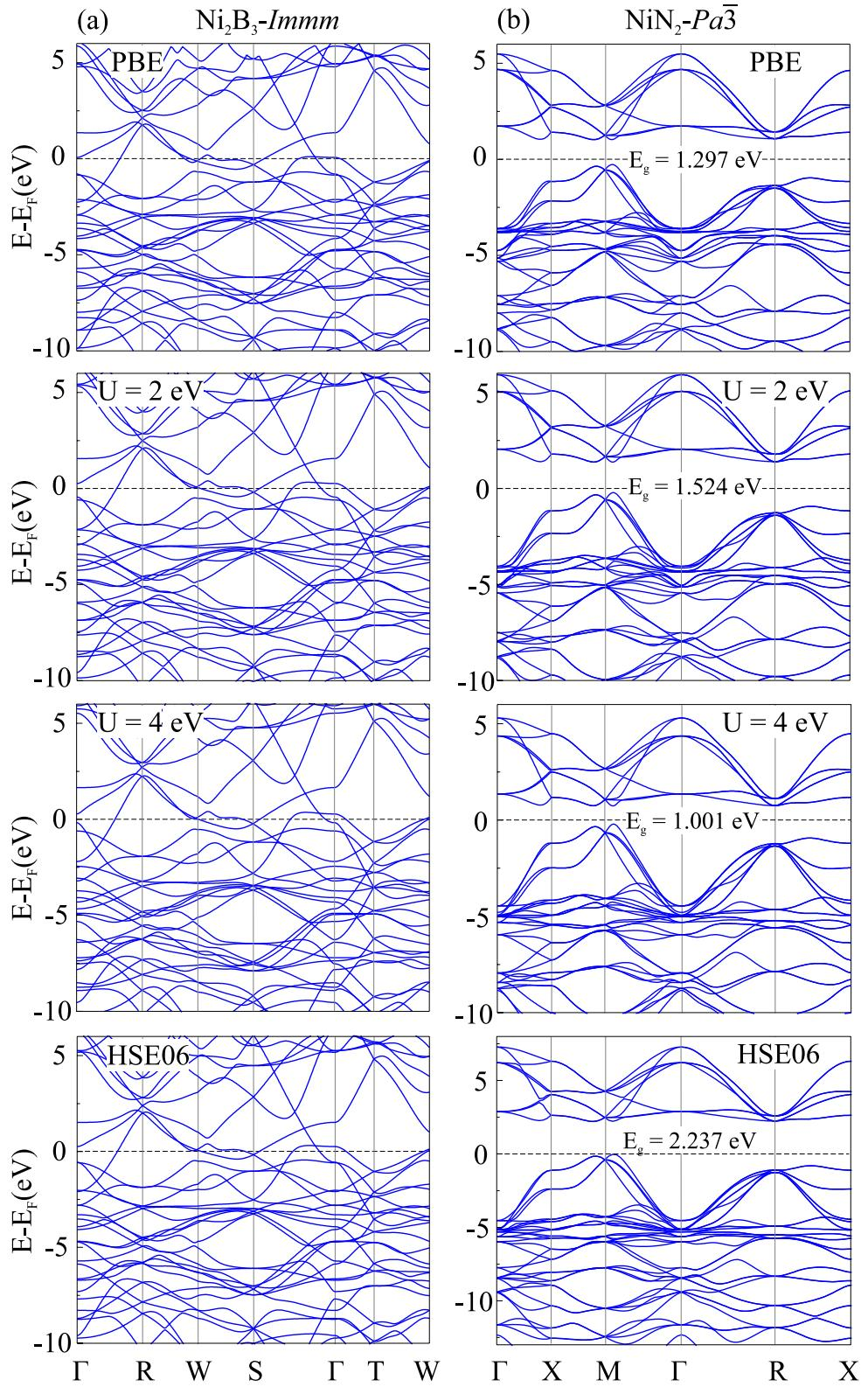
Figure S10: Band structures of  $\text{Ni}_2\text{B}_3$ -*Immm* (a) and  $\text{NiN}_2$ -*Pa\bar{3}* (b) calculated with PBE, GGA+U ( $U = 2, 4$  eV), and HSE06.
