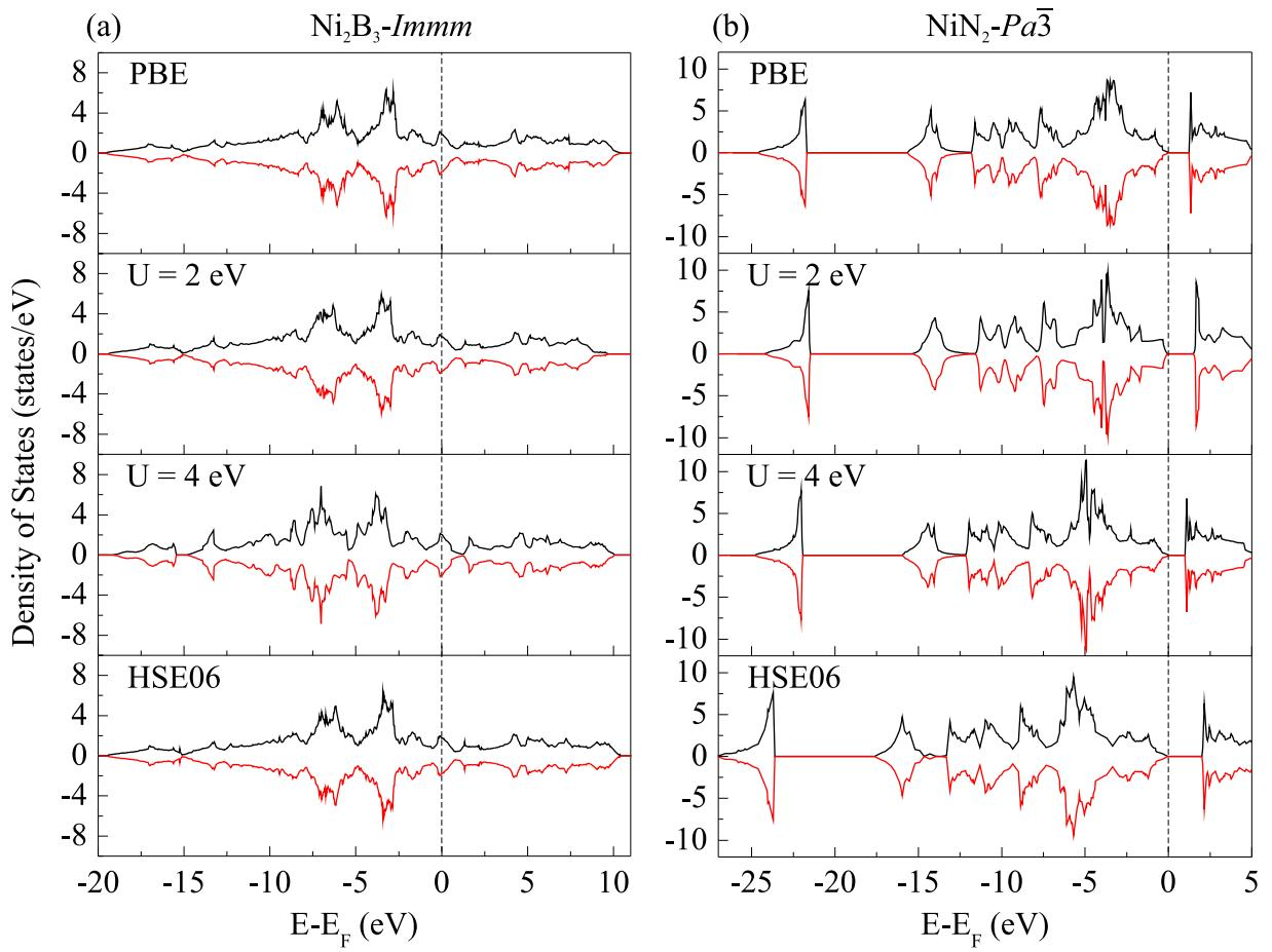
Figure S9: Total DOS of  $\text{Ni}_2\text{B}_3$ -*Immm* (a) and  $\text{NiN}_2$ -*Pa* $\bar{3}$  (b) calculated with PBE, GGA+U ( $U = 2, 4$  eV), and HSE06.
