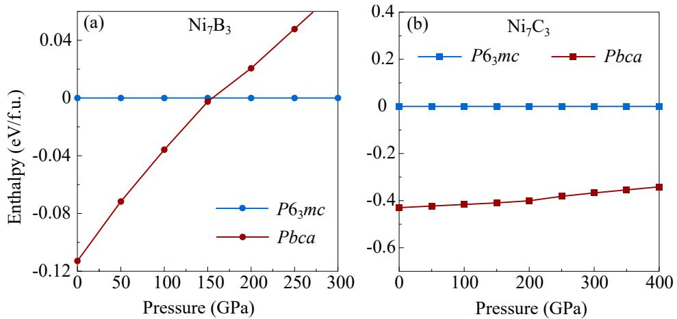
Figure S4: Enthalpy-pressure dependence for metastable phases Ni<sub>7</sub>B<sub>3</sub> (a) and Ni<sub>7</sub>C<sub>3</sub> (b).
