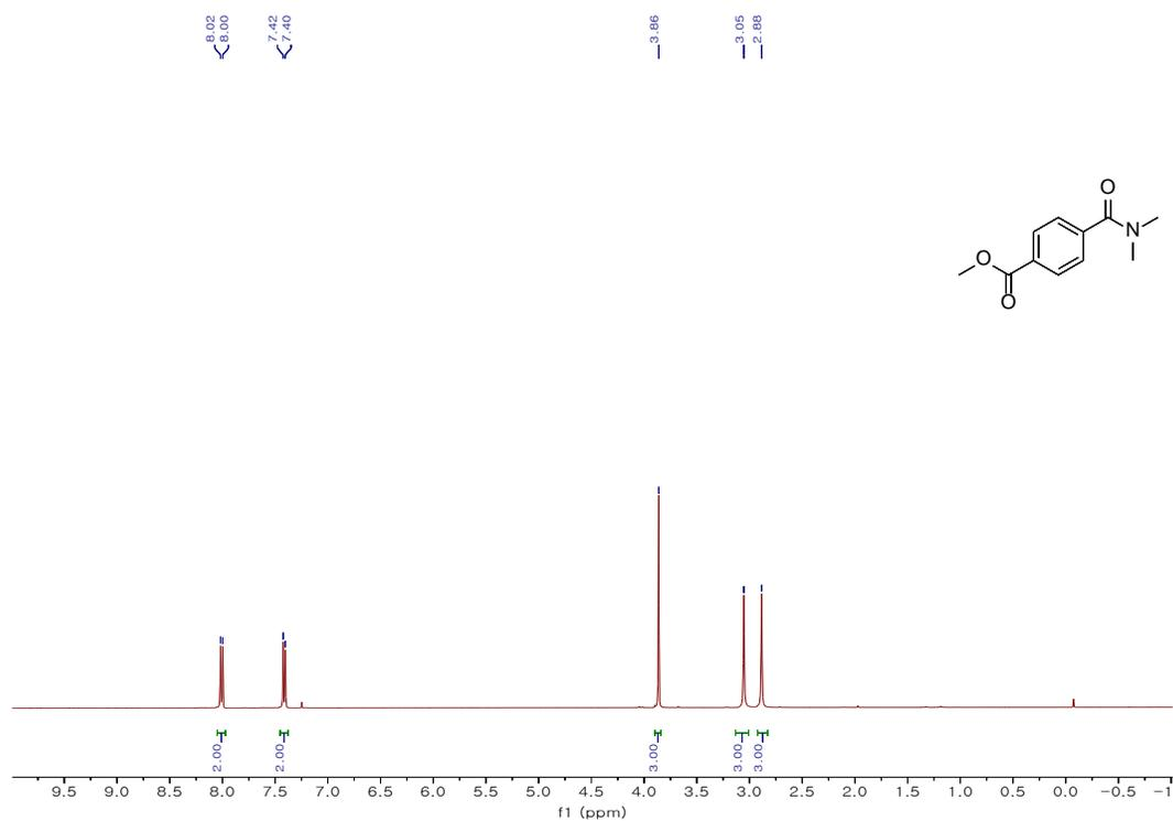
**Figure S5:**  $^1\text{H}$  NMR of Methyl 4-(dimethylcarbamoyl)benzoate (**1a**)
