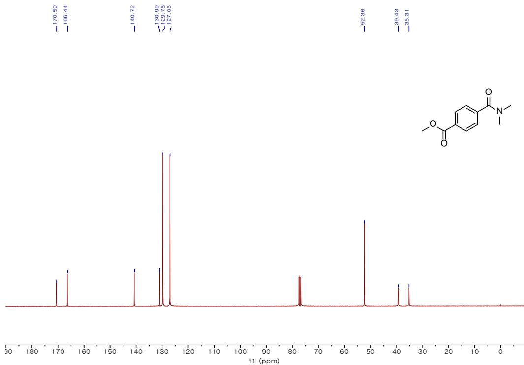
**Figure S6:**  $^{13}\text{C}$  NMR of Methyl 4-(dimethylcarbamoyl)benzoate (**1a**)
