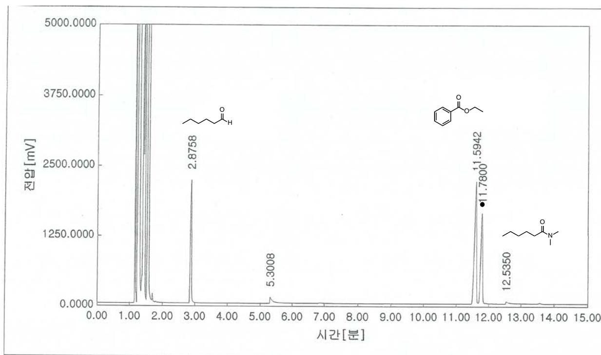
**Figure S30:** GC chromatogram of entry 11 in Table 2 and (●) represent internal standard.
