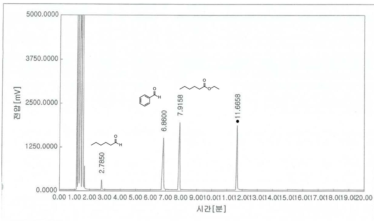
**Figure S41:** GC chromatogram of entry 9 in Table 3 and (●) represent internal standard.
