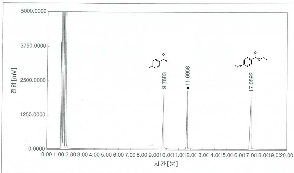
**Figure S39:** GC chromatogram of entry 7 in Table 3 and (●) represent internal standard.
