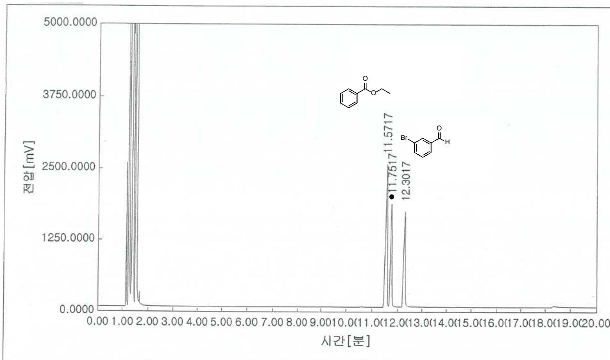
**Figure S22:** GC chromatogram of entry 3 in Table 2 and (●) represent internal standard.
