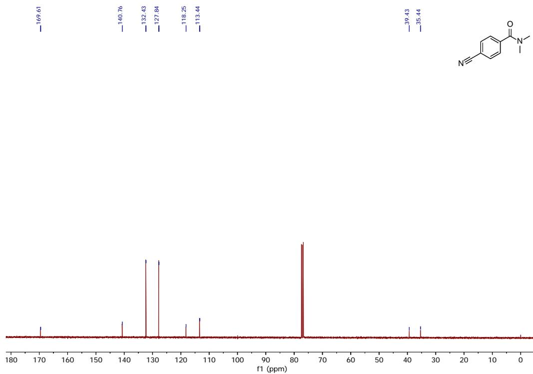
**Figure S2:** <sup>13</sup>C NMR of N,N-dimethyl-4-cyanobenzamide (Entry 5 in Table 2)
