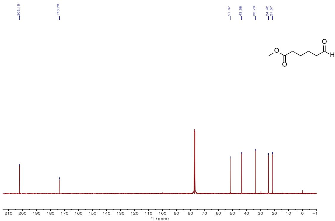
**Figure S19:**  $^{13}\text{C}$  NMR of Methyl 6-oxohexanoate (**2b**)
