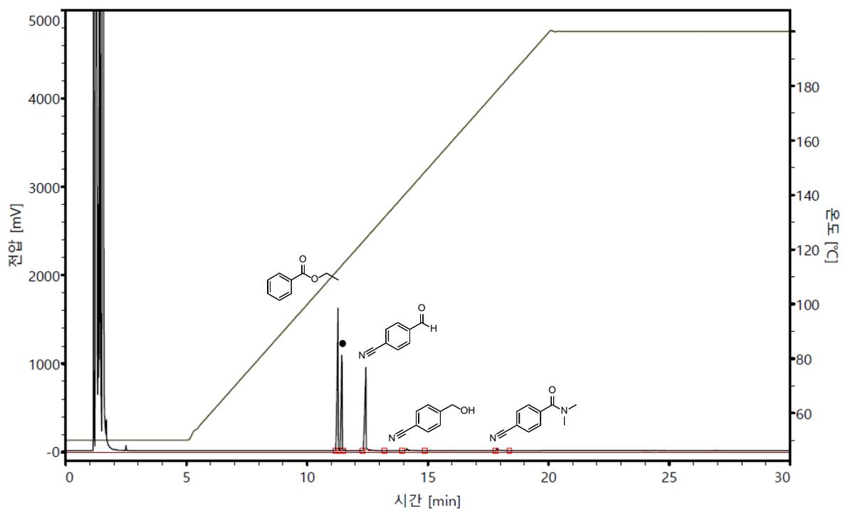
**Figure S24:** GC chromatogram of entry 5 in Table 2 and (●) represent internal standard.
