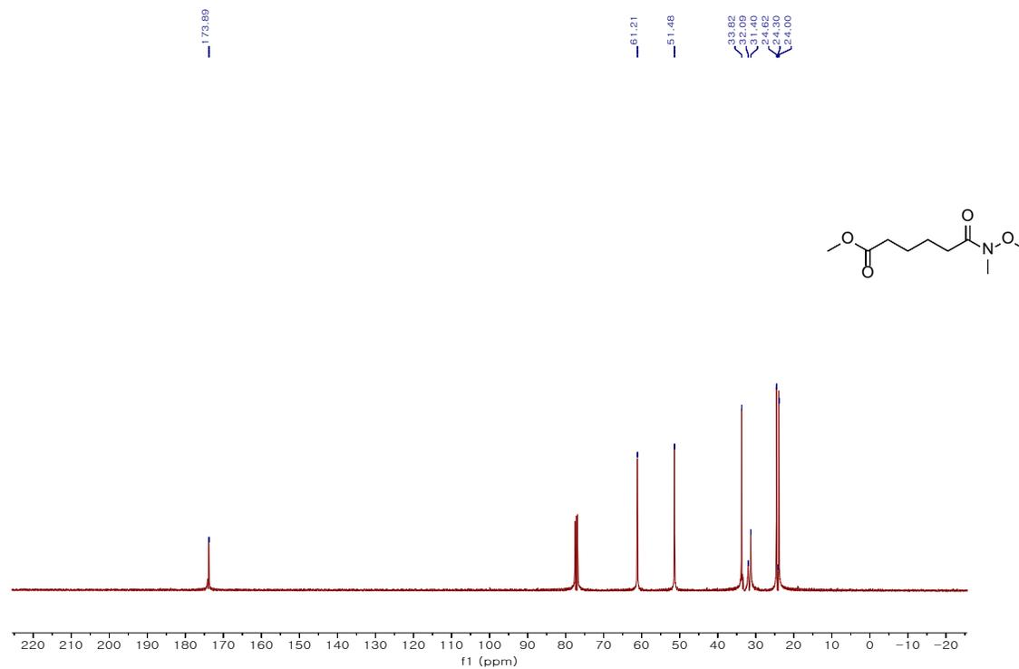
**Figure S12:** <sup>13</sup>C NMR of Methyl 6-(methoxy(methyl)amino)-6-oxohexanoate (**1d**)
