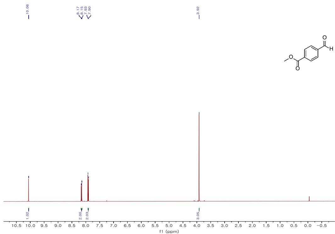
**Figure S16:**  $^1\text{H}$  NMR of Methyl 4-formylbenzoate (**2a**)
