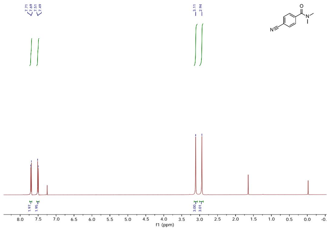
**Figure S1:** <sup>1</sup>H NMR of N,N-dimethyl-4-cyanobenzamide (Entry 5 in Table 2)
