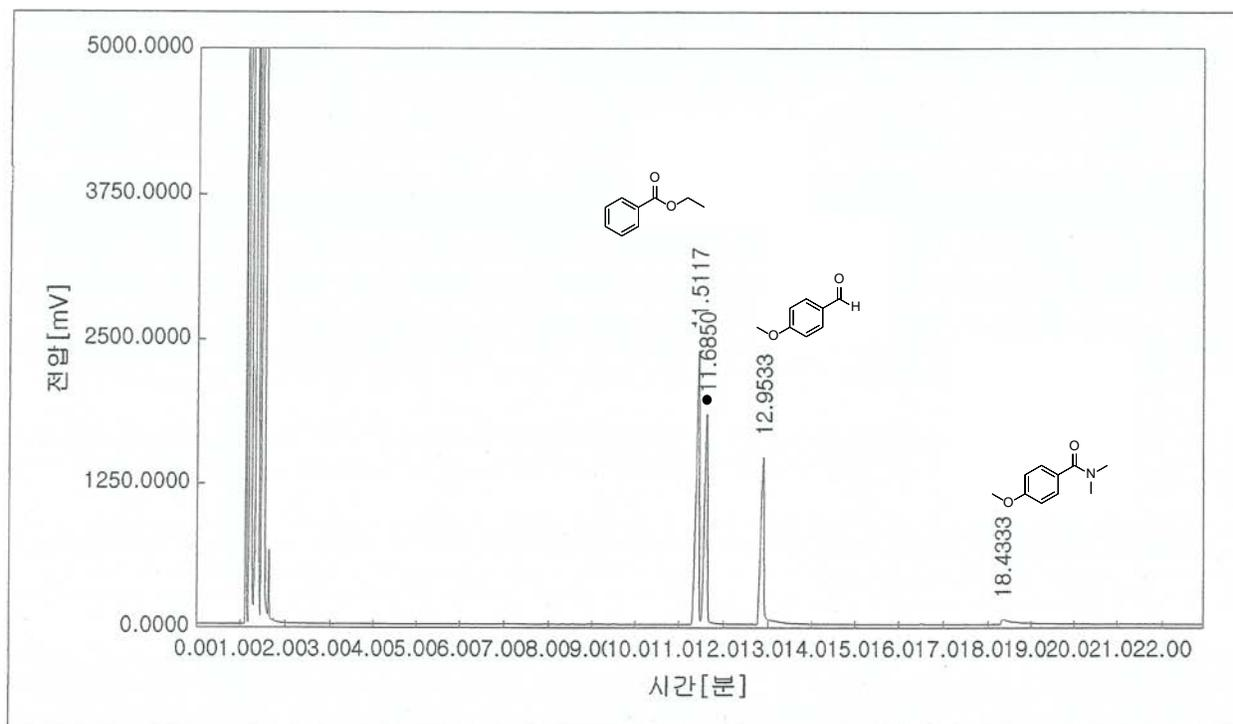
**Figure S27:** GC chromatogram of entry 8 in Table 2 and (●) represent internal standard.
