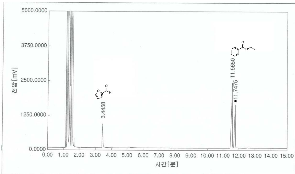
**Figure S29:** GC chromatogram of entry 10 in Table 2 and (●) represent internal standard.
