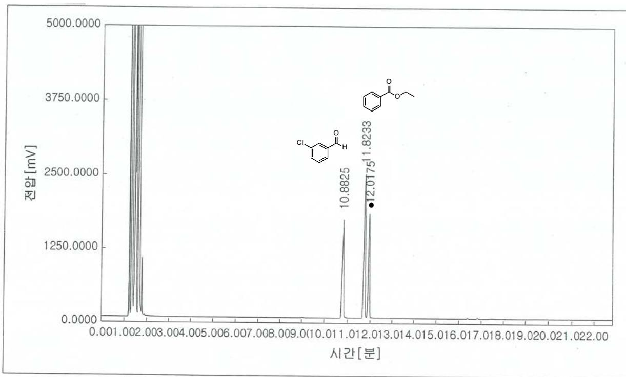
**Figure S21:** GC chromatogram of entry 2 in Table 2 and (●) represent internal standard.
