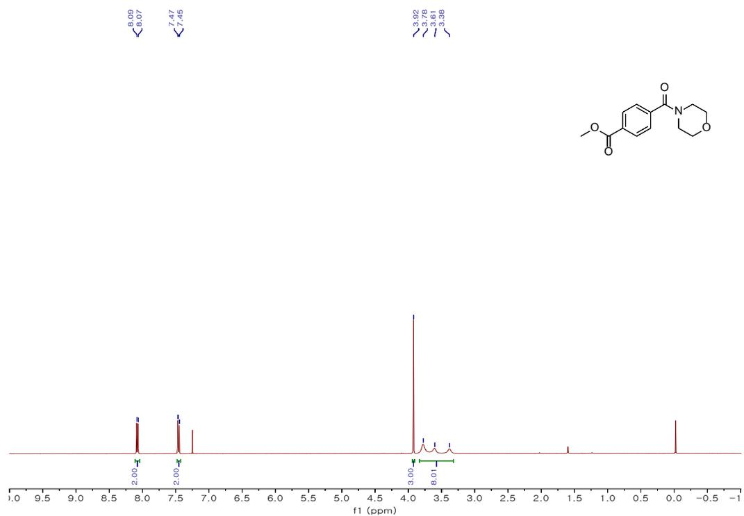
**Figure S7:** <sup>1</sup>H NMR of Methyl 4-(morpholine-4-carbonyl)benzoate (**1b**)
