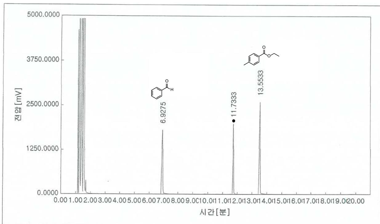
**Figure S48:** GC chromatogram of entry 4 in Table 4 and (●) represent internal standard.
