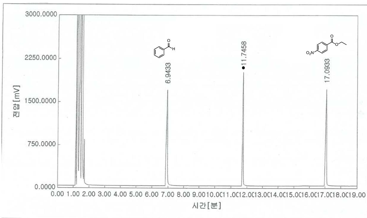
**Figure S37:** GC chromatogram of entry 5 in Table 3 and (●) represent internal standard.
