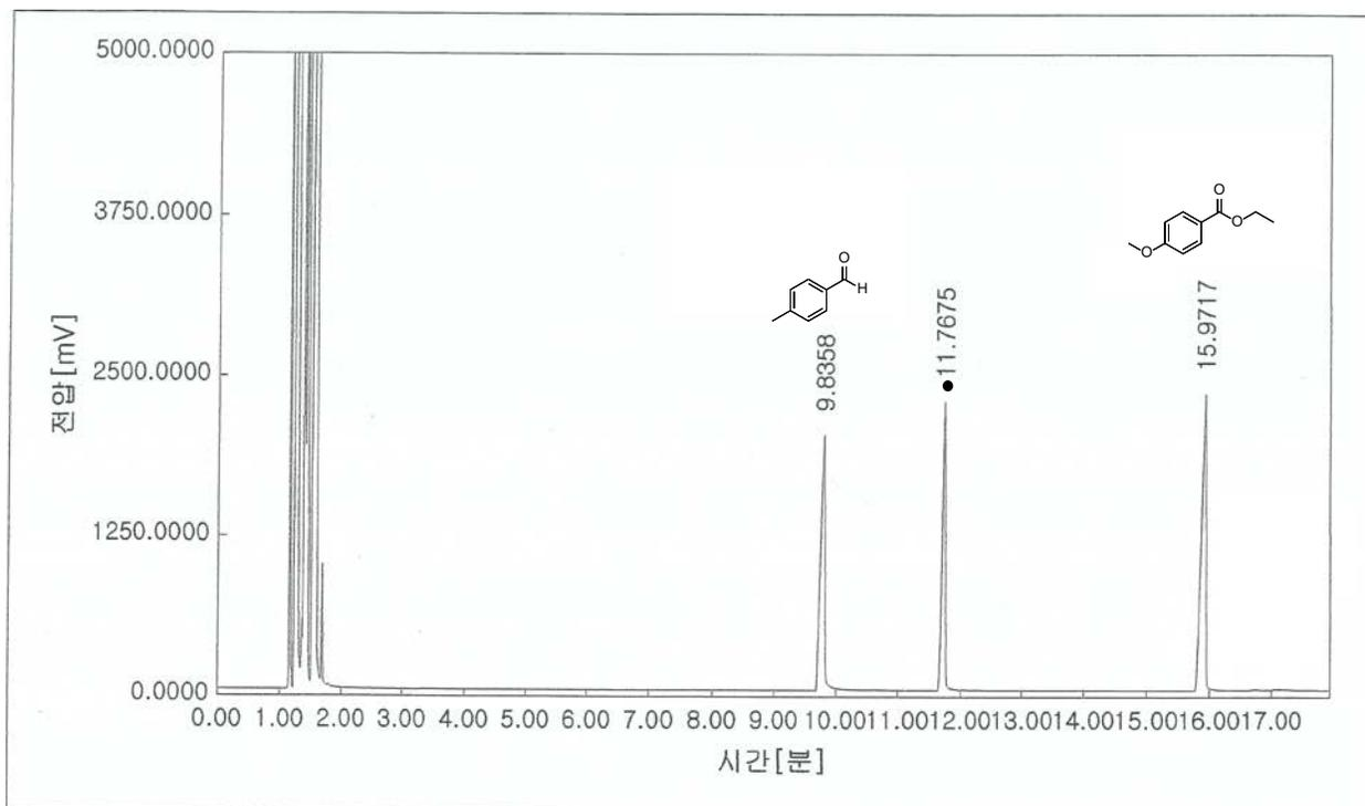
**Figure S35:** GC chromatogram of entry 3 in Table 3 and (●) represent internal standard.
