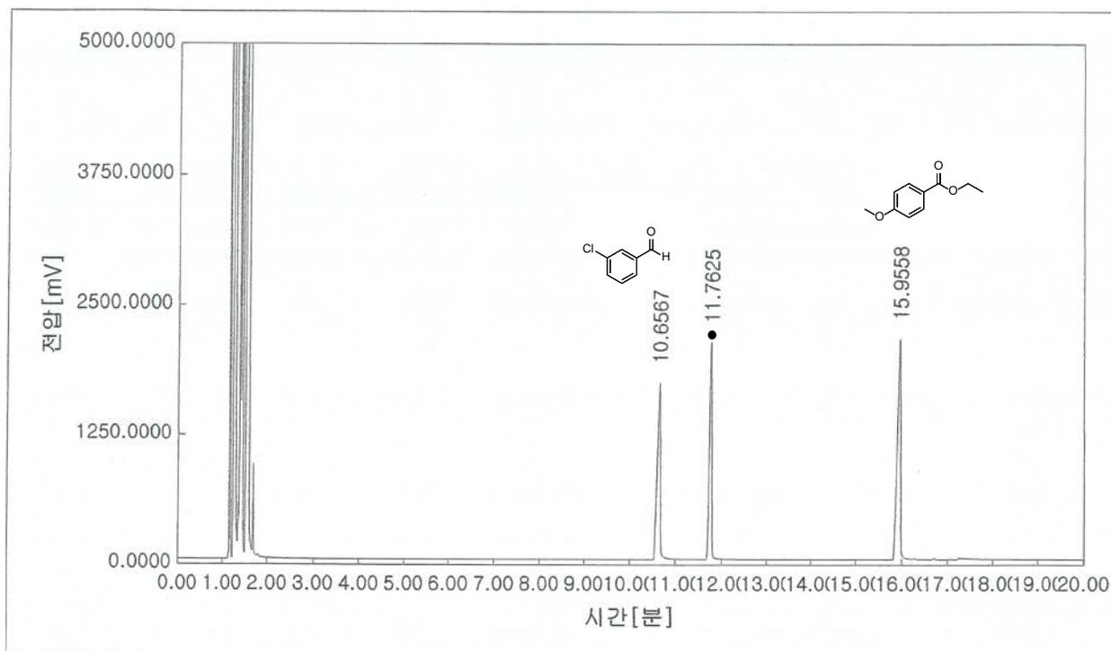
**Figure S34:** GC chromatogram of entry 2 in Table 3 and (●) represent internal standard.
