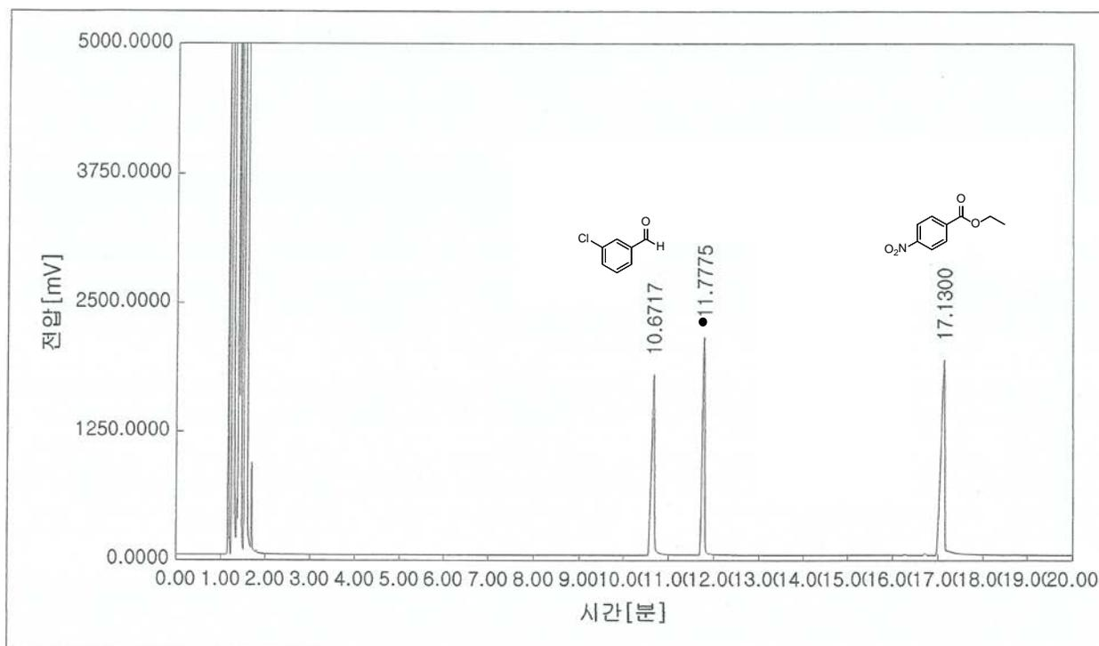
**Figure S38:** GC chromatogram of entry 6 in Table 3 and (●) represent internal standard.
