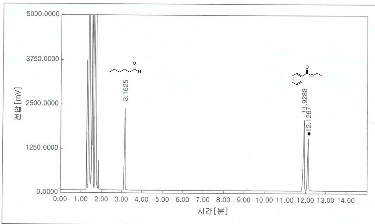
Figure S46: GC chromatogram of entry 2 in Table 4 and (●) represent internal standard.
