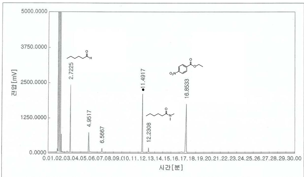
**Figure S40:** GC chromatogram of entry 8 in Table 3 and (●) represent internal standard.
