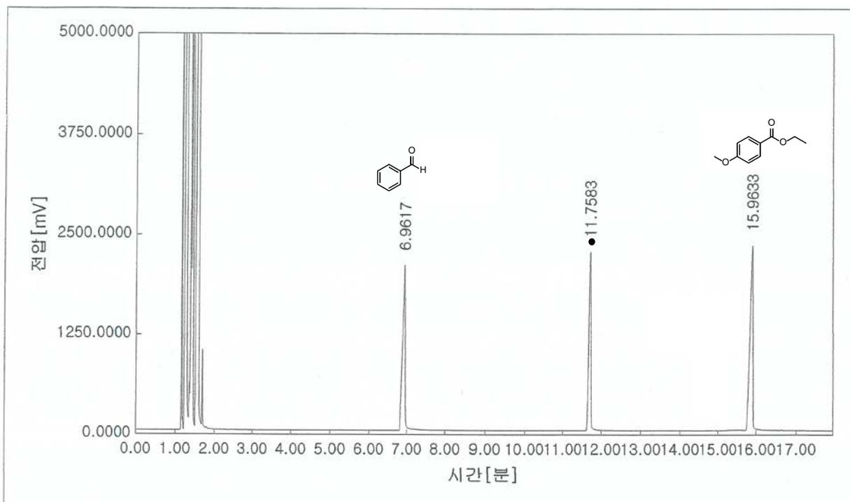
**Figure S33:** GC chromatogram of entry 1 in Table 3 and (●) represent internal standard.
