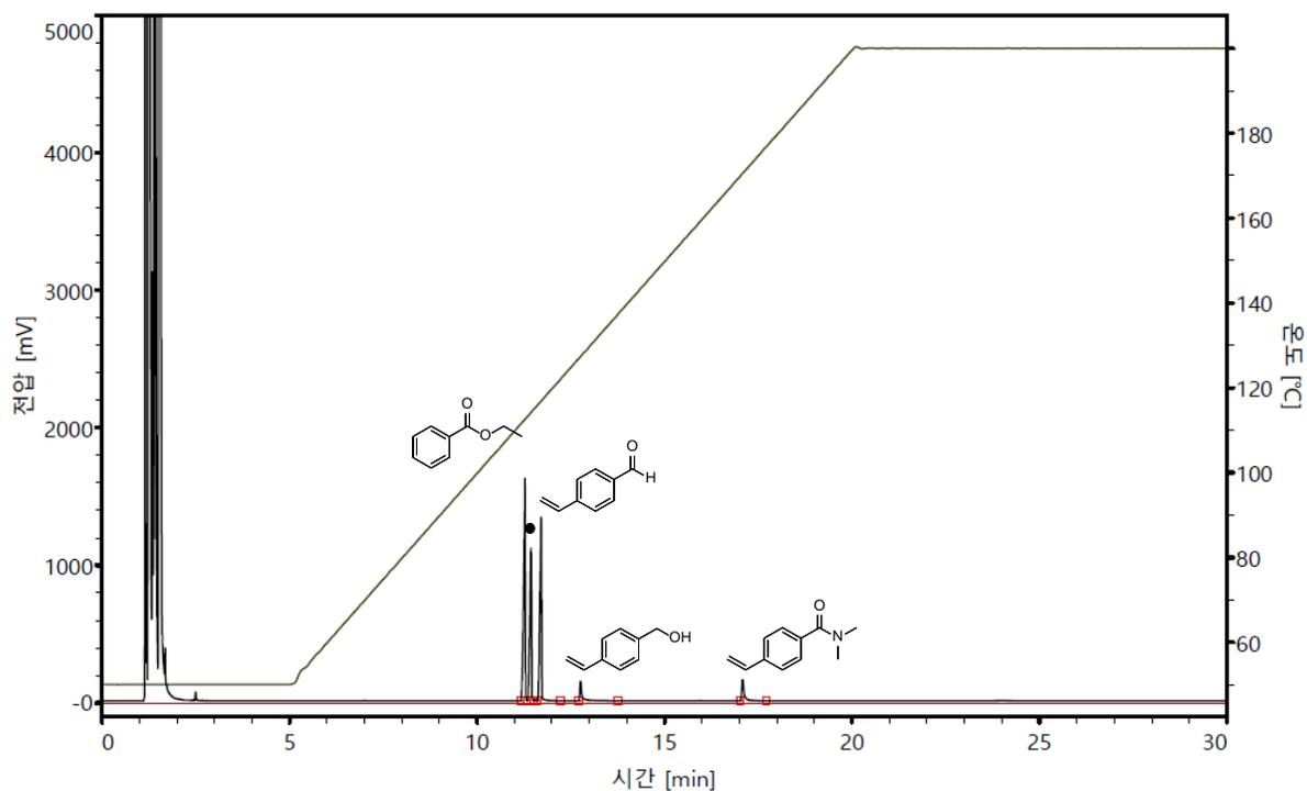
**Figure S25:** GC chromatogram of entry 6 in Table 2 and (●) represent internal standard.
