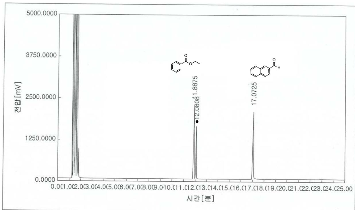
**Figure S28:** GC chromatogram of entry 9 in Table 2 and (●) represent internal standard.
