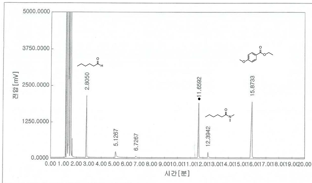
**Figure S36:** GC chromatogram of entry 4 in Table 3 and (●) represent internal standard.
