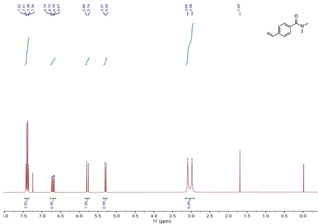
**Figure S3:**  $^1\text{H}$  NMR of N,N-dimethyl-4-vinylbenzamide (Entry 6 in Table 2)
