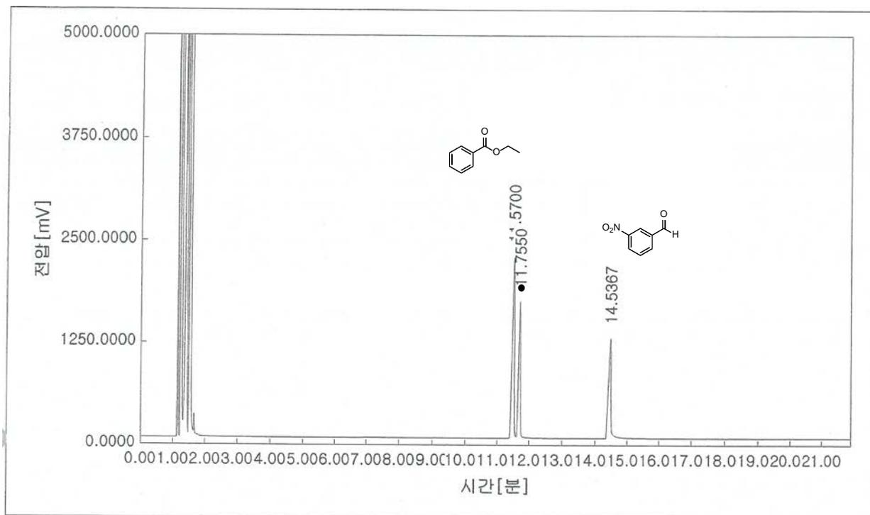
**Figure S23:** GC chromatogram of entry 4 in Table 2 and (●) represent internal standard.
