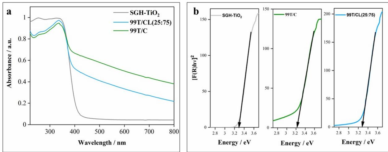
**Fig. S6 a)** UV-Visible DRS absorption spectra of SGH-TiO<sub>2</sub>, 99T/CL (25:75) and 99T/C.
