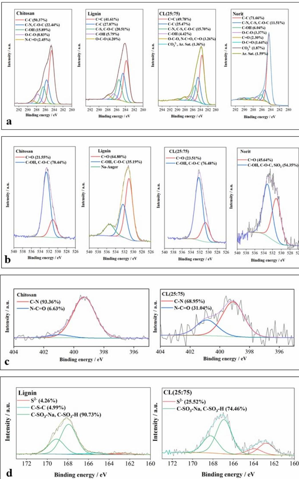
**Fig. S5 XPS spectra of chitosan, lignin, CL(25:75) and Norit a) C 1s, b) O 1s c) N 1s d) S2p**
