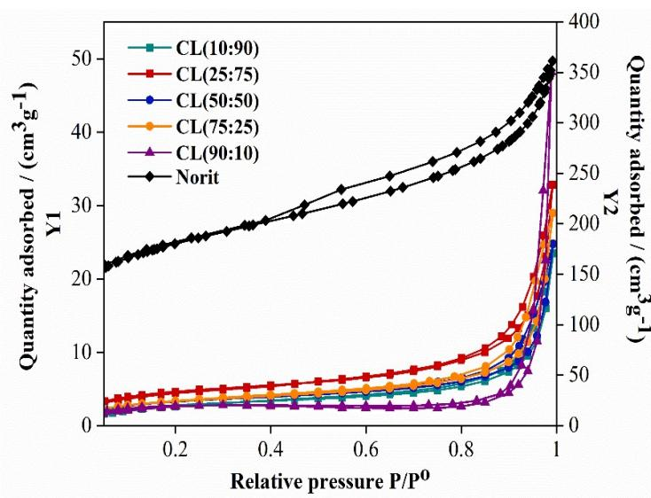
**Fig. S2** Nitrogen adsorption-desorption isotherms of CL composites and Norit (Quantity adsorbed by CL composites displayed on Y1 axis and quantity adsorbed by Norit displayed on Y2 axis).
