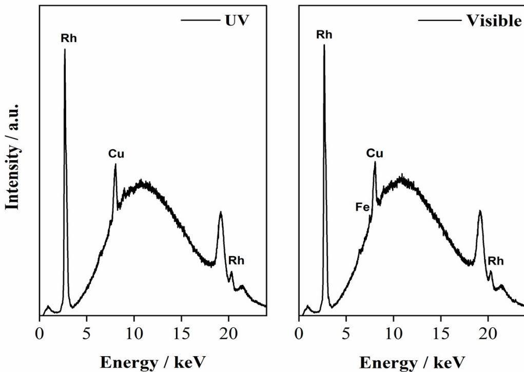
**Fig. S8 XRF analysis of BnOH solution catalyzed over 75T/CL(25:75) nanocomposite.**
