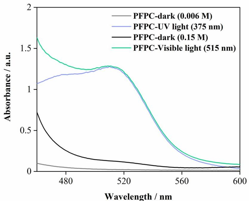
**Fig. S10** UV-Visible absorption spectrum of potassium–ferrioxalate phenanthroline complex (PFPC).
