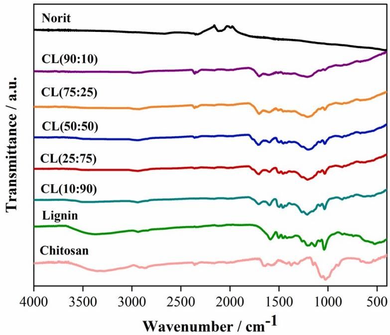
**Fig. S4 FTIR spectra of chitosan, lignin, Norit and CL composites.**
