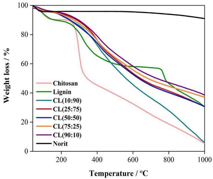
**Fig. S3 Thermogravimetric analysis (TGA) curves of CL composites and Norit under N<sub>2</sub> atmosphere.**
