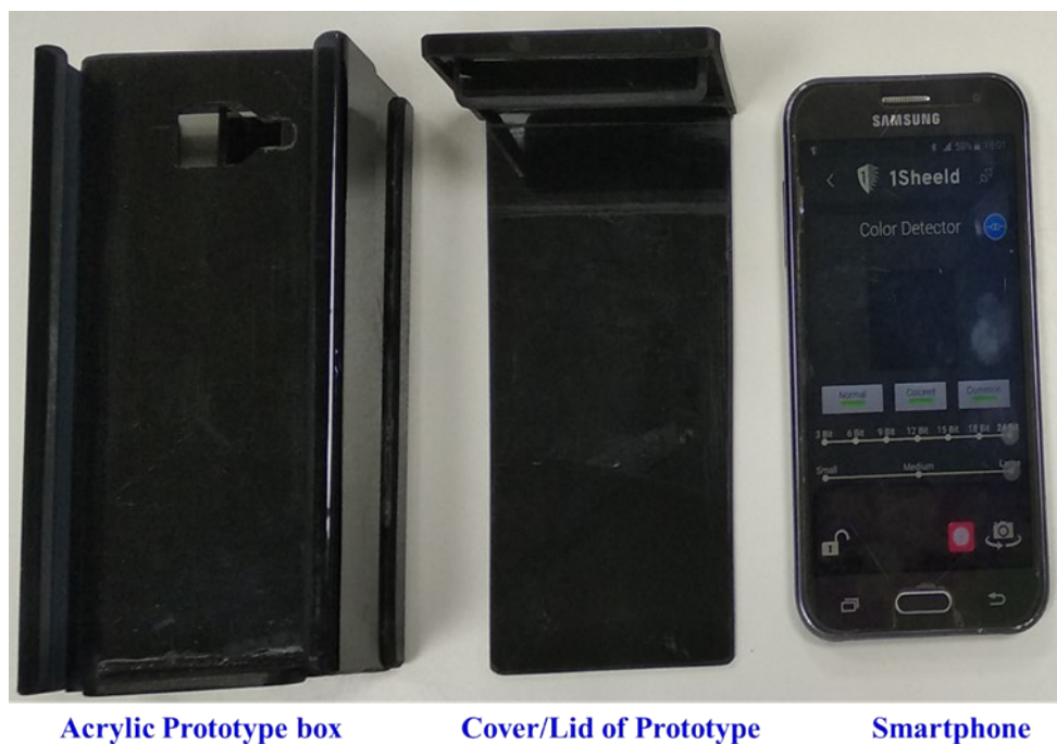
Fig. S25 Sensory prototype displaying the Smartphone, black acrylic prototype box along with its lid separately.
