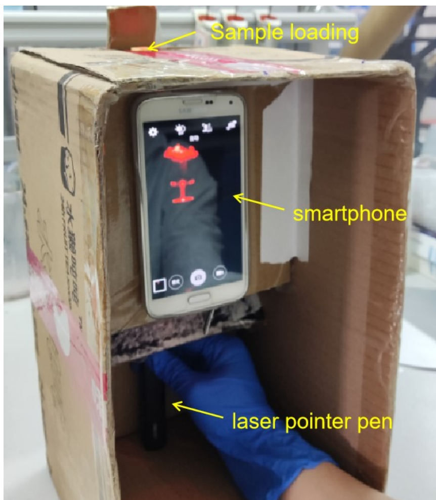
3 Fig. S1 The photograph of the home-made fully-enclosed device providing stable 4 “black” environmental condition.
