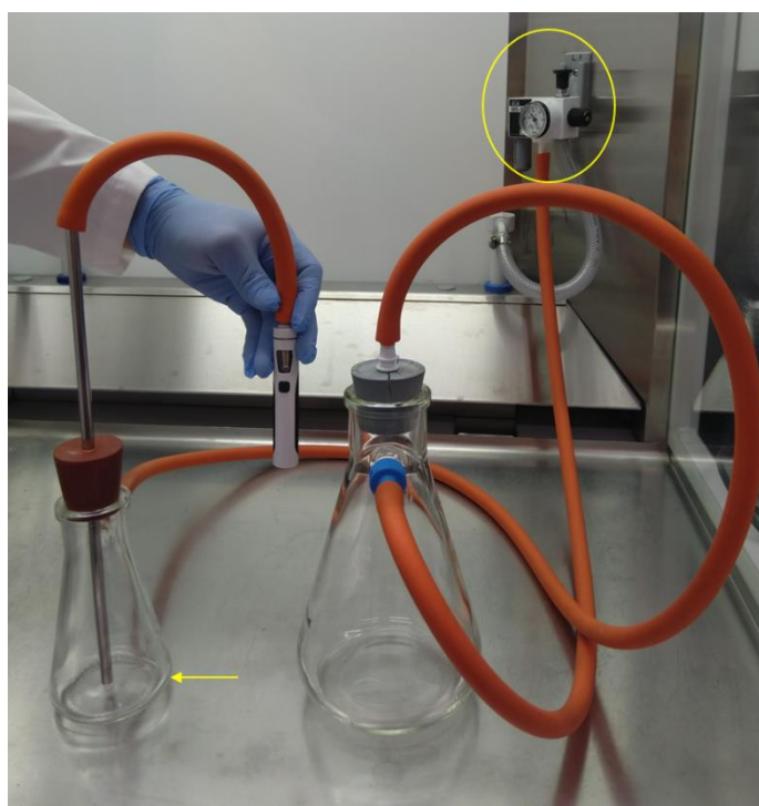
Figure S1: The vacuum system for preparation of electronic cigarette aerosol solutions. The sample collection flask is indicated by an arrow and the vacuum measurement instrumentation by a circle.
