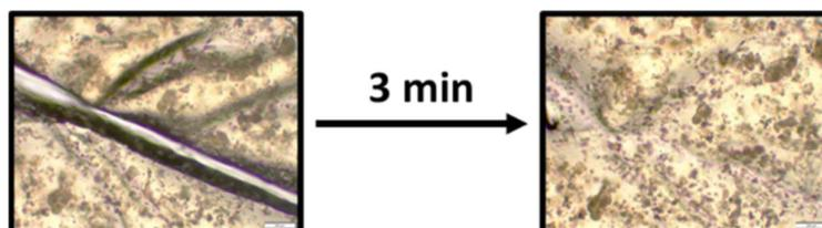
**Fig. S8.** Self-healing pathway with corresponding optical microscopic images depicting the autonomous self-healing of the film of decrosslinked polymer **TP4** to show complete autonomous healing within 3 min.
