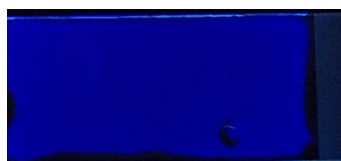
Figure S7. Photograph of epoxy-EAn layer under 365 nm UV light after overexposure for information erasure.
