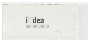
Figure S6. Photograph of epoxy-EAn layer under natural light after information input.
