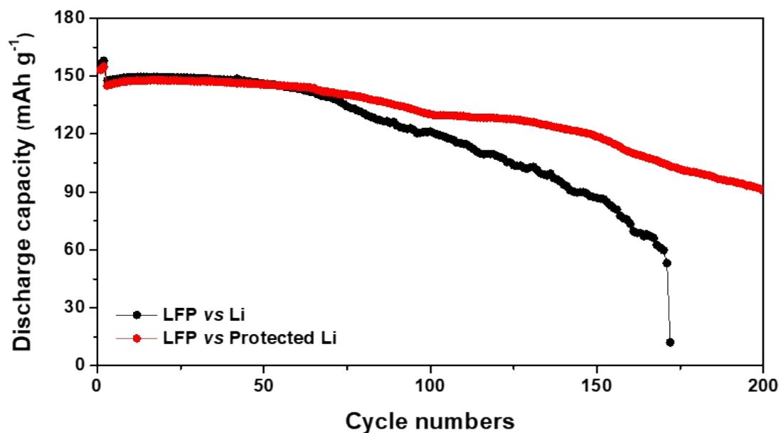
Fig. S8. Discharge capacity curves of the LFP||bare Li and LFP||protected Li full cells at the current density of 0.5C.
