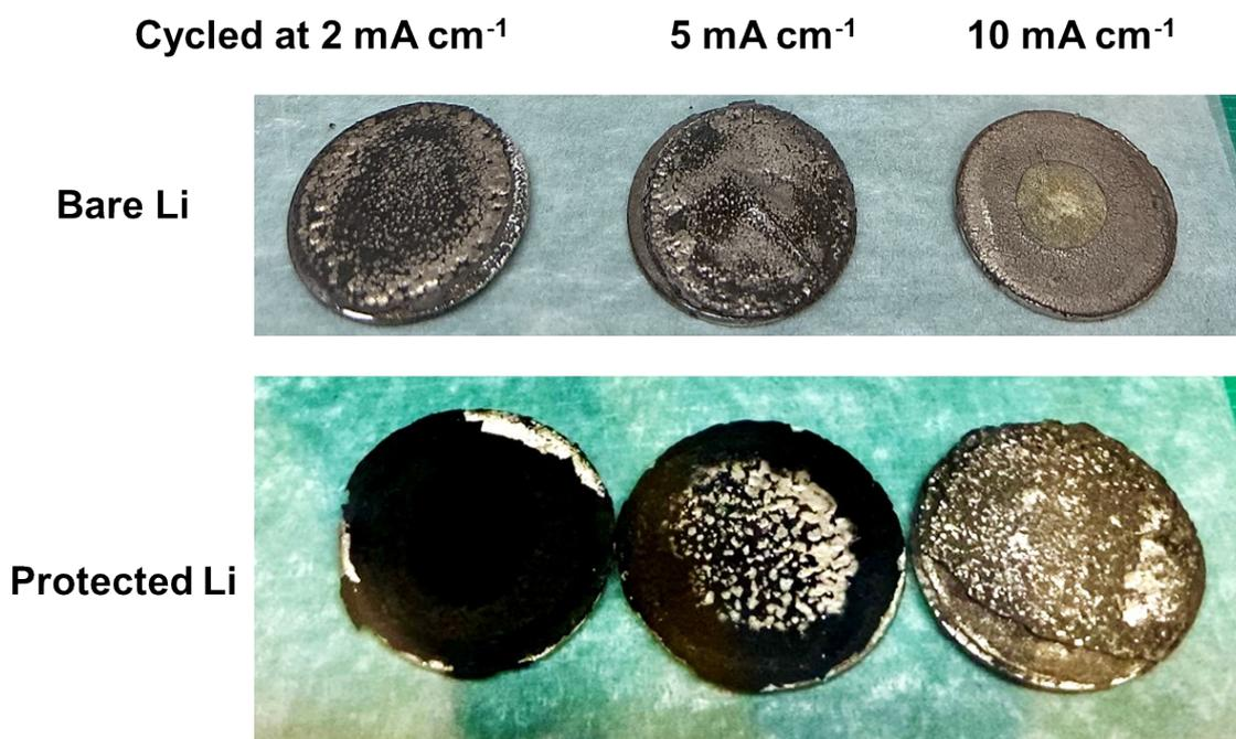
**Fig. S5.** Photographs of the bare Li and protected Li surfaces after symmetric cell cycling tests at various current densities.
