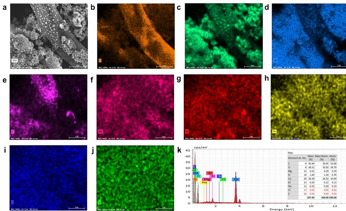
**Fig. S3.** (a) FE-SEM image of carbonized Post-it note and its energy dispersive X-ray spectrometry (EDS): elemental mapping images of (b) C, (c) O, (d) Ca, (e) Si (f) Mg, (g) Al, (h) Na, (i) S, (j) Cl, and (k) EDS spectrum (weight and atom % inset).
