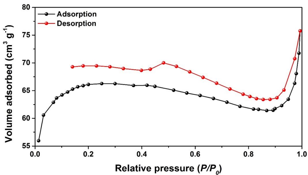
Fig. S4. Nitrogen adsorption/desorption isotherms at 77 K of the carbonized Post-it note.
