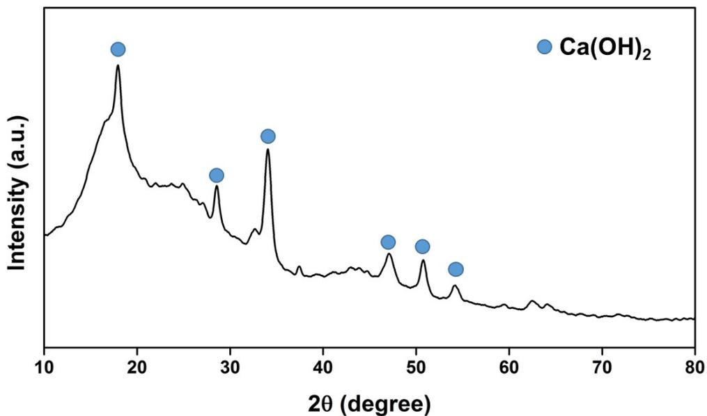
Fig. S3. X-ray diffractogram curve of the as-received Post-it note.
