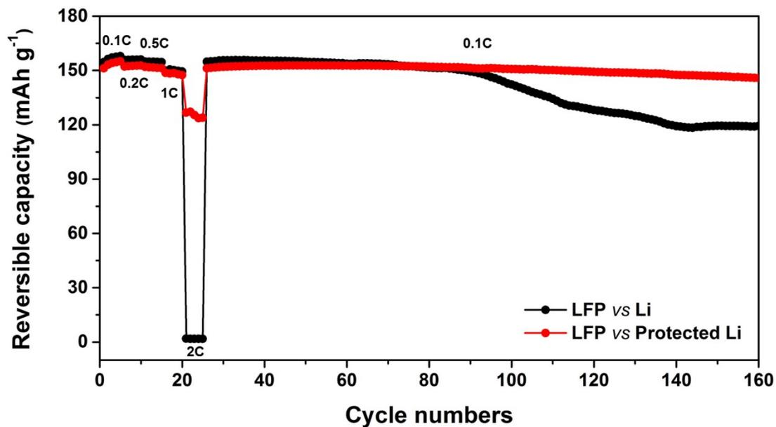
Fig. S7. Rate capabilities at charging current densities of 0.1C, 0.2C, 0.5C, 1C, 2C, and 0.1C.
