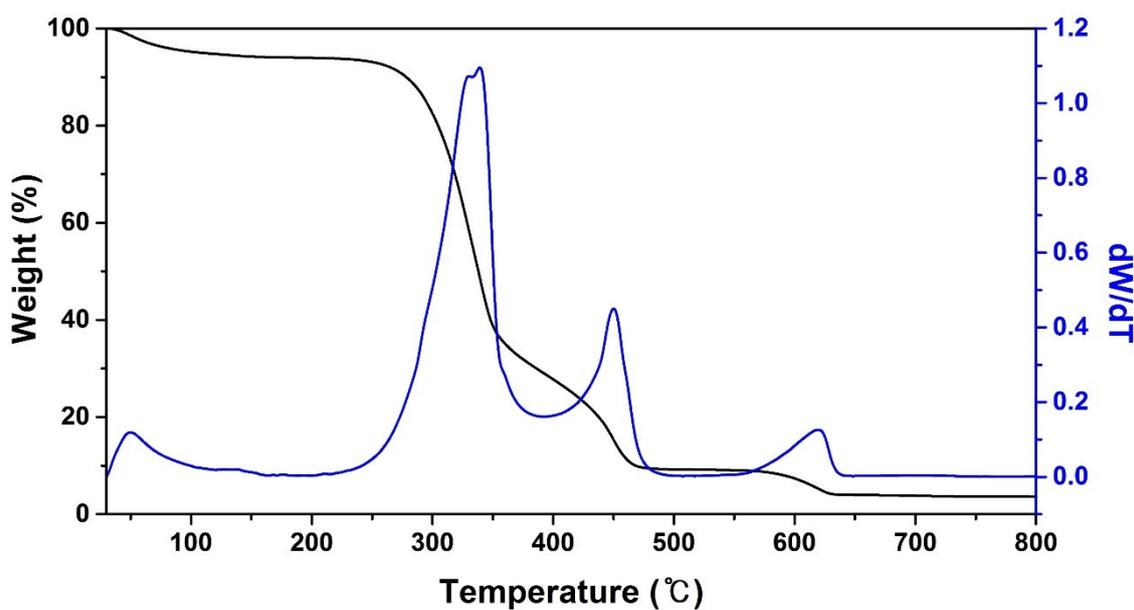
**Fig. S1.** Thermogravimetric analysis of the Post-it note under air atmosphere and its differential weight-change curve.
