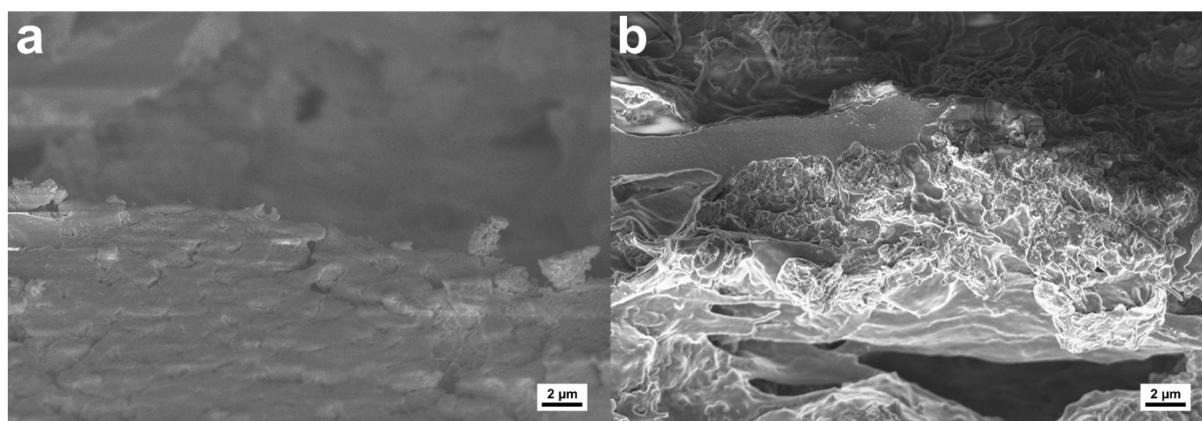
**Fig. S6** Scanning electron microscope images of (a) the protected Li surface and (b) cross-section of the protection layer after 5000<sup>th</sup> cycles. The current density was  $10 \text{ mA cm}^{-1}$ , the areal capacity was  $1 \text{ mAh cm}^{-1}$ .
