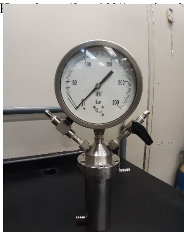
Figure S2. Stainless steel reactor.
