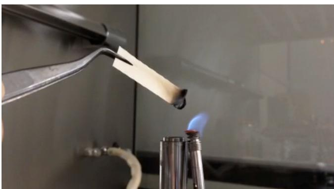
After ignition, a char layer was formed promptly, the test piece hardly burned
