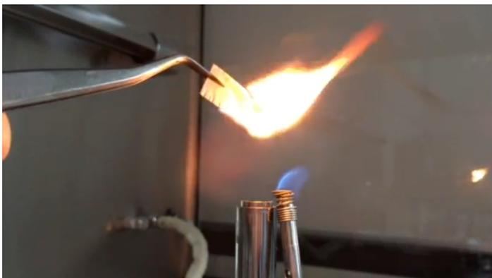
After ignition, the flame burned throughout and the specimen burned mostly.
