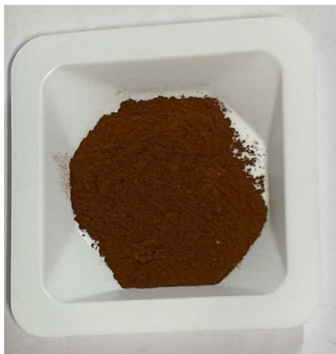
Figure S15: Fe-rich precipitate
