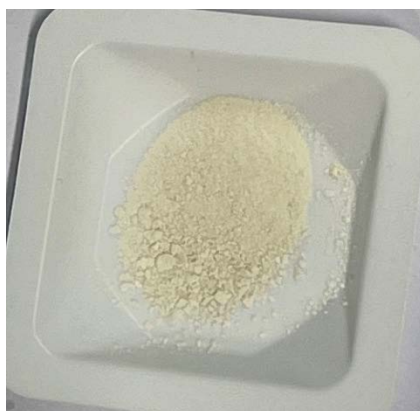
Figure S16: Zn-rich precipitate
