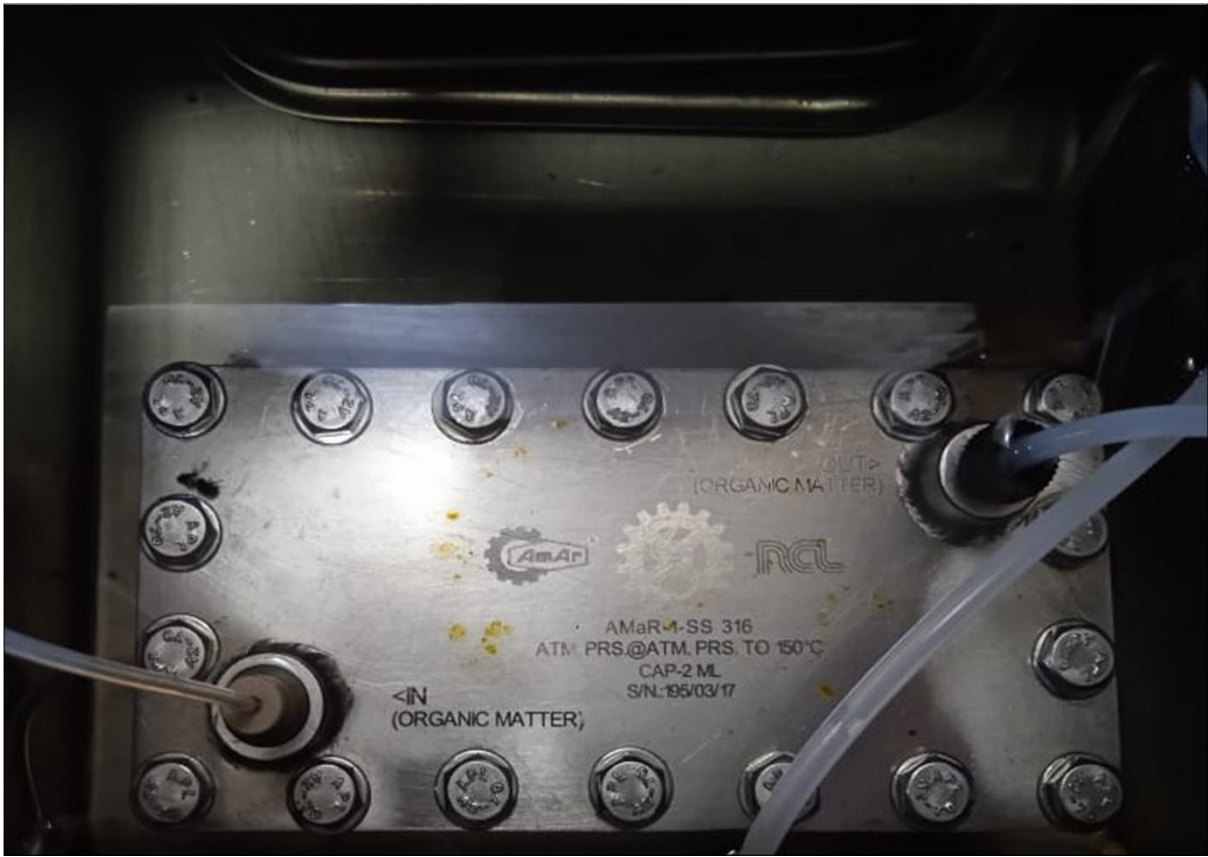
Figure S2. Dual function microreactor deep in the oil bath.
