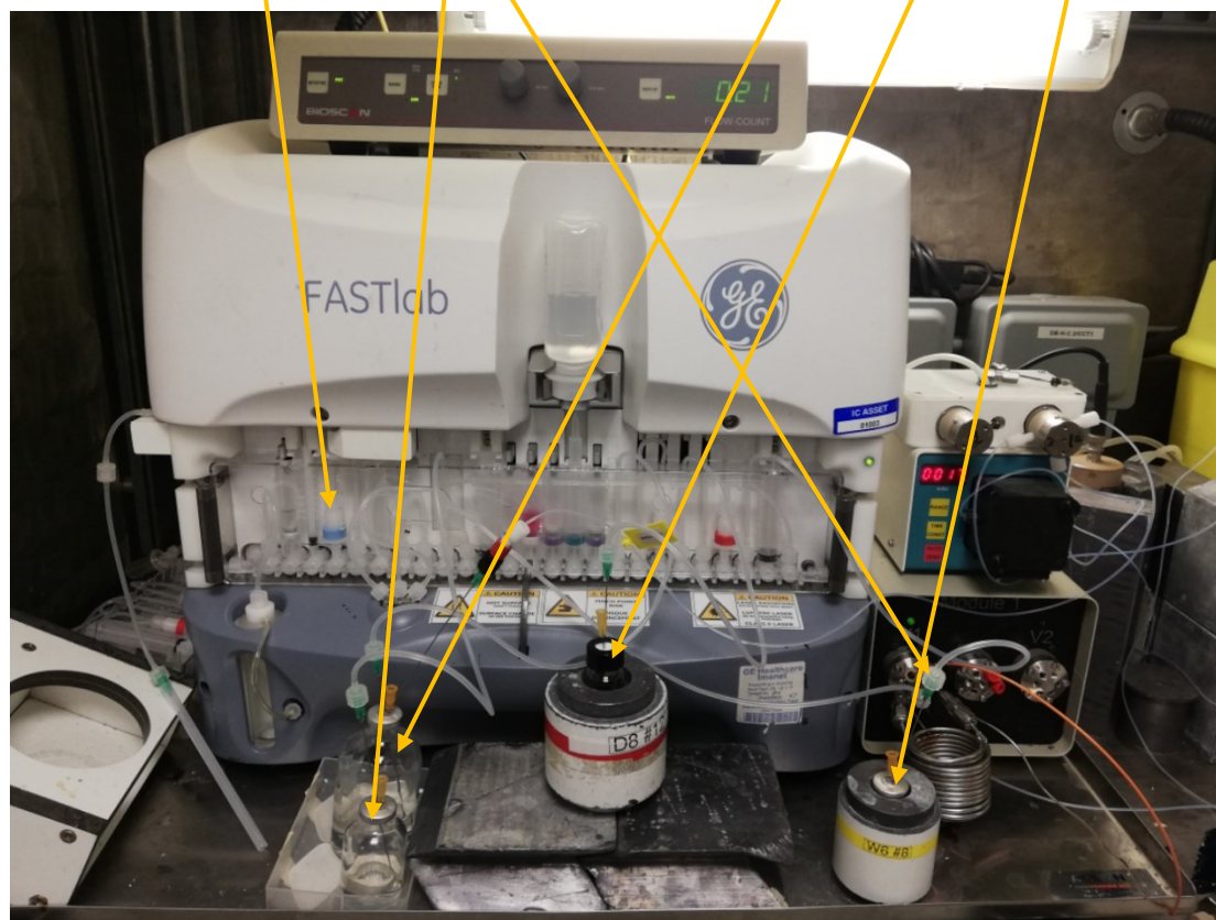
Figure 14. Schematic and photograph of the FASTLab™ cassette setup for the automated radiosynthesis of [ ^{18}\text{F} ]TTCO-IL2.
