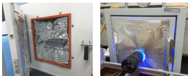
Figure S3. Kessil Lamp Photoreactor. Left to right. (A) Interior set-up of vacuum oven. (B) Irradiation with Kessil lamp.
