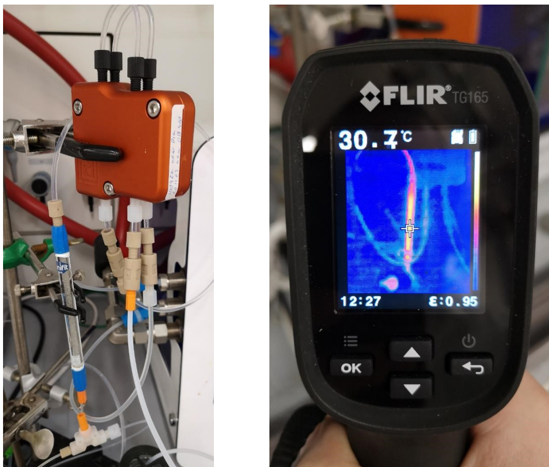
Fig. S4. Left: photograph of the packed Omnifit column used to form the N -chloroamine, followed by the membrane separator. Right: thermal imaging camera (FLIR TG165) used to roughly assess the temperature within the Omnifit column, which shows a mild exotherm (~30 °C).
