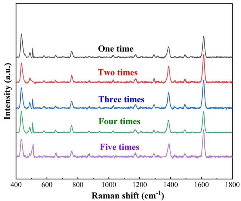
**Fig. S2** Raman spectra of the MB molecules detected using the SERS substrates after various recycle times.
