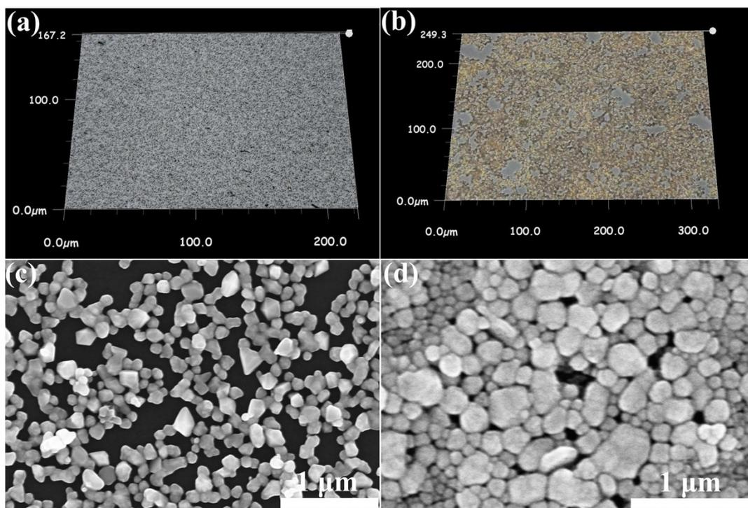
**Fig. S3** (a-b) SDFM images of the AuNPs-based SERS substrates dried for 2h: (a) at room temperature, (b) at 80 °C; (c-d) The corresponding SEM images of the SERS substrates dried for 2h: (c) at room temperature, (d) at 80 °C.
