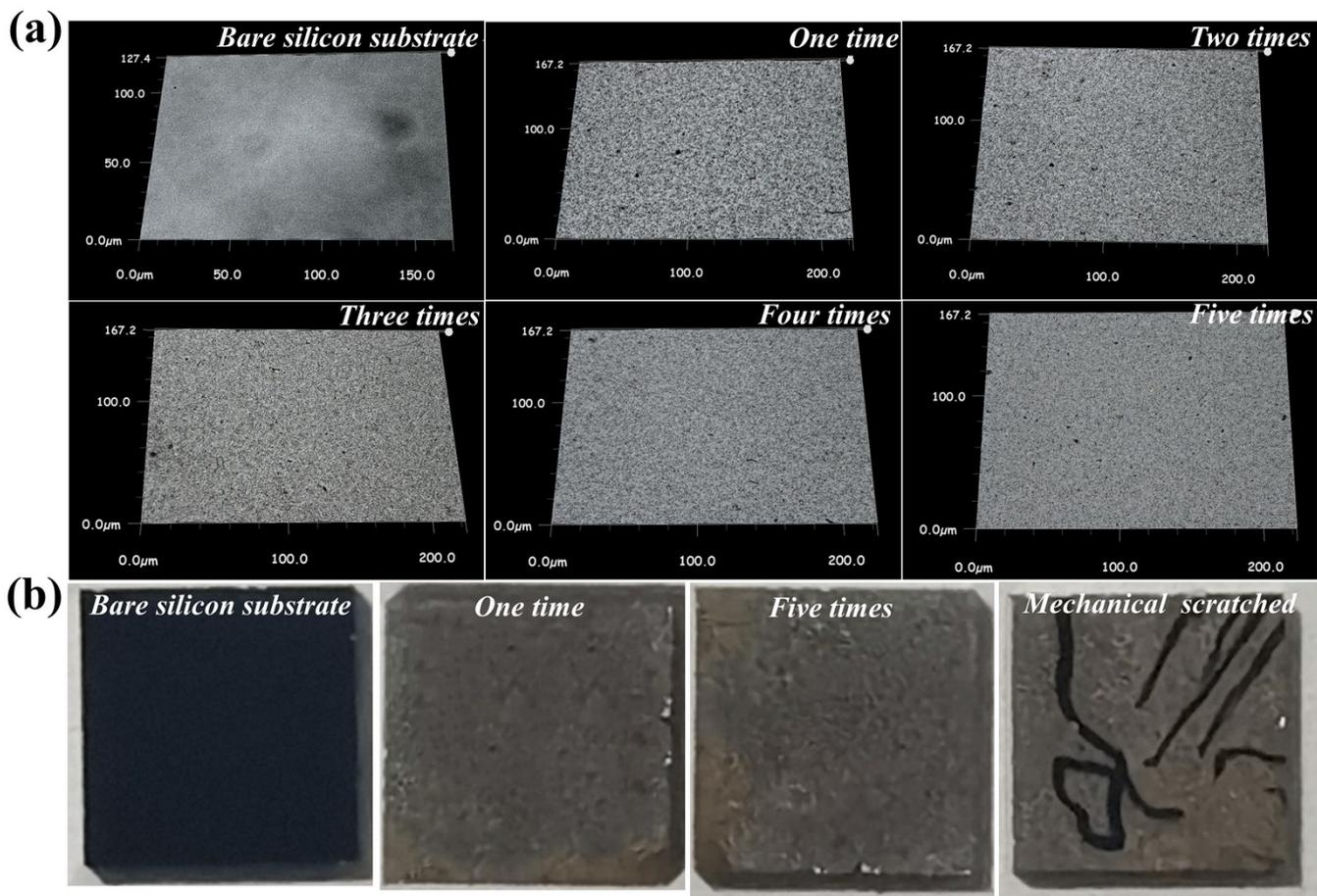
**Fig. S1** (a) Representative SDFM images of the SERS substrates after different times of usage; (b) The photographs of the SERS substrates after different treatments.
