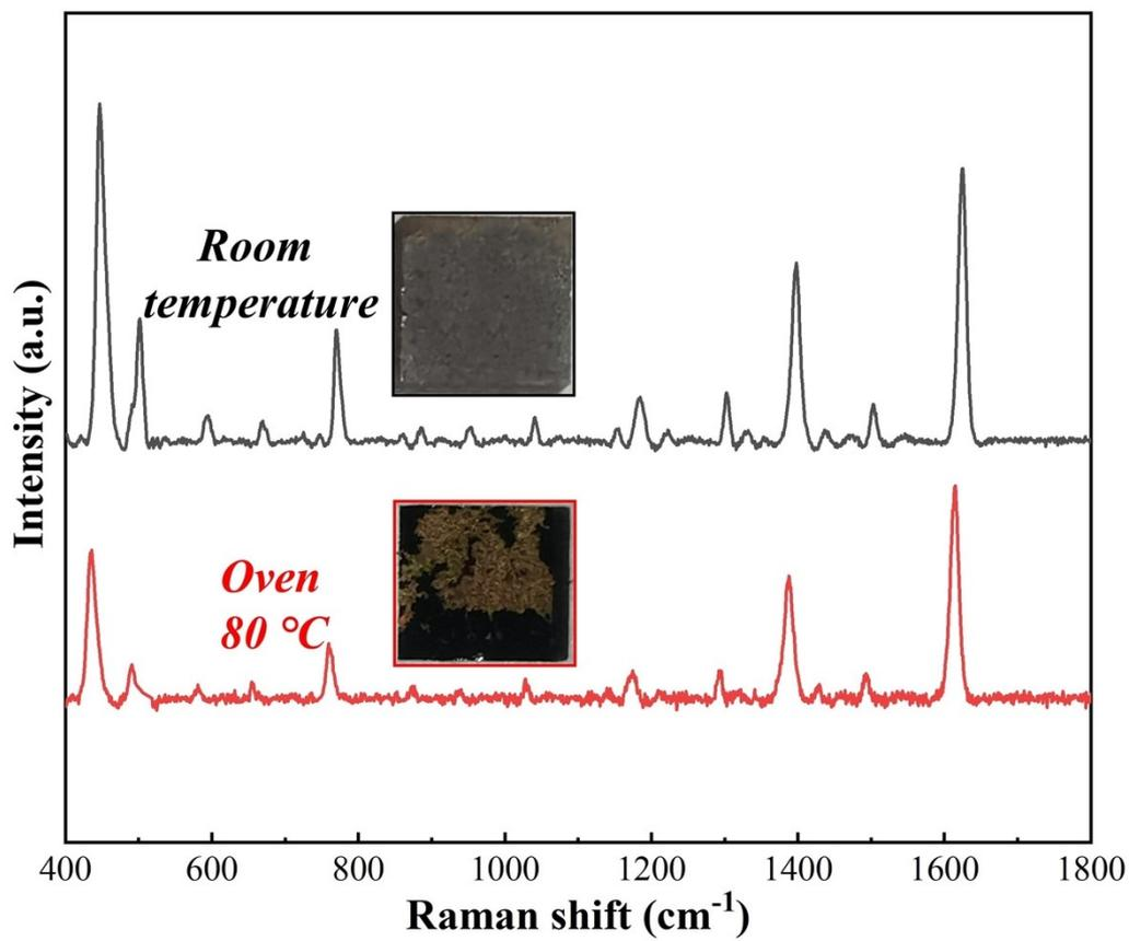
Fig. S4 SERS spectra of the MB molecules absorbed on substrates dried at room temperature as well as at 80 °C.
