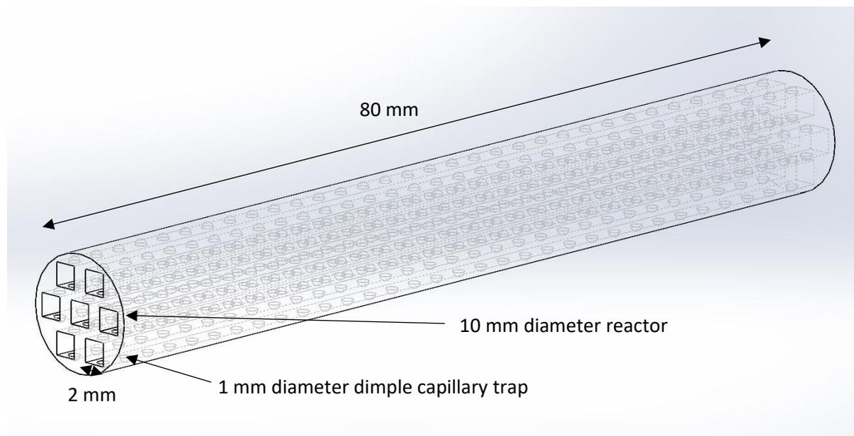
**Figure S3** Monolithic dimpled Capillary Force Trap Reactor (CFTR) (see main text for details)
