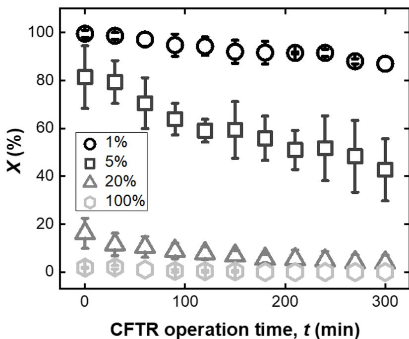
**Figure S2.** Substrate (1-hexene) conversion,  $X$  vs. CFTR operation time,  $t$ .  $C_{hex,0} = 0.08$  M (1% 1-hexene in decane),  $C_{hex,0} = 0.4$  M (5% 1-hexene in decane),  $C_{hex,0} = 1.6$  M (20% 1-hexene in decane),  $C_{hex,0} = 8.1$  M (100% 1-hexene in decane),  $C_{cat} = 2$  mM, precursor to stabilizer molar ratio:  $RhCl_3:PVP = 1:100$ ,  $Q_{org} = 20$   $\mu$ L/min,  $\tau = 50$  s:  $Q_{gas} = 0.04$  mL/min.
