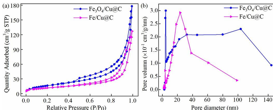
Fig. S1 (a) N<sub>2</sub> adsorption-desorption isotherms and (b) pore size distribution curves of Fe/Cu@C (Fe<sup>3+</sup> 10 wt%) and Fe<sub>3</sub>O<sub>4</sub>/Cu@C (Fe<sup>3+</sup> 10 wt%).
