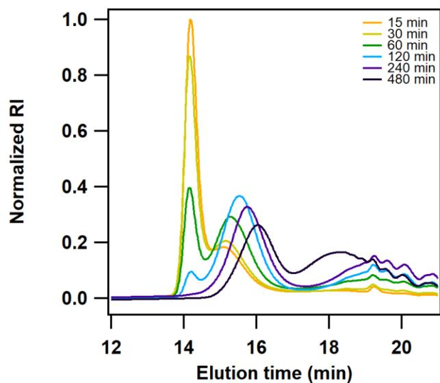
**Figure S20.** GPC traces of **P2-H** at different sonication times after 10 mM TFA treatment.
