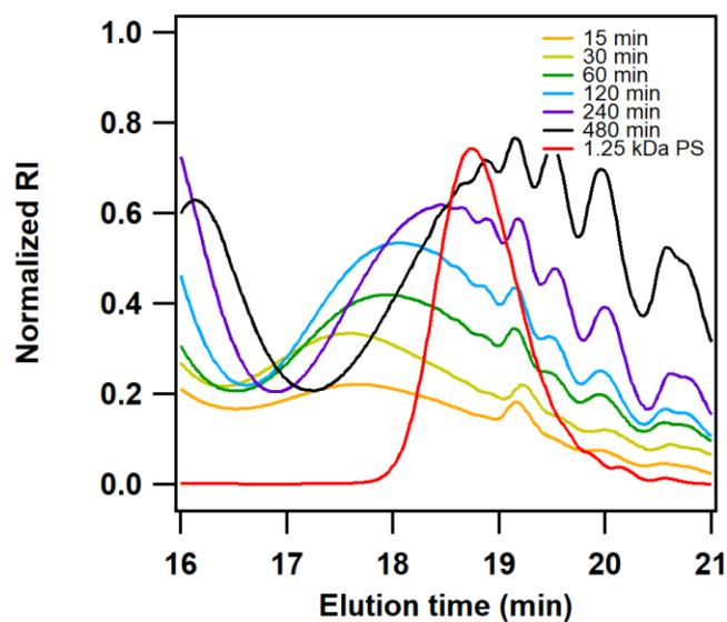
**Figure S18.** GPC traces of **P1-H** at different sonication times after 10 mM TFA treatment. The red trace is a PS standard ( $M_n = 1.25$  kDa) for comparison of MW.
