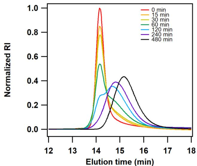
**Figure S19.** GPC traces of **P2-H** at different sonication times (sonication condition: 1 mg/mL solution in THF).
