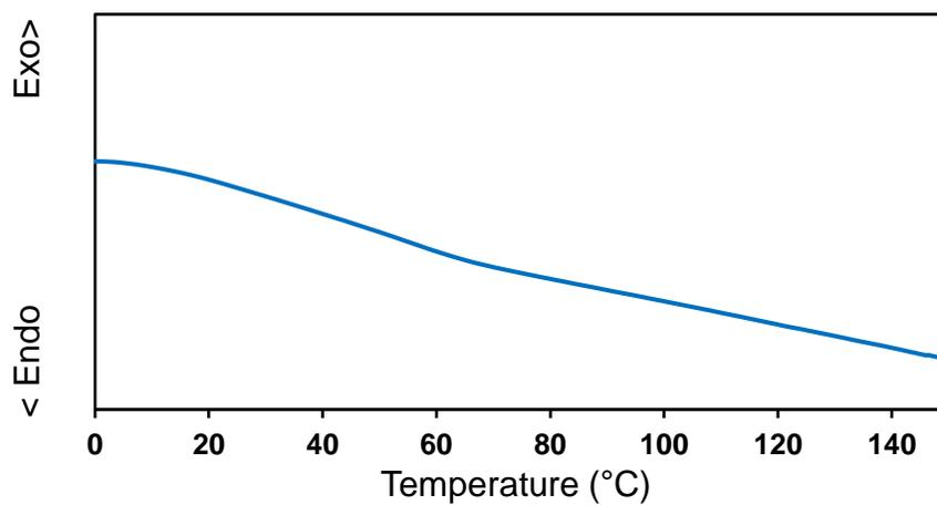
**Figure S26.** DSC curve of polymer **P3-H** indicating a T<sub>g</sub> of 56 °C.
