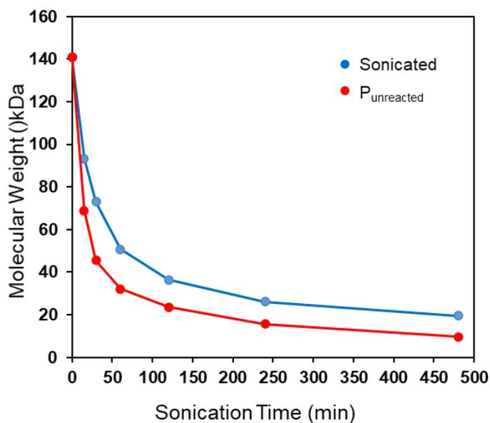
**Figure S22.**  $M_n$  of sonicated **P1-H** before acidic degradation (blue curve) and  $P_{\text{unreacted}}$  at different sonication times (red curve).  $P_{\text{unreacted}}$  refers to the unactivated polymer segments that are presumably located toward the ends of the polymer chain.
