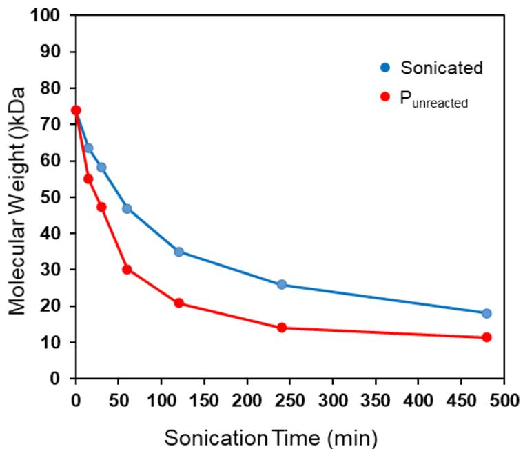
**Figure S23.**  $M_n$  of sonicated **P2-H** before acidic degradation (blue curve) and **P<sub>unreacted</sub>** at different sonication times (red curve). **P<sub>unreacted</sub>** refers to the unactivated polymer segments that are presumably located toward the ends of the polymer chain.
