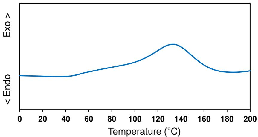
**Figure S4.** DSC curve of **P1** indicating thermal decomposition beginning at 46 °C.
