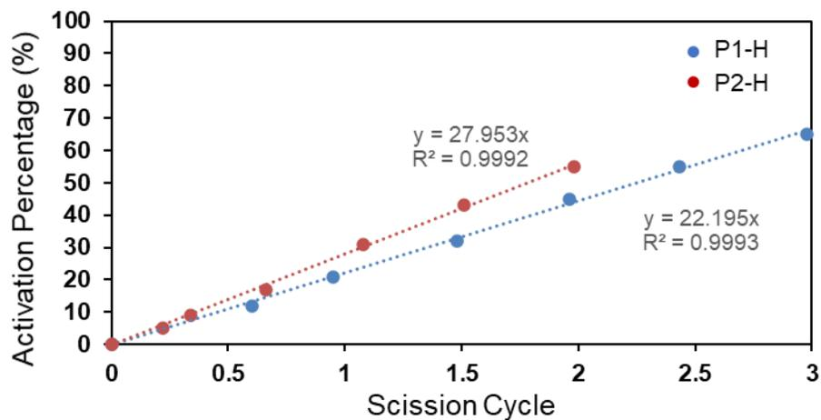
**Figure S17.** Activation percentage versus scission cycle for **P1-H** and **P2-H**. The activation percentage per scission cycle for **P1-H** and **P2-H** is 22% and 28%, respectively.
