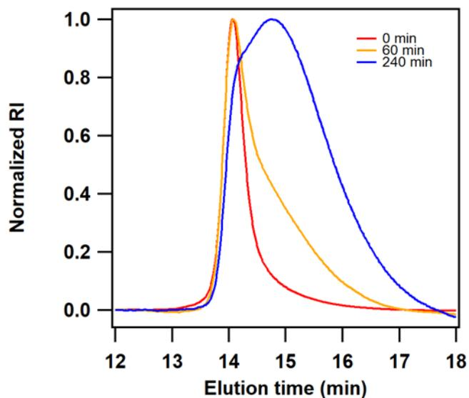
**Figure S3.** GPC traces of poly(1) showing peak broadening upon leaving quenched polymerization solution for the indicated times under ambient condition (polymerization condition:  $[M]_0 = 1$  M,  $[M]_0/[G3] = 1000$ , reaction time = 15 min, temperature = 0 °C).
