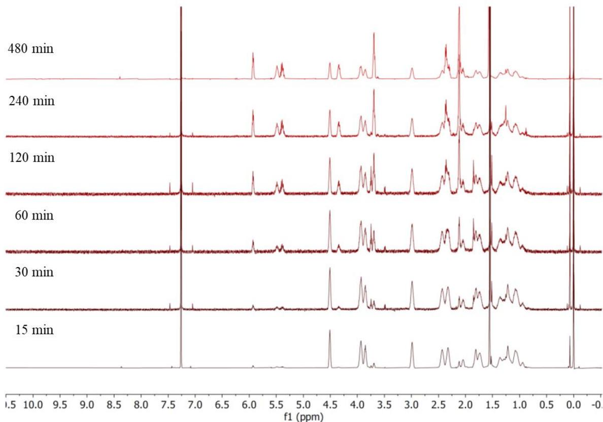
**Figure S15.**  $^1\text{H}$  NMR spectra of **P2-H** at different sonication times.
