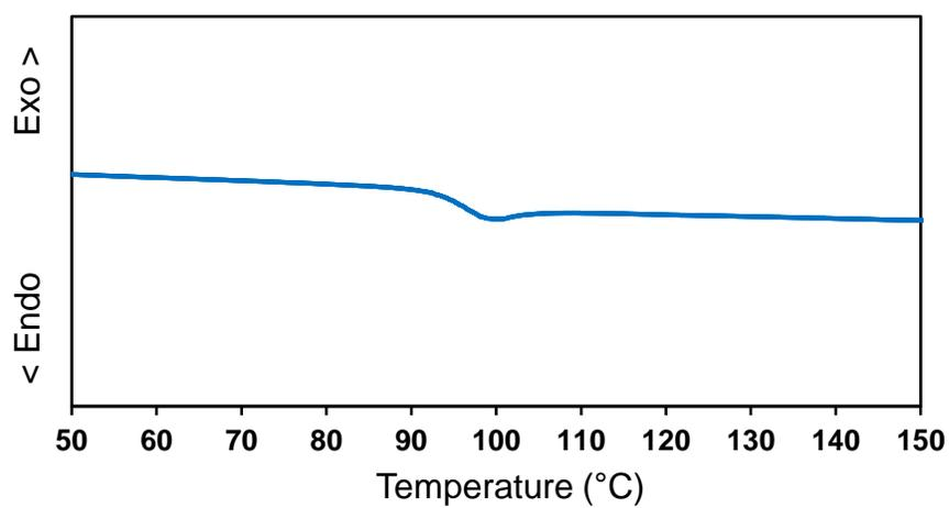
**Figure S5.** DSC curve of polymer **P1-H** indicating a  $T_g$  of 94 °C.
