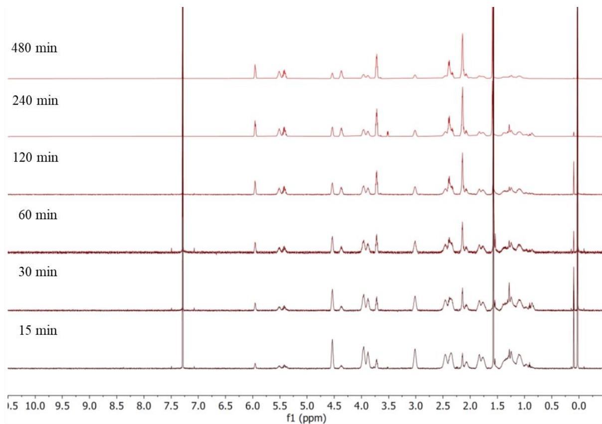
**Figure S14.** <sup>1</sup>H NMR spectra of **P1-H** at different sonication times.
