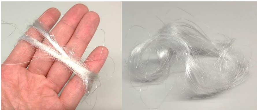
Fig. S18 polymer strands after extrusion of the polymer melt and spinning-up the material on the Haul-off apparatus
