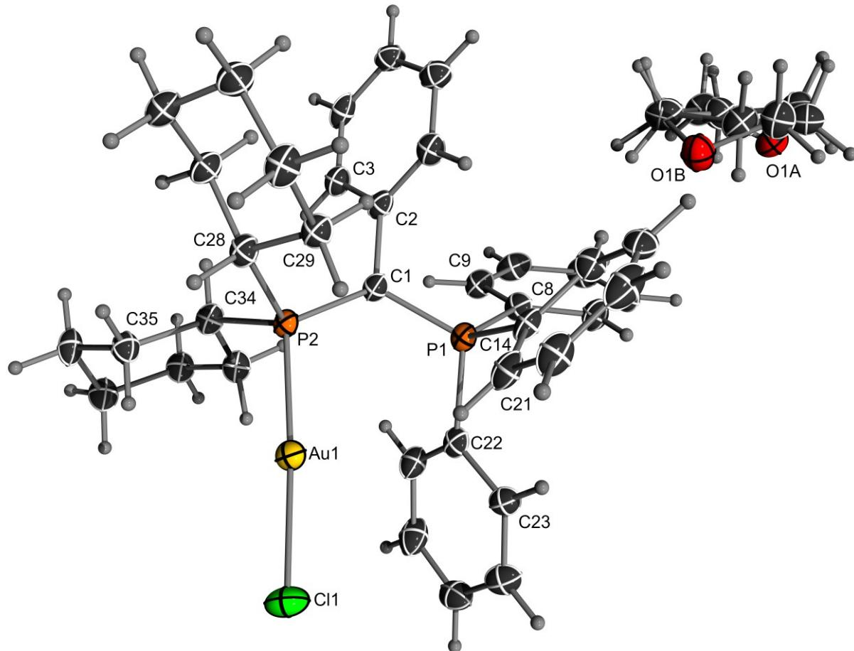
Figure 3.6: ORTEP of  $\text{Y}_{\text{Ph}}\text{PCy}_2\bullet\text{AuCl}$  (1•AuCl) Ellipsoids are drawn at the 50% probability level.
