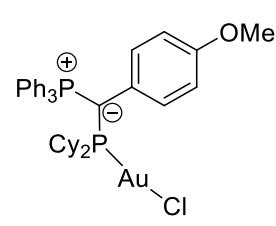
100 mg (173  $\mu\text{mol}$ ) phosphonium ylide **Y<sub>pOMe</sub>PCy<sub>2</sub>** (**2**) and 52.6 mg (164  $\mu\text{mol}$ , 0.95 eq.) (THT)AuCl were dissolved in 4 mL acetonitrile and the yellow suspension was stirred for 16 h. The suspension became clear and a white precipitate formed. The solution was filtered through cannula and the remaining white solid was dried *in vacuo* to afford pure product (91.3 mg, 113  $\mu\text{mol}$ , 65 %).
