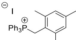
7.5 g (28.8 mmol) triphenylphosphine and 7.56 g (28.8 mmol) 2-(iodomethyl)-1,3,5-trimethylbenzene were dissolved in 125 mL toluene. The solution was refluxed for 24 h and the thus formed precipitate was filtered off. The white solid was dried *in vacuo* to afford pure product (13.8 g, 26.4 mmol, 92 %).
