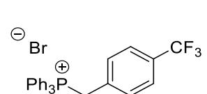
1.00 g (3.81 mmol) triphenylphosphine were dissolved in 50 mL toluene. While stirring 0.58 mL (3.81 mmol) 4-(trifluoromethyl)benzylbromide were added dropwise to the solution. The solution was refluxed for 24 h and the thus formed precipitate was filtered off and washed with 5 mL toluene. The colorless solid was dried *in vacuo* to afford pure product (1.60 g, 3.19 mmol, 84 %).
