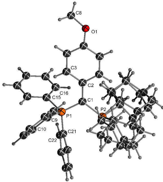
Figure 3.2: ORTEP of  $\text{Y}_{\text{pOMe}}\text{PCy}_2$  (**2**). Ellipsoids are drawn at the 50% probability level.
