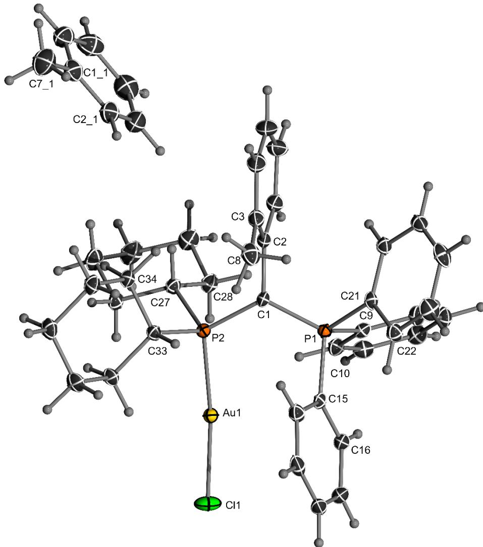
Figure 3.9: ORTEP of  $\text{Y}_{\text{oTol}}\text{PCy}_2 \cdot \text{AuCl}$  (**4**· $\text{AuCl}$ ) Ellipsoids are drawn at the 50% probability level.
