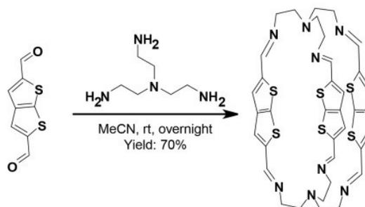
**Scheme S1.** Synthetic scheme of the ThT-cage.
