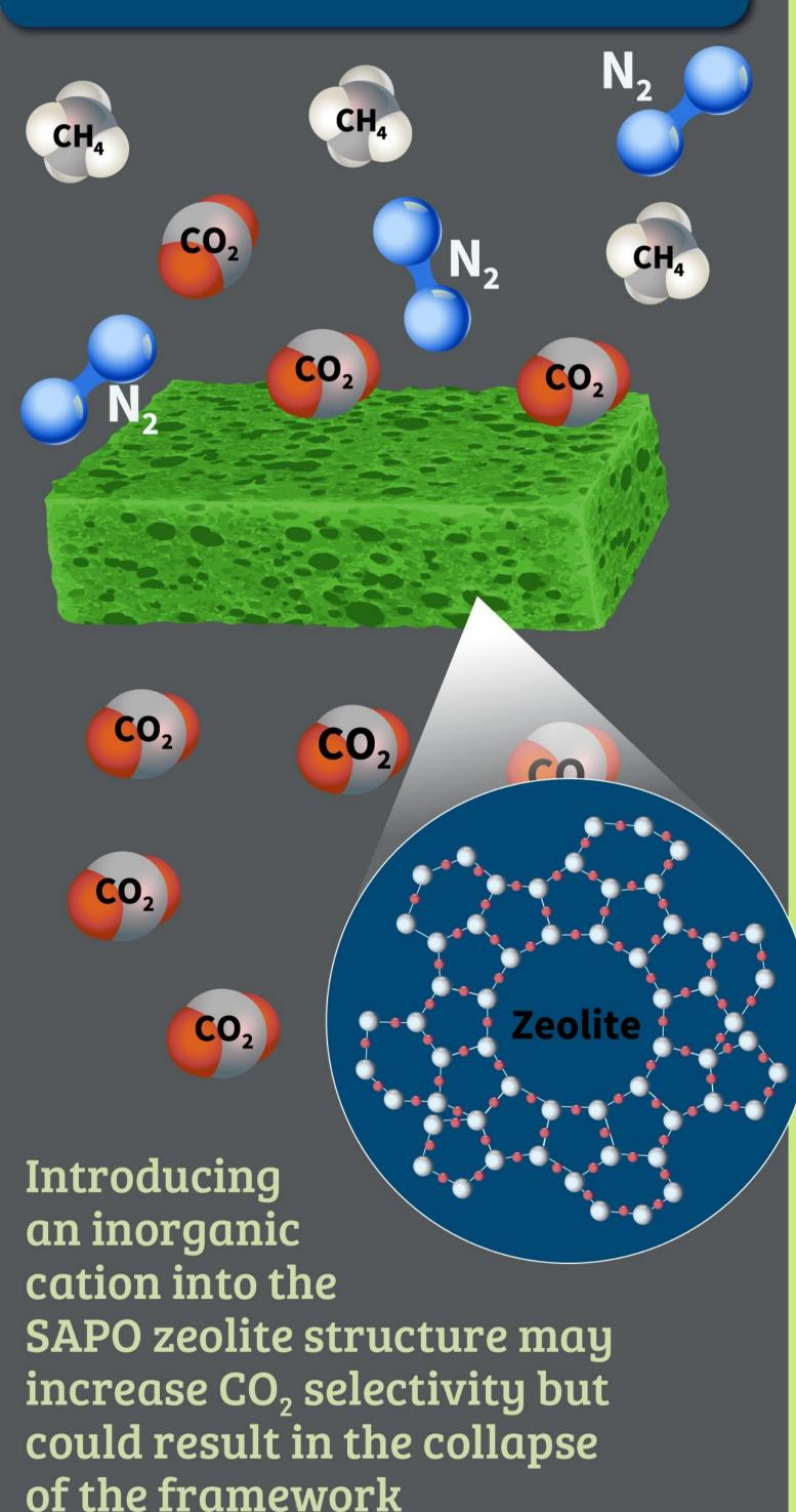
A novel SAPO zeolite with cation-induced trapdoor effect for separation of CO, from methane (CH,) and nitrogen (N<sub>2</sub>) is reported using a direct ion-exchange approach
