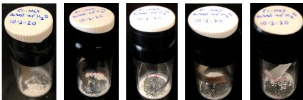
**Figure S82.** Progression of  $H_2S$  release into ambient air from  $H_2S$ -loaded Zr-mes- $H_2O$  over the course of 5 days. Each image was taken after replacing the previous lead test strip with a new one at 24-hour intervals. The strip turned black for the first 4 days followed by no color change on the 5<sup>th</sup> day, confirming that this MOF releases  $H_2S$  slowly over the course of 4 days in air.
