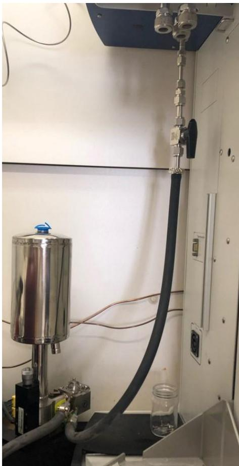
**Figure S107.** DRIFTS experimental setup for dosing Zr-fum-H<sub>2</sub>O with known pressures of H<sub>2</sub>S gas using a Micromeritics 3-Flex gas sorption analyzer.
