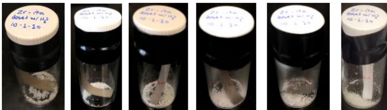
**Figure S83.** Progression of  $H_2S$  release into ambient air from  $H_2S$ -loaded Zr-ita- $H_2O$  over the course of 6 days. Each image was taken after replacing the previous lead test strip with a new one at 24-hour intervals. The strip turned black for the first 5 days followed by no color change on the 6<sup>th</sup> day, confirming that this MOF releases  $H_2S$  slowly over the course of 5 days.
