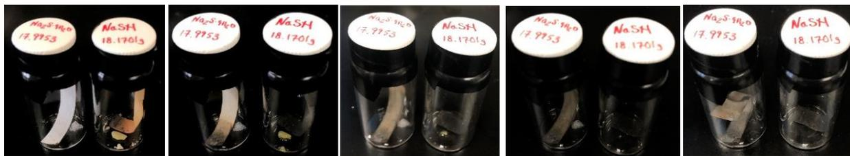
**Figure S84.** Progression of H<sub>2</sub>S release into ambient air from Na<sub>2</sub>S·9H<sub>2</sub>O and NaSH over the course of 5 h. Each image was taken at 1 h intervals, and the lead strip was not changed throughout the duration of the assay. The rapid hydrolysis of both salts in humid air (neither solid remained after 5 h) demonstrates their instability compared to H<sub>2</sub>S-loaded Zr-fum, Zr-mes, and Zr-ita.
