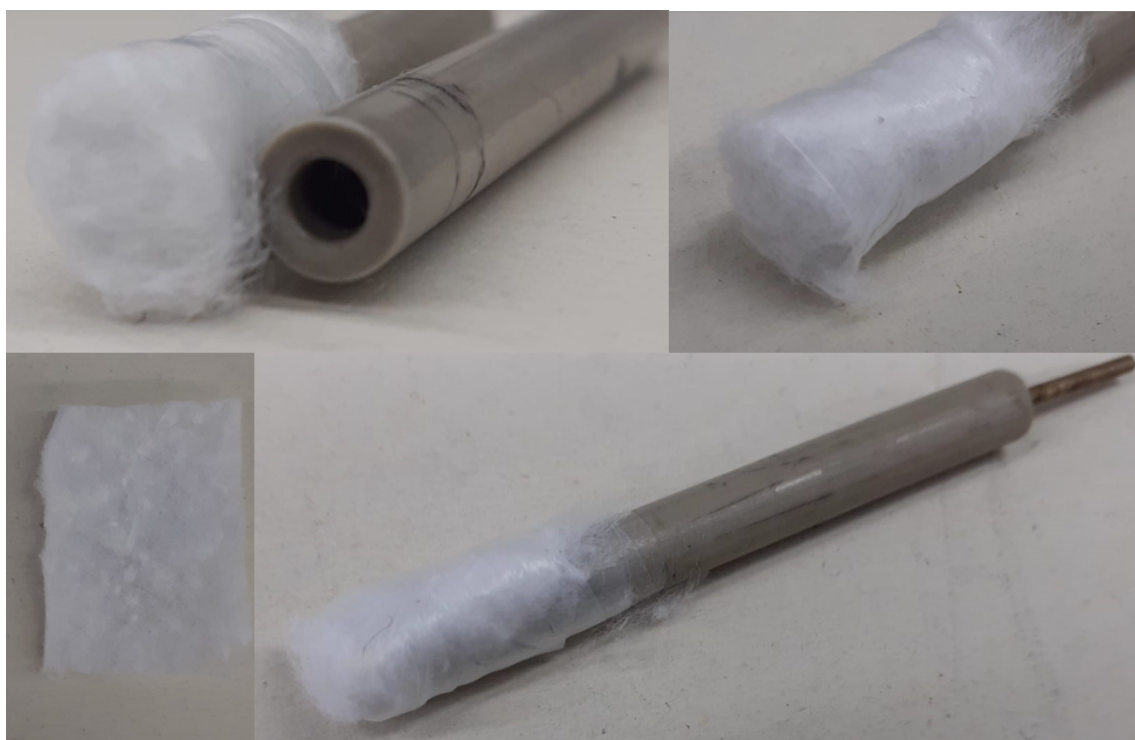
Figure S1. Images of the electrode preparative for long-term electrocatalytic experiments to avoid the expulsion of the blend out of the electrode pocket.
