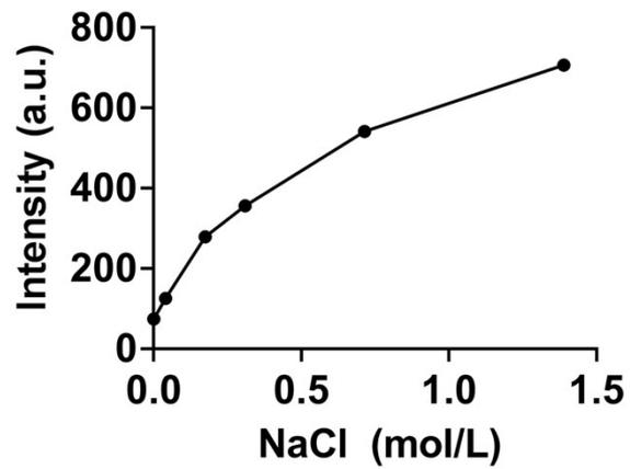
**Figure S1.** Fluorescence intensity of Ce6 in D-KCD/A nanoparticles in different salt solutions. The excitation wavelength of Ce6 is 400 nm.
