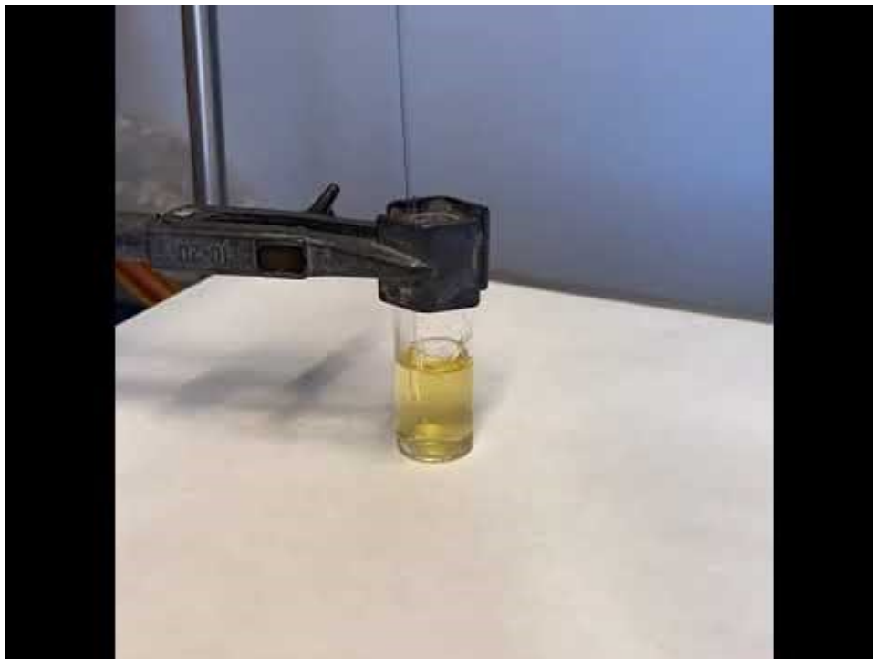
Video S1. Decarboxylation of 0.020 M nitroacetic acid 1 in the presence of 0.010 NaOH ( \mu = 0.50 M, T = 20^\circ\text{C} ). Reaction followed by means of bromocresol green as an indicator.
