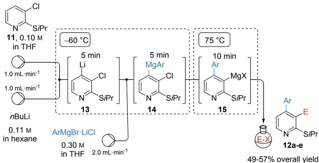
**Figure SI1:** Flow chemistry set-up for the preparation of 2,3,4-trifunctionalized pyridines of type **12**.
