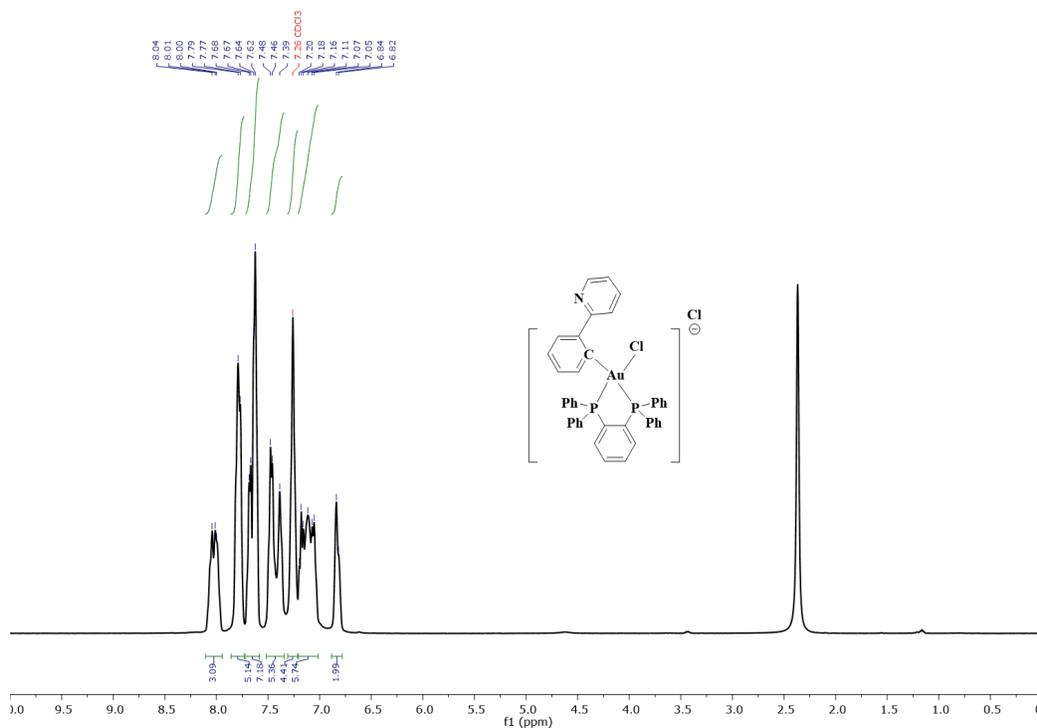
**Figure S22.**  $^1\text{H}$  NMR spectrum of complex AuPhos-89 in  $\text{CDCl}_3$  at 298K
