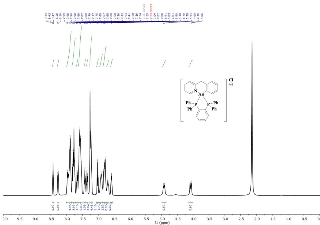
Figure S7. <sup>1</sup>H NMR spectrum of complex AuPhos-83 in CDCl<sub>3</sub> at 298K
