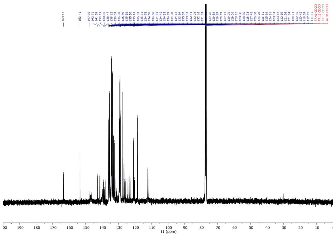
Figure S5.  $^{13}\text{C}\{^1\text{H}\}$  NMR spectrum of complex AuPhos-82 in  $\text{CDCl}_3$  at 298K
