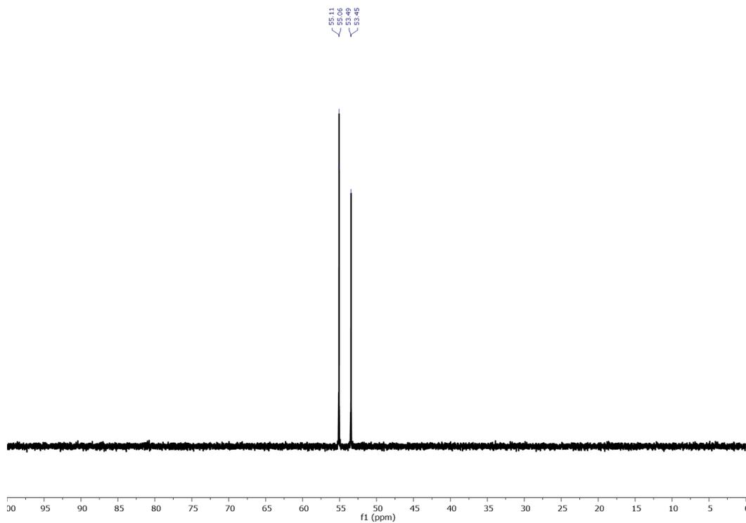
Figure S12.  $^{31}\text{P}\{^1\text{H}\}$  NMR spectrum of complex AuPhos-84 in  $\text{CDCl}_3$  at 298K
