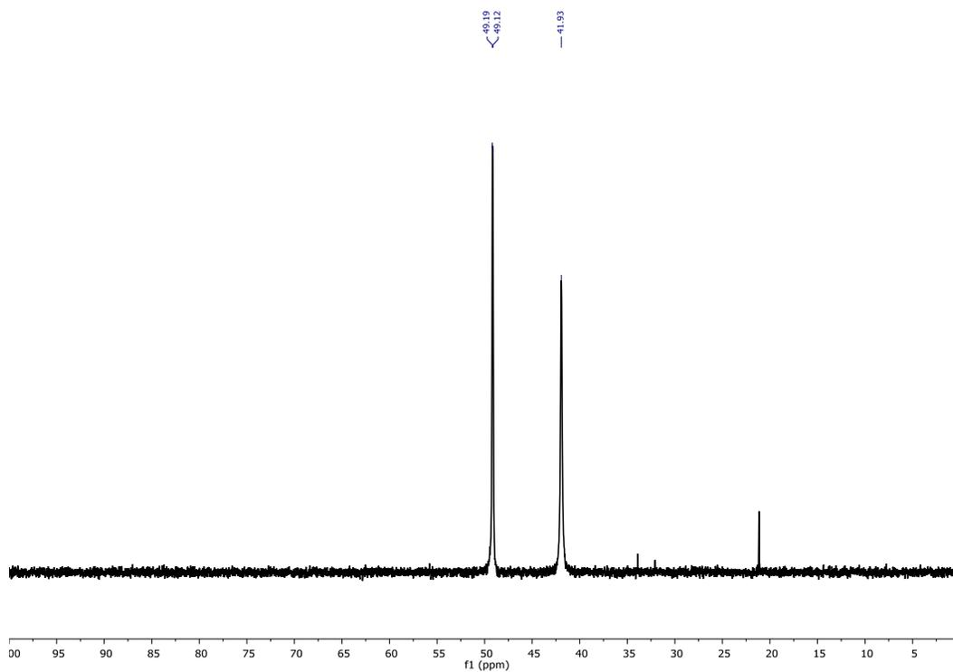
**Figure S3.**  $^{31}\text{P}\{^1\text{H}\}$  NMR spectrum of complex AuPhos-81 in  $\text{CDCl}_3$  at 298K, impurity at 34, 32 & 21 ppm
