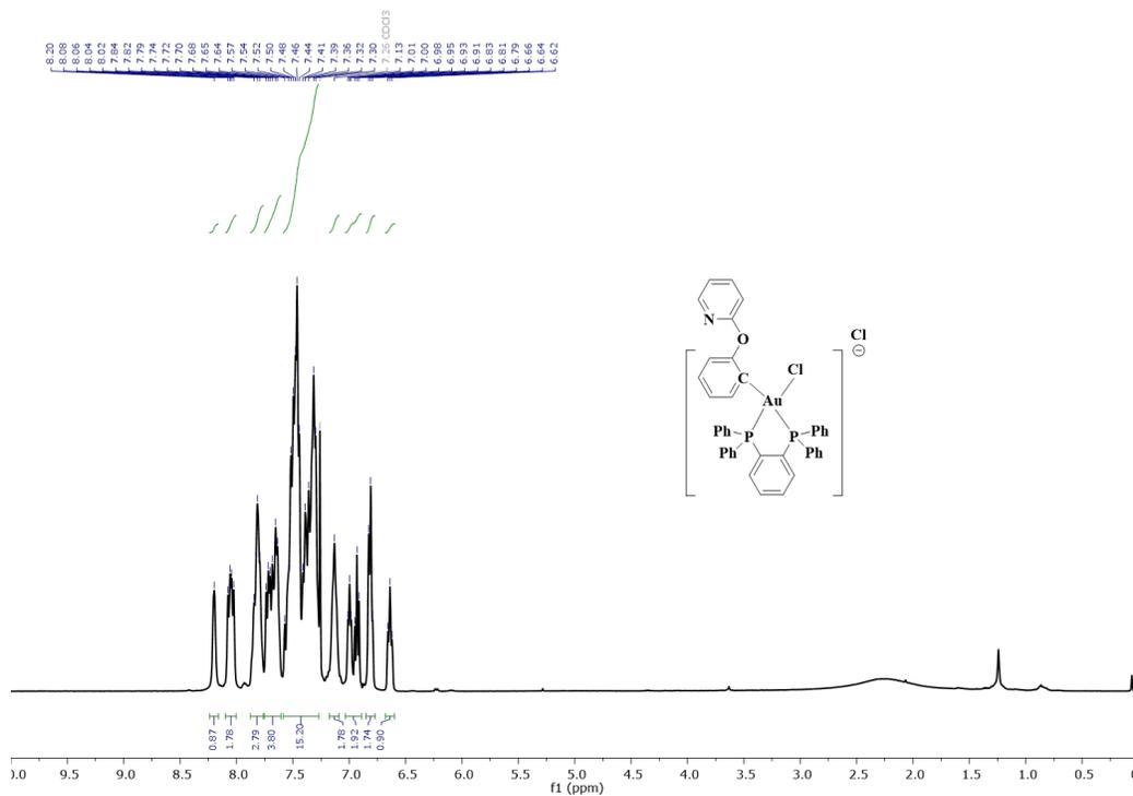
**Figure S4.**  $^1\text{H}$  NMR spectrum of complex AuPhos-82 in  $\text{CDCl}_3$  at 298K
