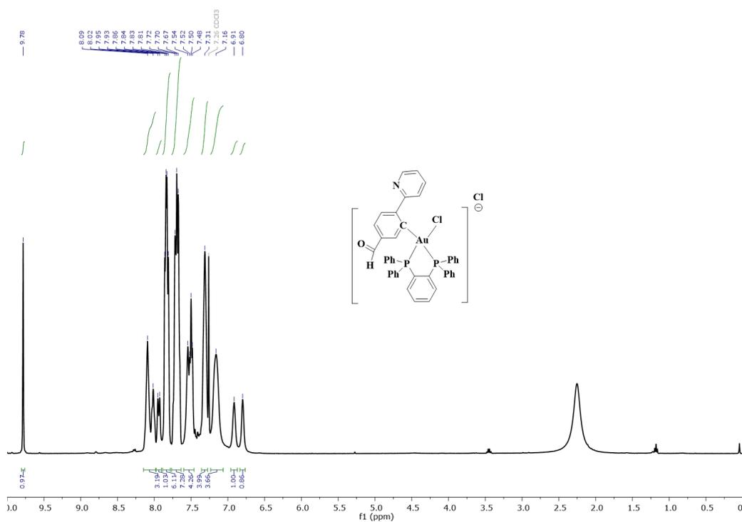
Figure S19.  $^1\text{H}$  NMR spectrum of complex AuPhos-88 in  $\text{CDCl}_3$  at 298K
