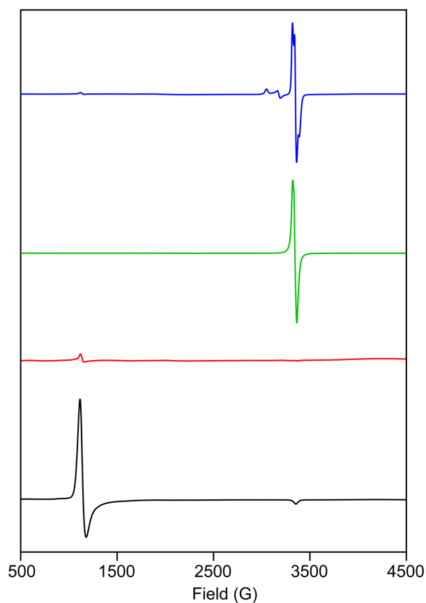
Figure S3. EPR spectral features (in frozen THF at 7 K) for 2 mM solutions of [(F_{20}TPP)Fe^{III}(O_2^-)] (red), compared to that of a [(F_{20}TPP)Fe^{III}(Cl)] (black) ( g = 5.9, 2.0 ); TEMPO radical (green) ( g = 2.0 ), and the final heme product from the reaction between [(F_{20}TPP)Fe^{III}(O_2^-)] and TEMPO-H (blue).
