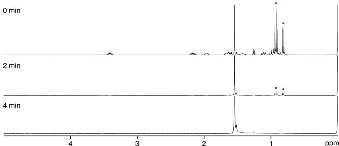
**Figure S48d.** Time-dependent <sup>1</sup>H NMR spectra (400 MHz, CDCl<sub>3</sub>, r.t., coronene as an internal standard) of **MTL** (solid) before/after heating at 80 °C under vacuum (480 Pa) for 2 and 4 min.
