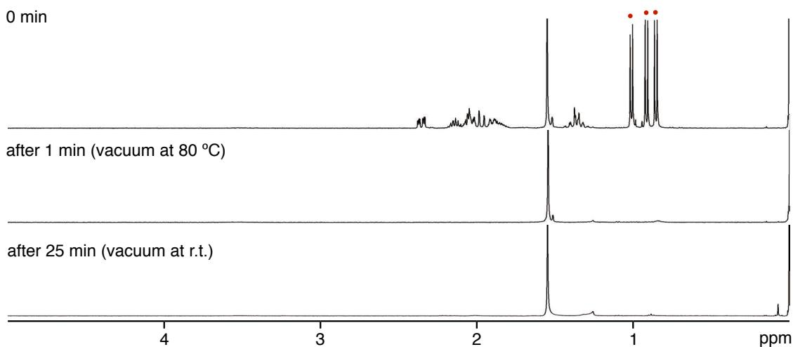
**Figure S48b.** Time-dependent <sup>1</sup>H NMR spectra (400 MHz, CDCl<sub>3</sub>, r.t., coronene as an internal standard) of **MTO** (neat) before/after heating at 80 °C under vacuum (480 Pa) for 1 min or standing at r.t. for 25 min.
