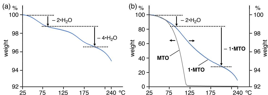
**Figure S49.** Thermogravimetry (TG) curves (heating rate of 10 °C/min from 25 °C to 240 °C) of (a) **1** and (b) MTO and **1•MTO**.
