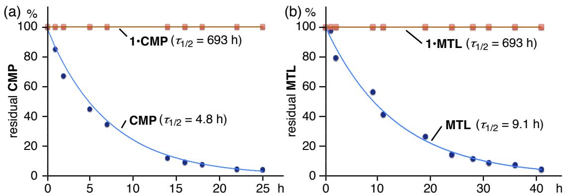
**Figure S47e.** Time-course volatility profiles (%) of (a) **CMP** and (b) **MTL** within/without **1** in water at 80 °C and their half-life times.
