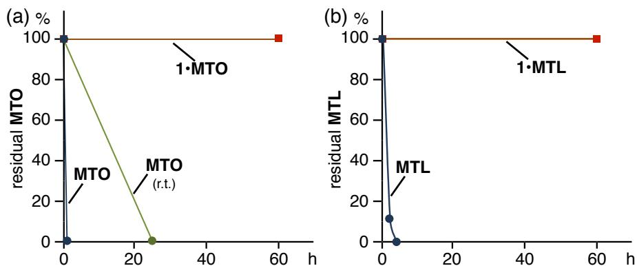
**Figure S48e.** Time-course volatility profiles (%) of MTO or MTL from (a) solid **1•MTO** and MTO (neat), and (b) solid **1•MTL** and MTL (neat) at 80 °C (or r.t.) under vacuum (480 Pa).
