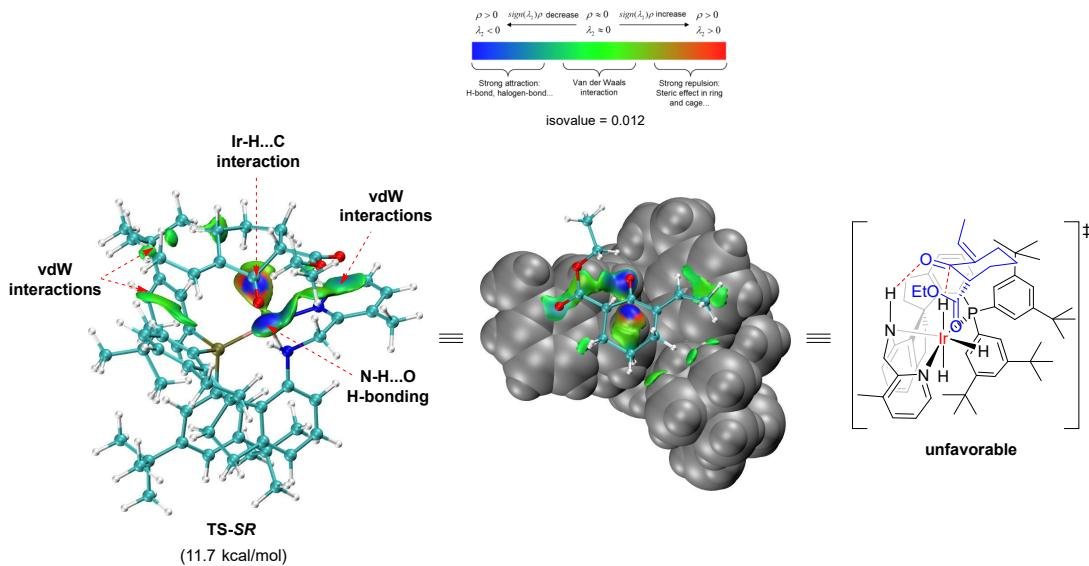
**Figure S4** Intermolecular NCIs in **TS-SR** as visualized by VMD
