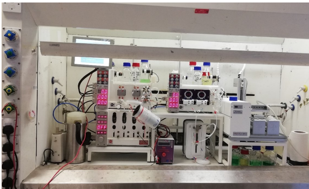
Figure S6: Picture of the automated electrolysis machine. The machine has 4 pumps (HPLC/peristaltic), an autosampler/fraction collector, galvanostat, backpressure regulators etc. that can all be remotely controlled via a PC.
