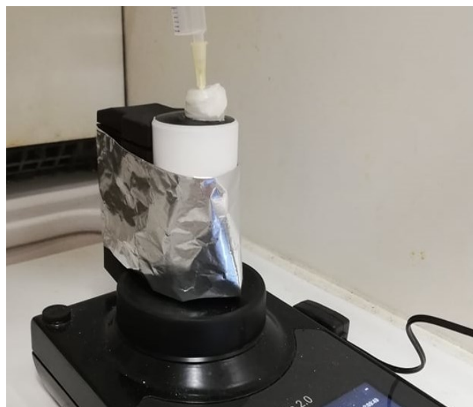
Figure S2: The electrochemical vial was shaded from light by a foil wrap. The fume cupboard light was switched off, and the vial purged with argon throughout.
