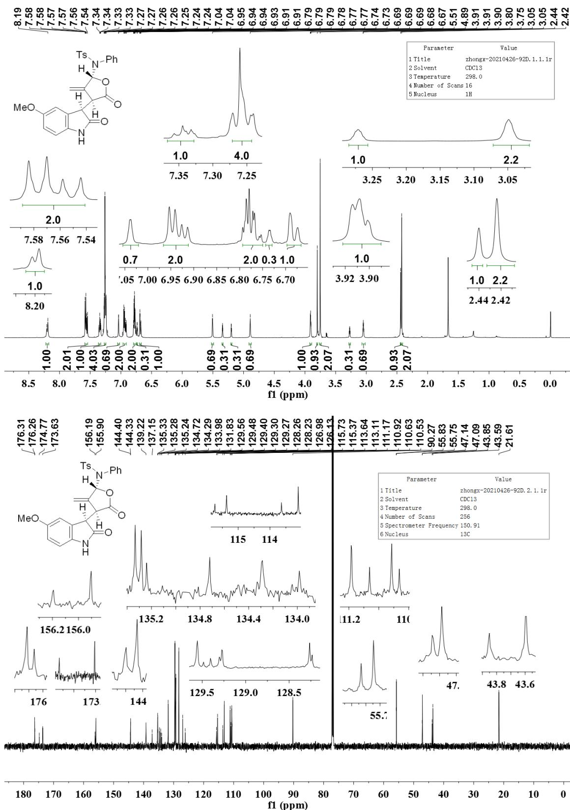
$^1\text{H}$  NMR and  $^{13}\text{C}\{\text{H}\}$  NMR spectra of compound **5ia** in  $\text{CDCl}_3$
