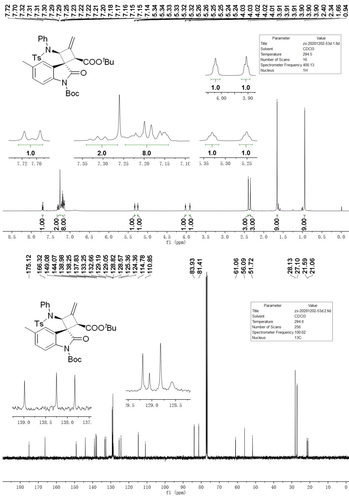
$^1\text{H}$  NMR and  $^{13}\text{C}\{\text{H}\}$  NMR spectra of compound **4fa** in  $\text{CDCl}_3$
