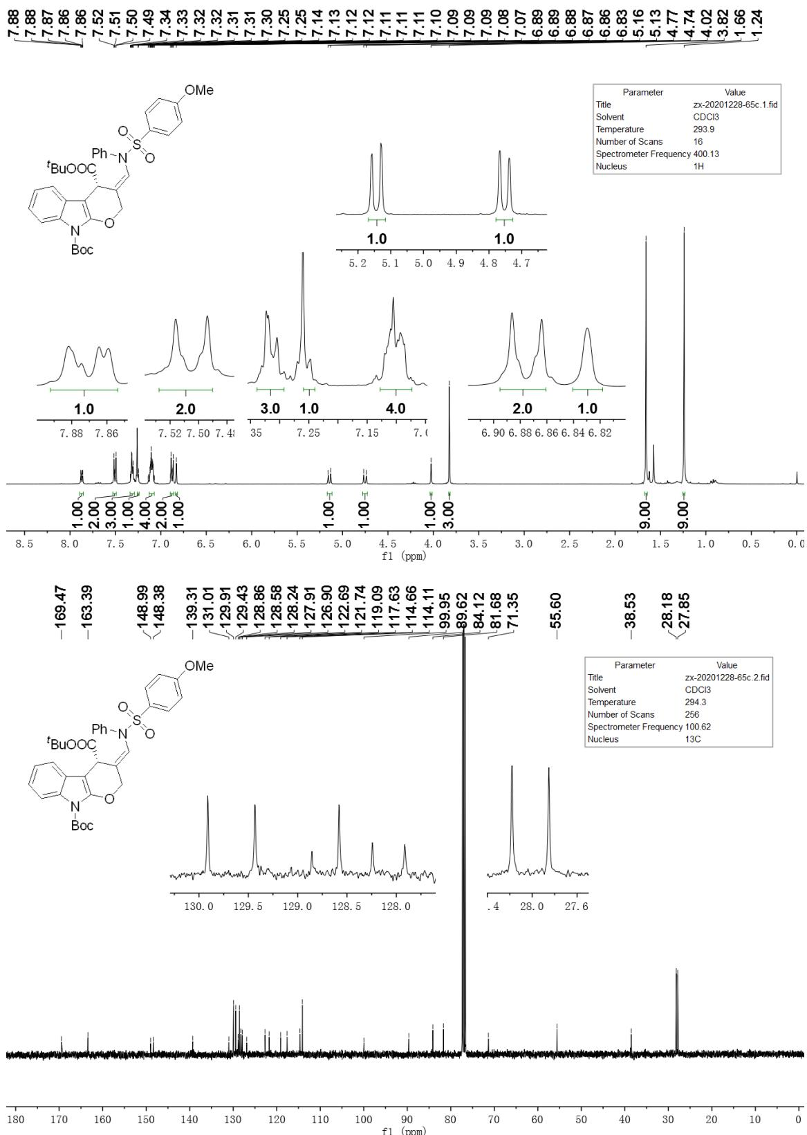
$^1\text{H}$  NMR and  $^{13}\text{C}\{^1\text{H}\}$  NMR spectra of compound **3ad** in  $\text{CDCl}_3$
