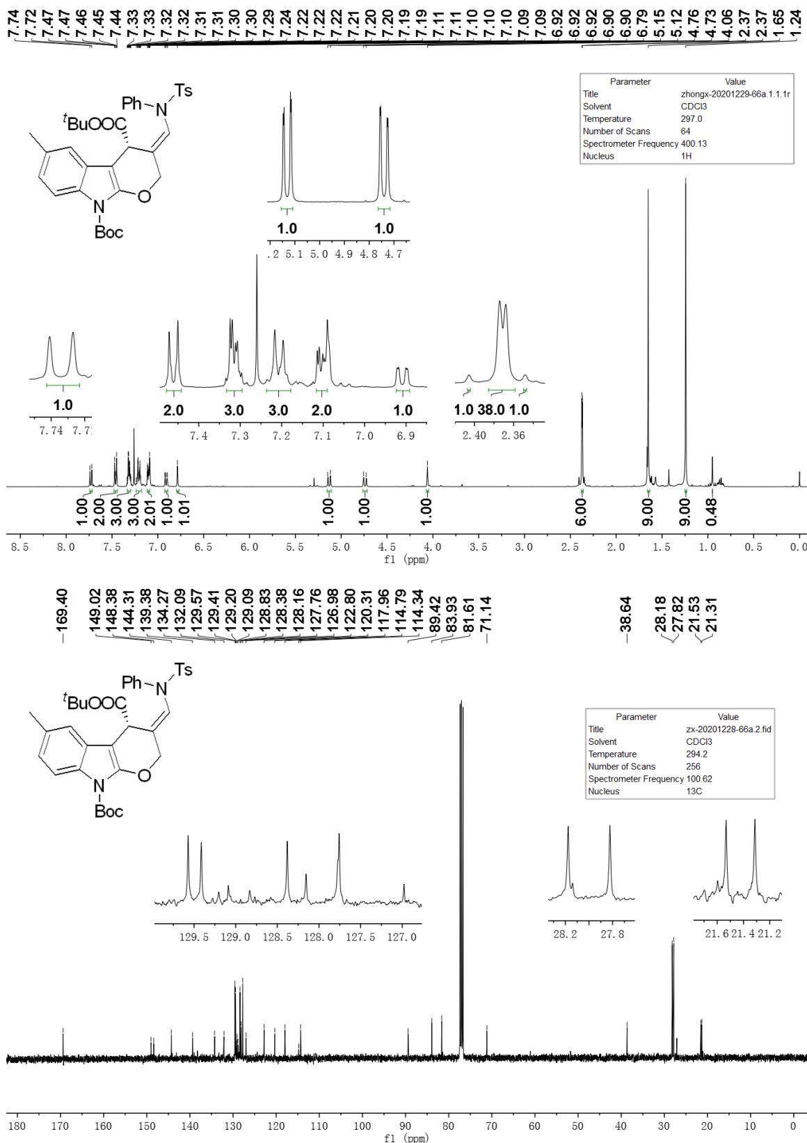
$^1\text{H}$  NMR and  $^{13}\text{C}\{\text{H}\}$  NMR spectra of compound **3ga** in  $\text{CDCl}_3$
