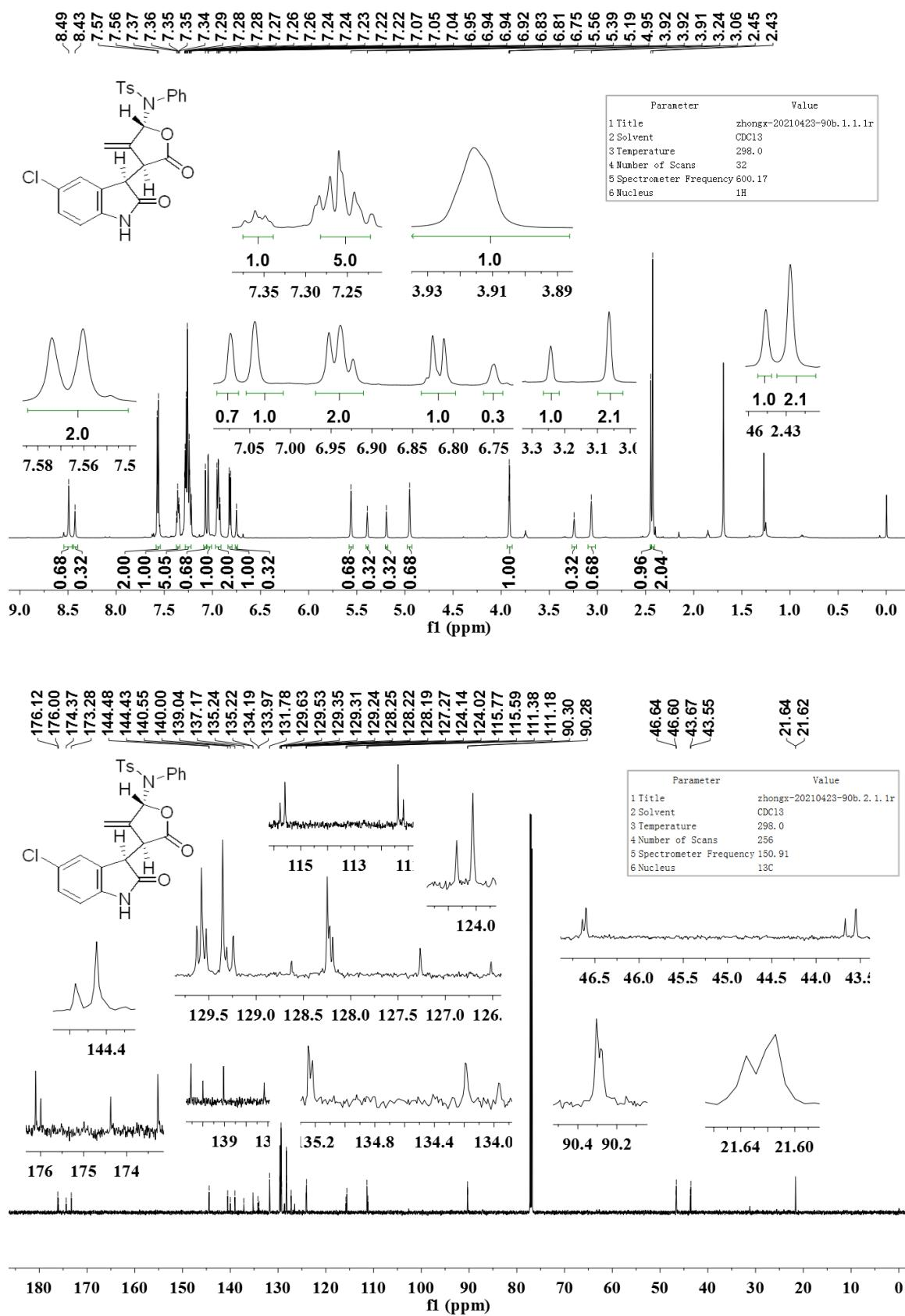
$^1\text{H}$  NMR and  $^{13}\text{C}\{\text{H}\}$  NMR spectra of compound **5na** in  $\text{CDCl}_3$
