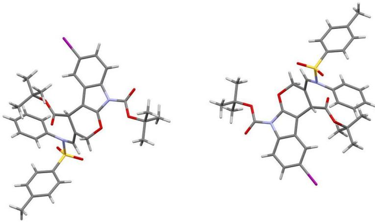
**Figure S2.** X-ray Crystal Structure of Product **rac-4ka**
