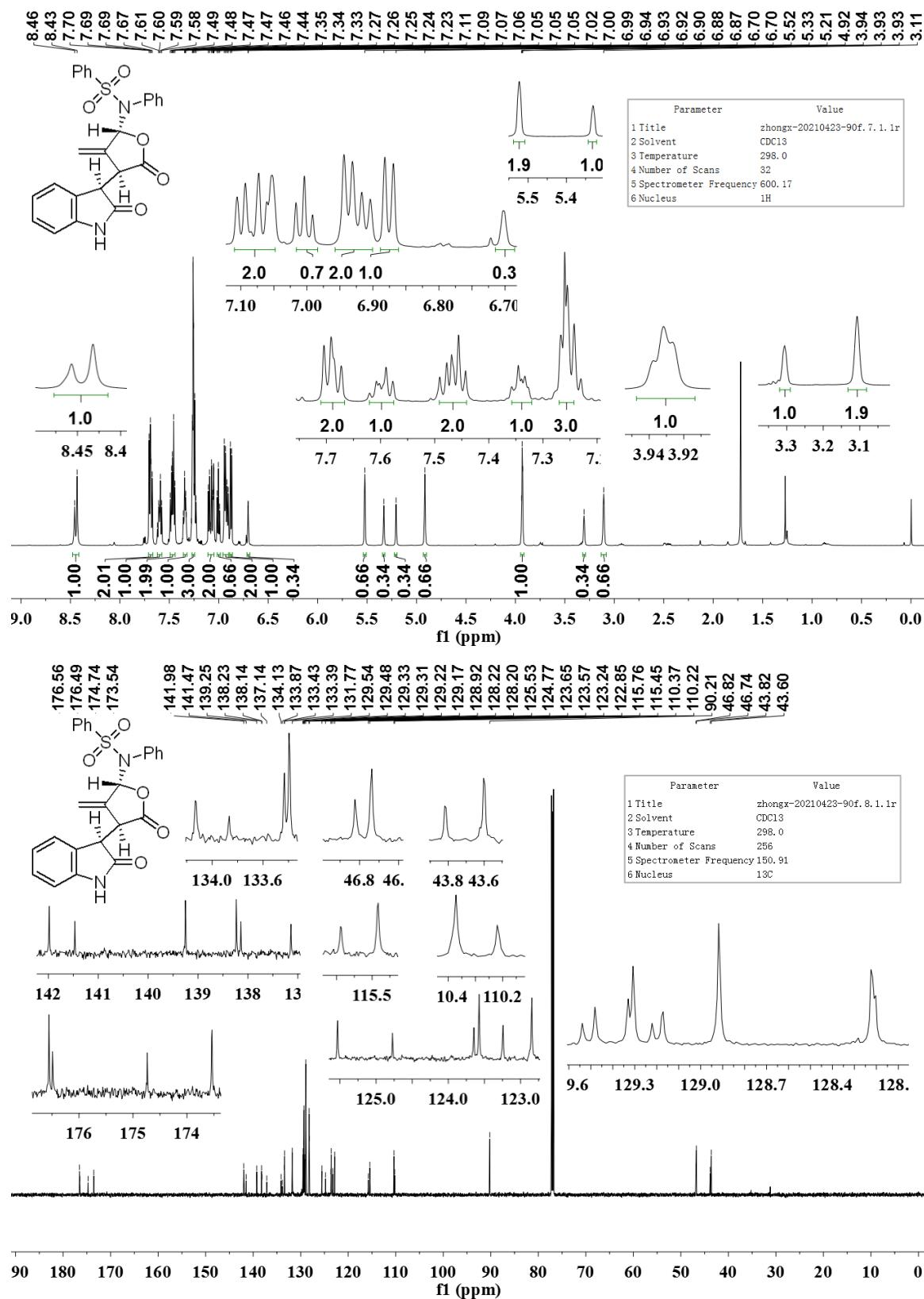
$^1\text{H}$  NMR and  $^{13}\text{C}\{\text{H}\}$  NMR spectra of compound **7aa** in  $\text{CDCl}_3$
