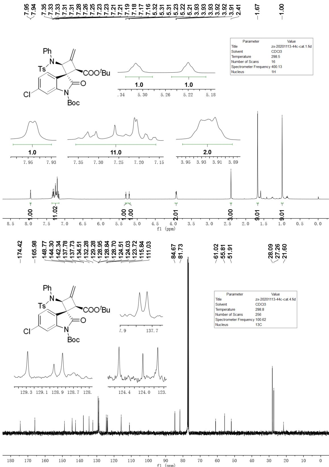
$^1\text{H}$  NMR and  $^{13}\text{C}\{^1\text{H}\}$  NMR spectra of compound **4na** in  $\text{CDCl}_3$
