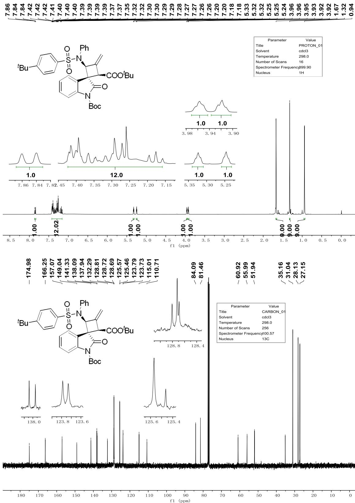
$^1\text{H}$  NMR and  $^{13}\text{C}\{^1\text{H}\}$  NMR spectra of compound **4ad** in  $\text{CDCl}_3$
