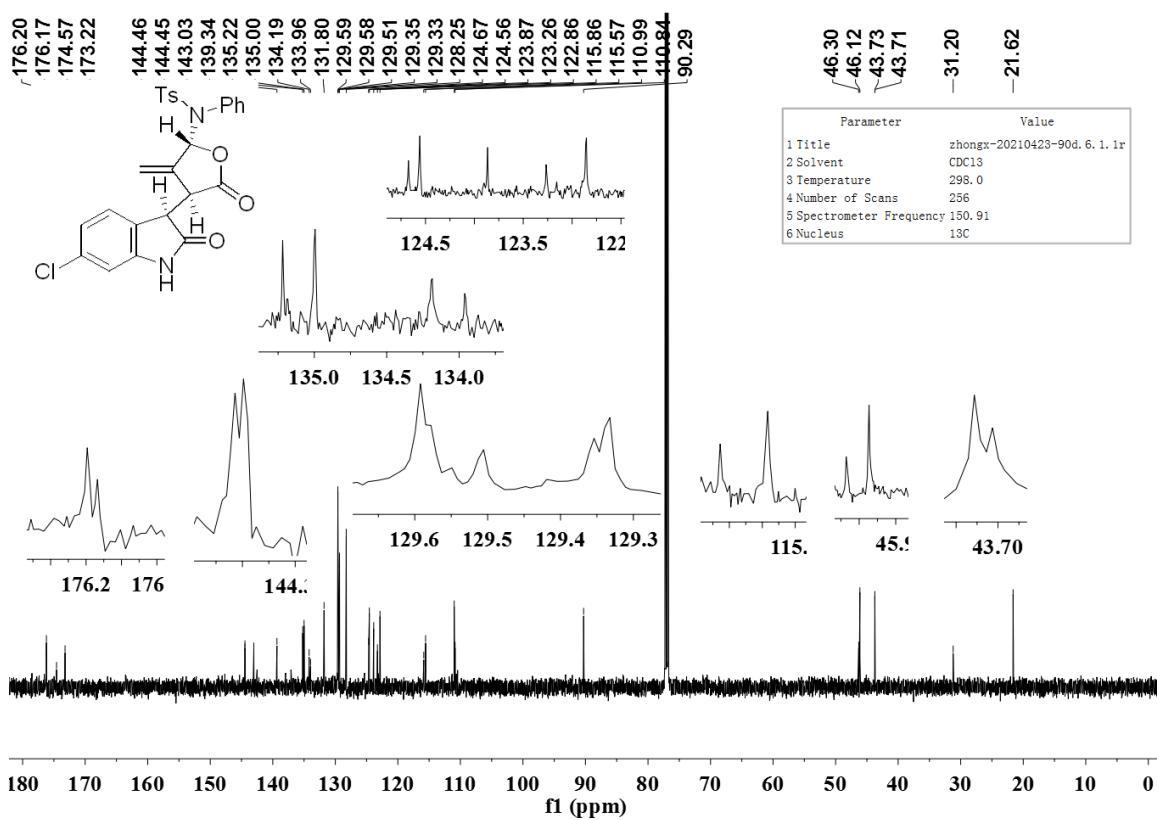
$^1\text{H}$  NMR and  $^{13}\text{C}\{^1\text{H}\}$  NMR spectra of compound **5ab** in  $\text{CDCl}_3$
