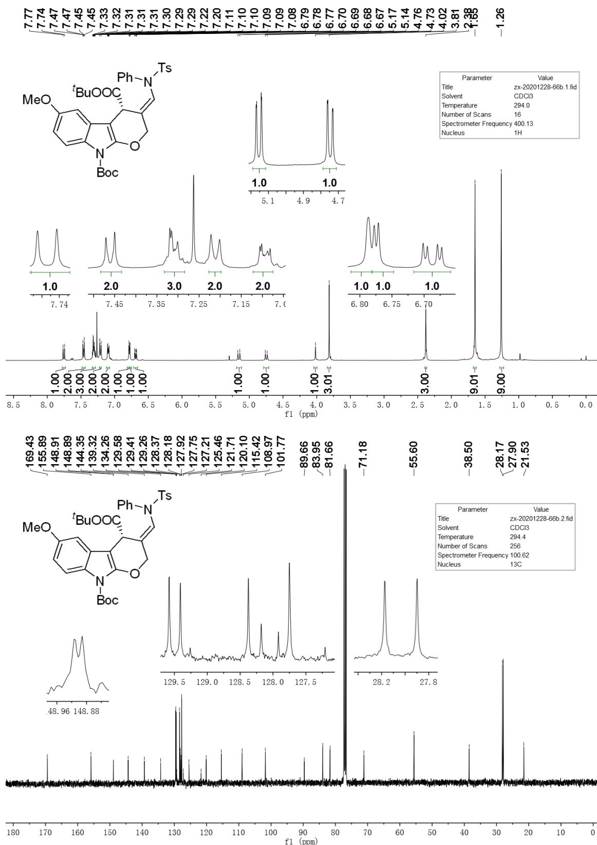
$^1\text{H}$  NMR and  $^{13}\text{C}\{^1\text{H}\}$  NMR spectra of compound **3ha** in  $\text{CDCl}_3$
