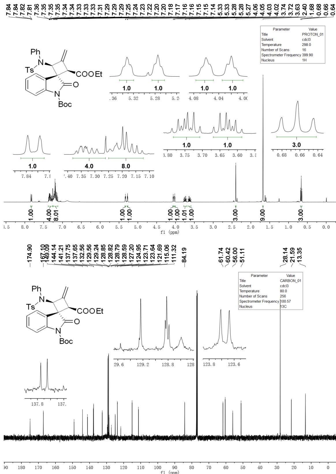
$^1\text{H}$  NMR and  $^{13}\text{C}\{^1\text{H}\}$  NMR spectra of compound **4ca** in  $\text{CDCl}_3$
