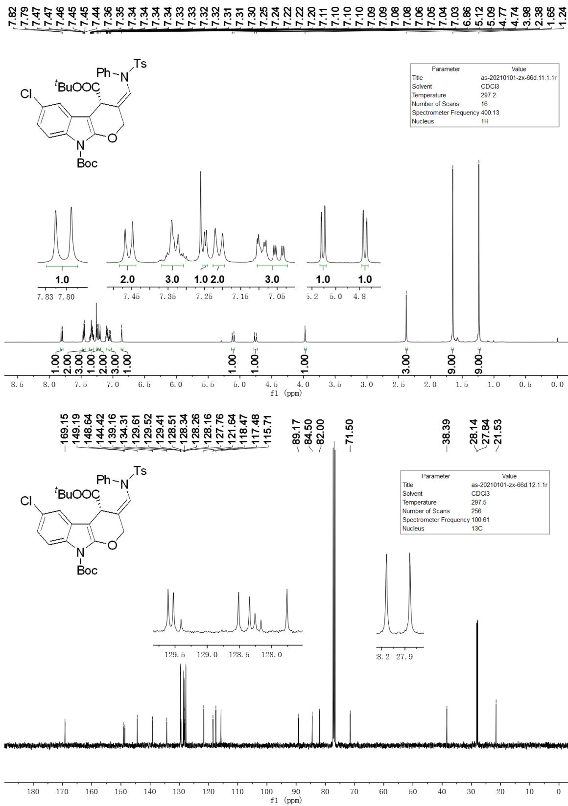
$^1\text{H}$  NMR and  $^{13}\text{C}\{\text{H}\}$  NMR spectra of compound **3ja** in  $\text{CDCl}_3$
