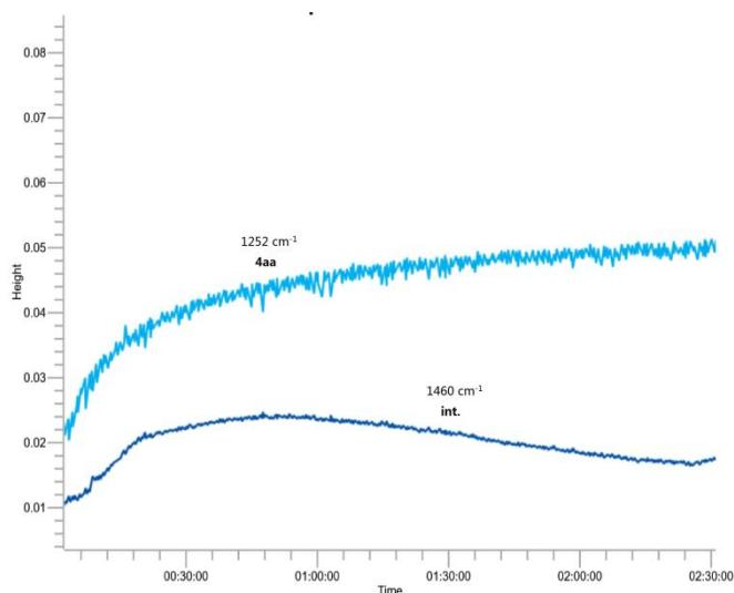
**Figure S10.** The trend of each component (X axes: reaction time; Y axes: absorbance unit). **4aa:** peak at  $1252 \text{ cm}^{-1}$ ; intermediate **int.:** peak at  $1420 \text{ cm}^{-1}$ .
