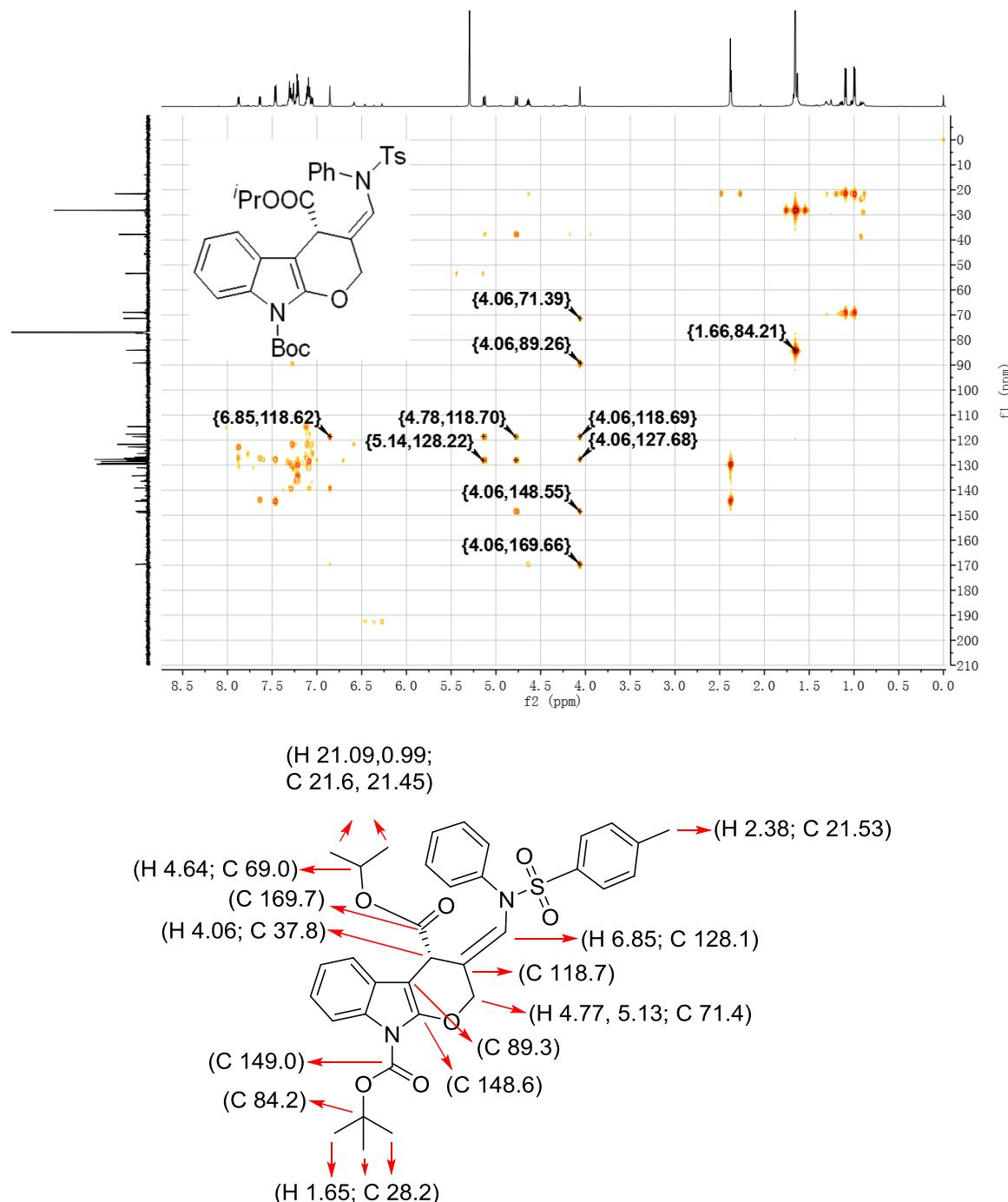
$^1\text{H}$  NMR and  $^{13}\text{C}\{\text{H}\}$  NMR spectra of compound **3ea** in  $\text{CDCl}_3$
