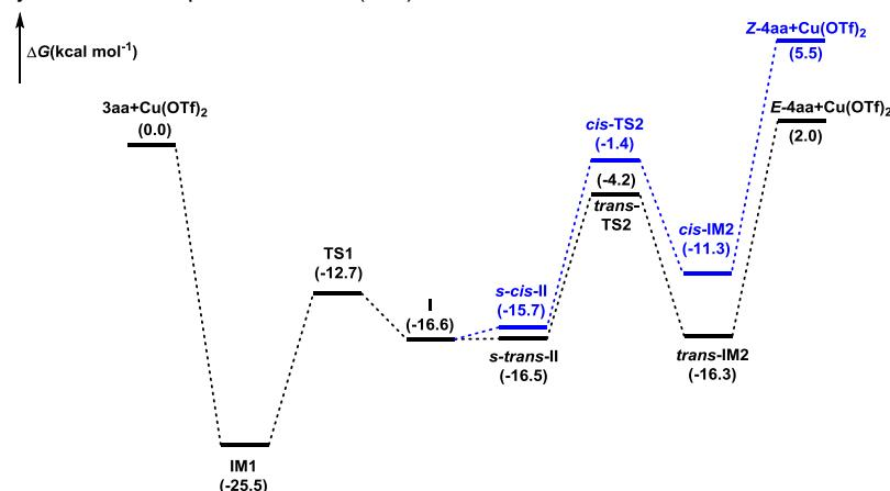
**Figure S12** Energy profiles for the isomerization from **3aa** to **E-4aa** or **Z-4aa** catalyzed by Cu(OTf)<sub>2</sub>. The relative Gibbs free energies (in kcal mol<sup>-1</sup>) were obtained at the M06-D3/6-31G(d,p)(SMD, dichloromethane) theoretical level at 303 K.
