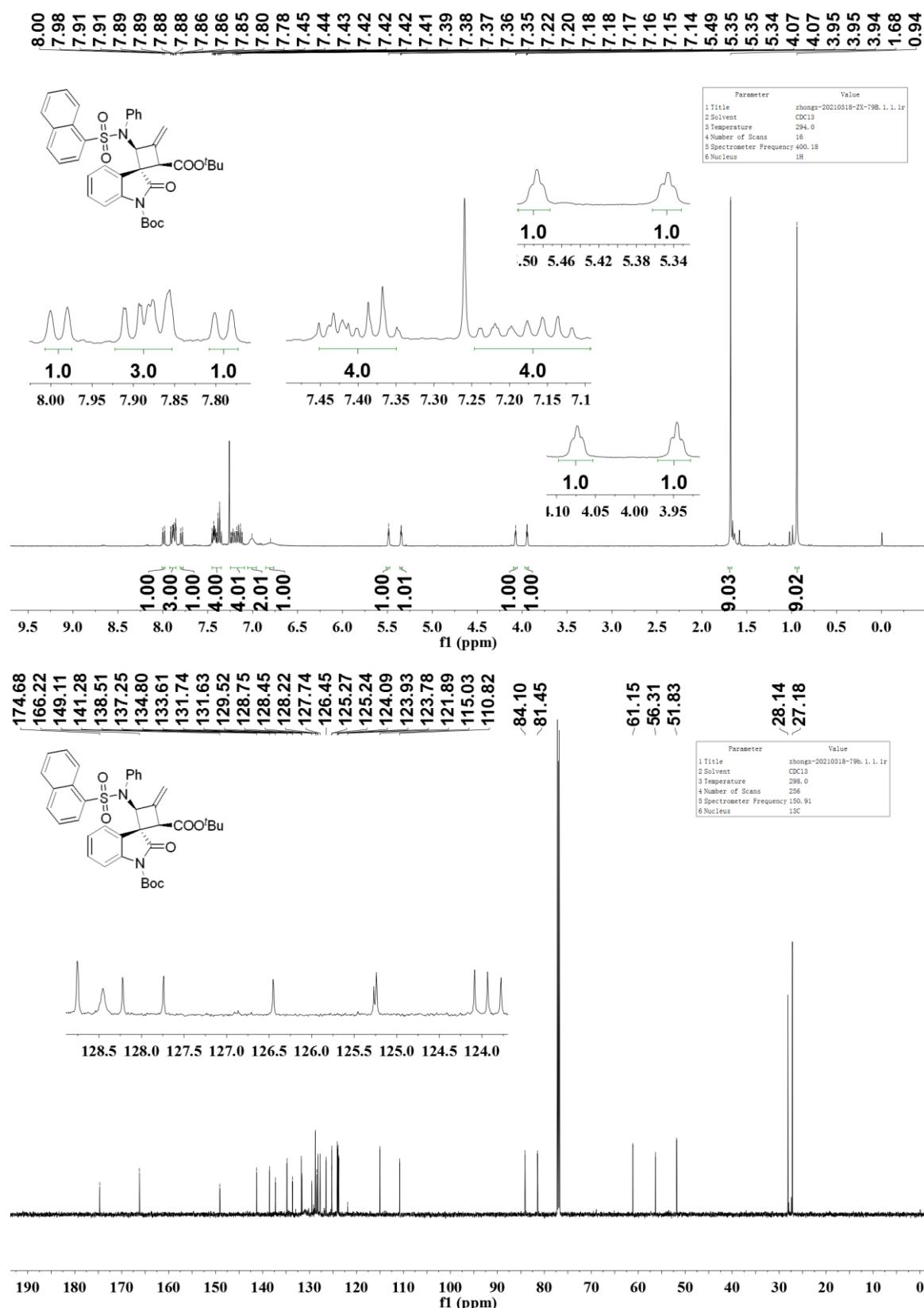
$^1\text{H}$  NMR and  $^{13}\text{C}\{\text{H}\}$  NMR spectra of compound **4ae** in  $\text{CDCl}_3$
