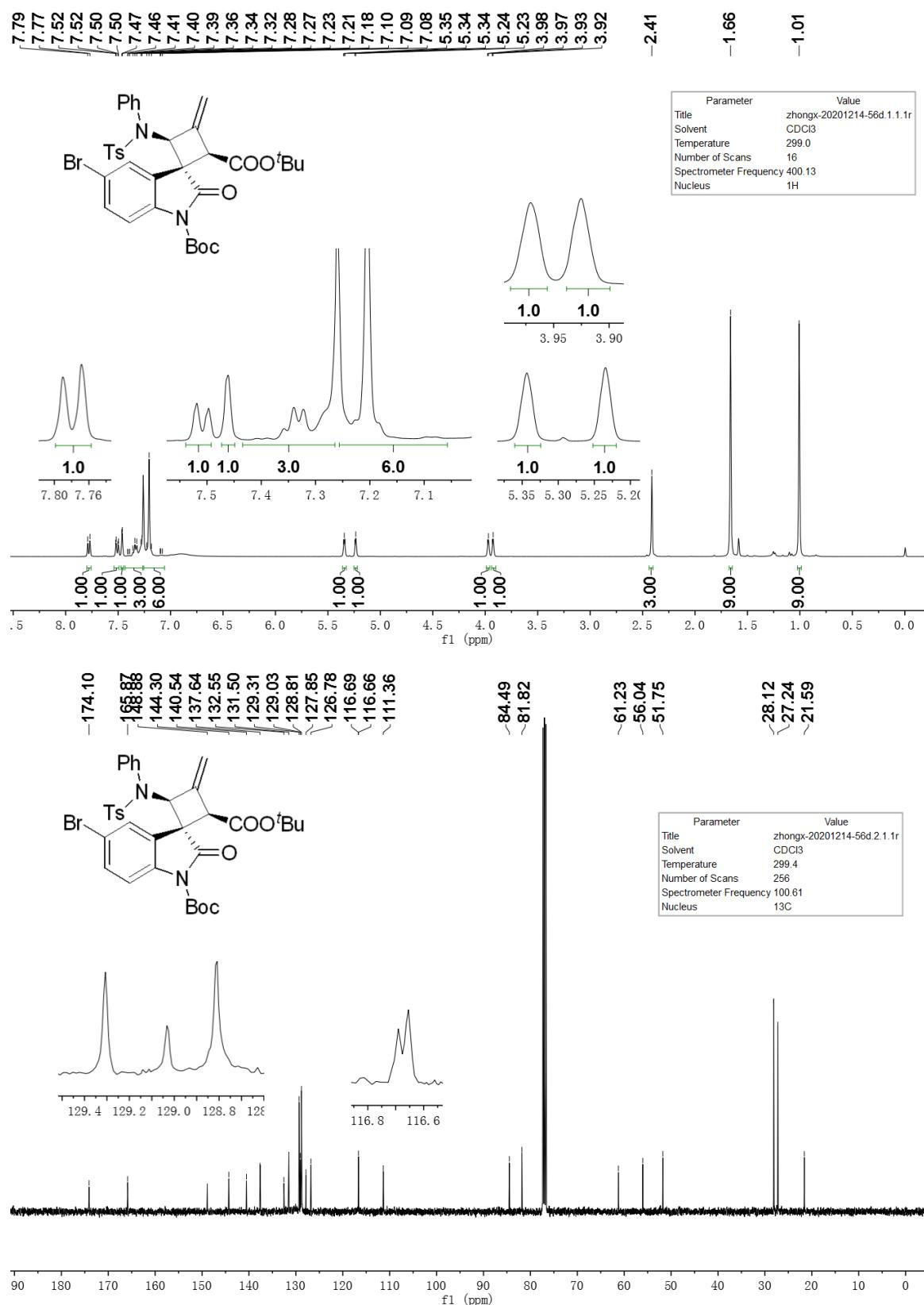
$^1\text{H}$  NMR and  $^{13}\text{C}\{\text{H}\}$  NMR spectra of compound **4ja** in  $\text{CDCl}_3$
