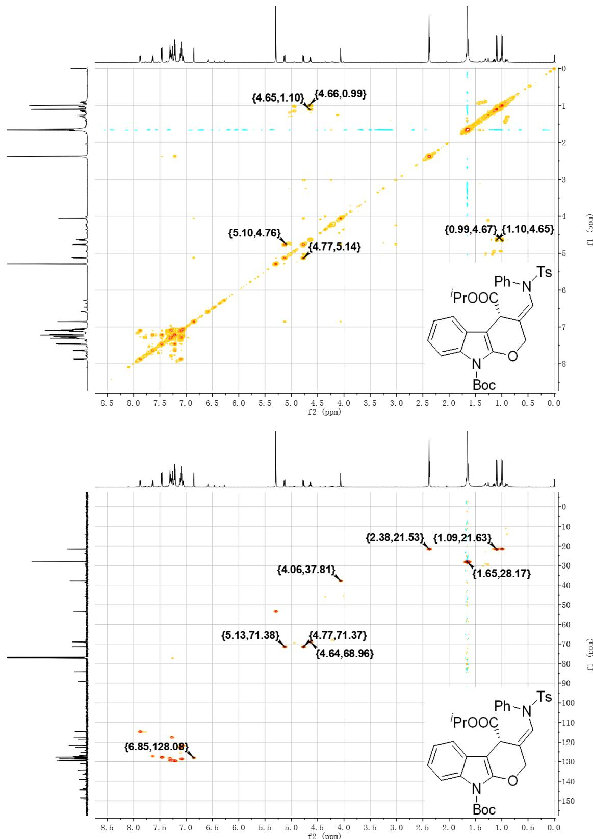
HMBC spectra of compound **4da** in  $\text{CDCl}_3$
