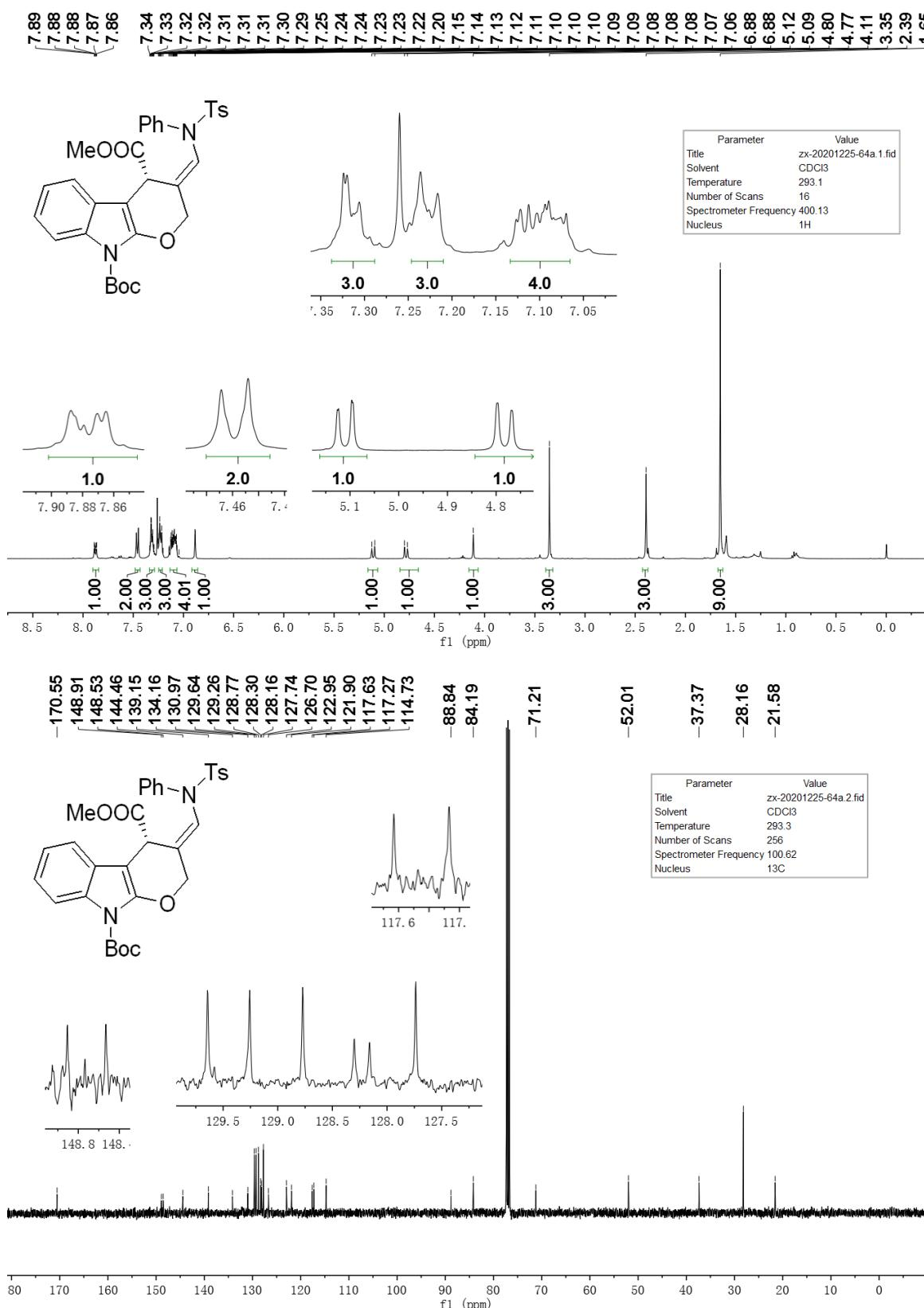
$^1\text{H}$  NMR and  $^{13}\text{C}\{\text{H}\}$  NMR spectra of compound **3ca** in  $\text{CDCl}_3$
