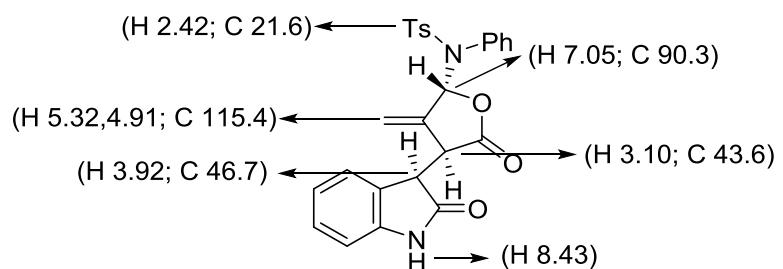
$^1\text{H}$  NMR and  $^{13}\text{C}\{\text{H}\}$  NMR spectra of compound **5ga** in  $\text{CDCl}_3$
