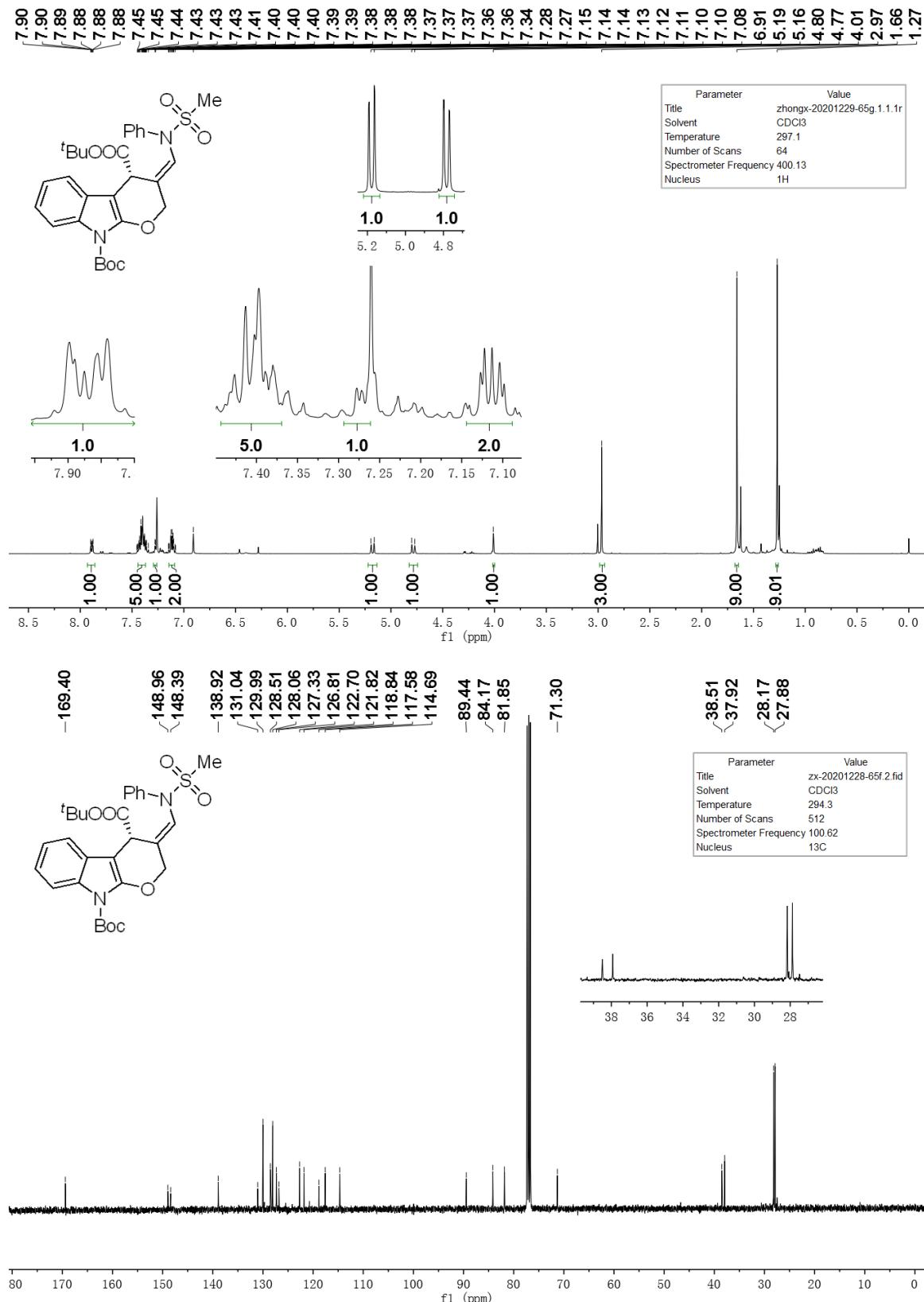
$^1\text{H}$  NMR and  $^{13}\text{C}\{\text{H}\}$  NMR spectra of compound **3ag** in  $\text{CDCl}_3$
