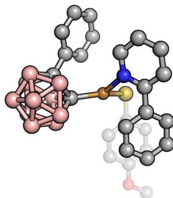
**Figure S1.** Computed structure for the most stable doublet copper(II)-*o*-carborane complex **C**. Nonrelevant hydrogens were omitted for clarity.
