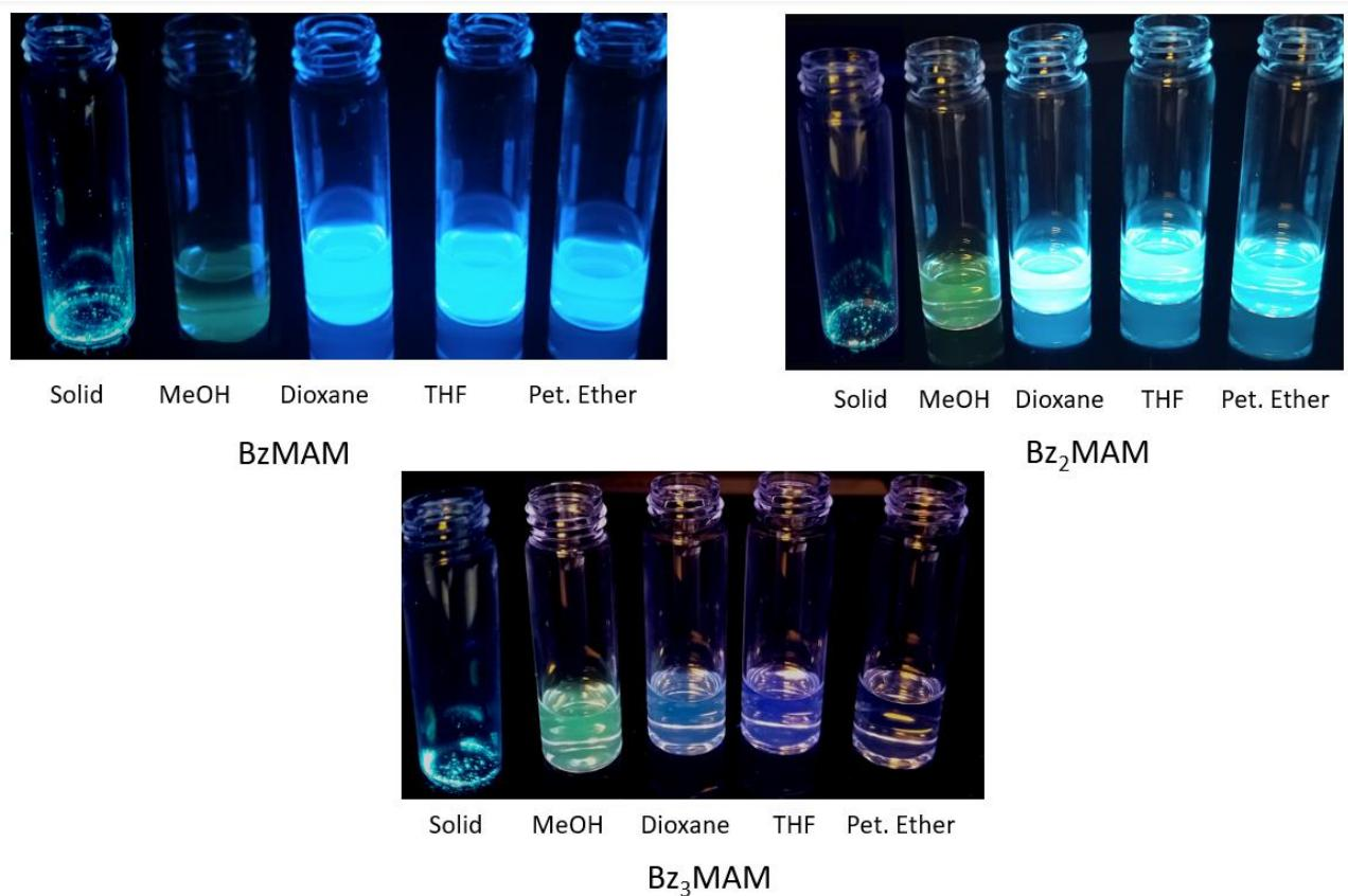
**Figure S13.** Digital photographs of **BzMAM**, **Bz<sub>2</sub>MAM** and **Bz<sub>3</sub>MAM** under UV illumination.
