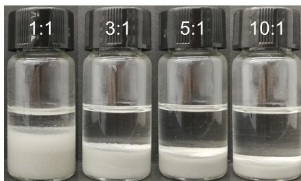
Figure S6. The appearance photos of water in toluene emulsions stabilized by ML-HPMs at different ratio of oil to water: (a) 1:1, (b) 3:1, (c) 5:1 (d)10:1.
