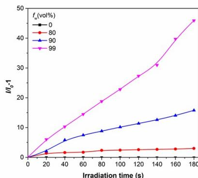
**Figure S6.** Time-dependent changes in fluorescence intensities ( $I/I_0-1$ ) at 523 nm of DCFH/TPA-DCR in THF solutions with different PBS fractions upon white light irradiation ( $40 \text{ mW cm}^{-2}$ ). Concentrations: 10  $\mu\text{M}$  for TPA-DCR and 1  $\mu\text{M}$  for DCFH.
