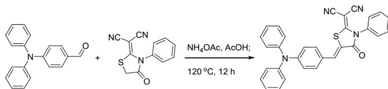
**Scheme S1.** Design and synthesis of the photosensitizer TPA-DCR.
