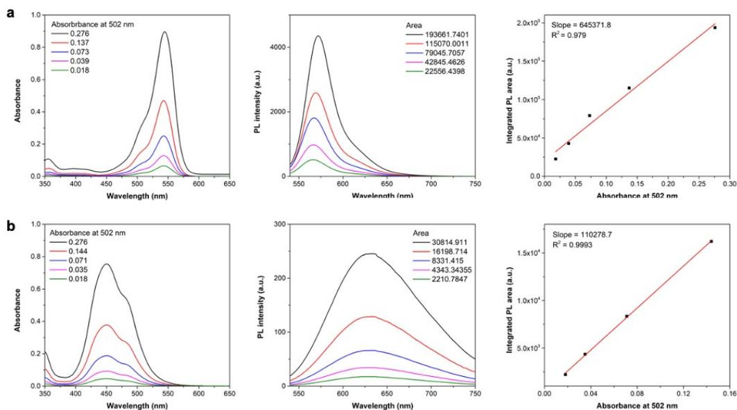
**Figure S9.** Quantum yield measurement of TPA-DCR NPs in water. UV-Vis, PL spectra and integrated emission intensities of (a) Rhodamine B and (b) TPA-DCR NPs in ethanol and water with increasing concentrations, respectively.
