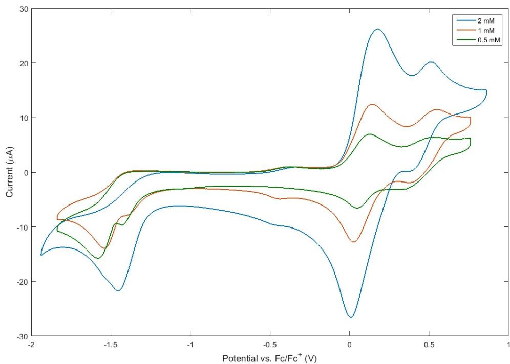
**Figure S57** - Cyclic voltammograms of **2a** at various concentrations.
