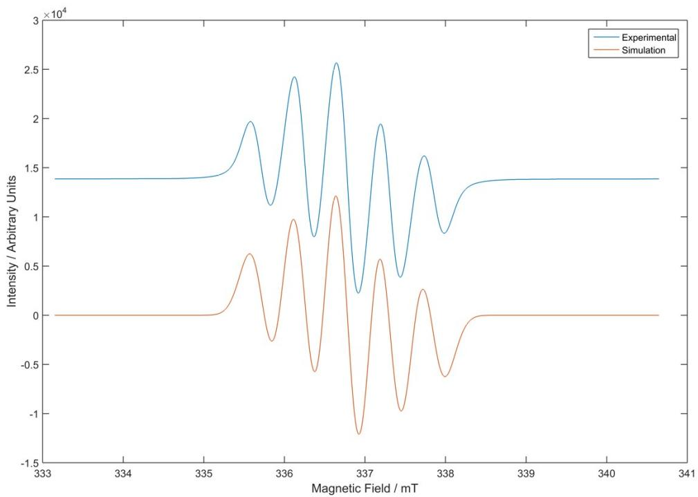
**Figure S44** - EPR spectra of **3h**.  $g$ -value = 2.00449, line width = 0.34 MHz,  $a_{N2}$  = 15.61 MHz,  $a_{N4}$  = 13.71 MHz.
