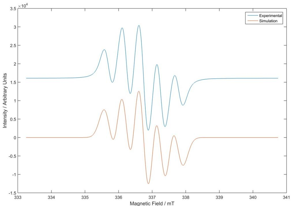
**Figure S41** - EPR spectra of **3e**.  $g$ -value = 2.00463, line width = 0.37 MHz,  $a_{N_2}$  = 14.69 MHz,  $a_{N_4}$  = 13.30 MHz.
