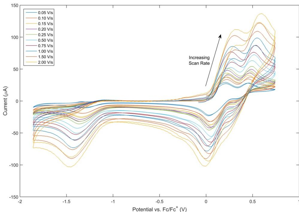
**Figure S58** - Cyclic voltammograms of **2f** at various scan rates.
