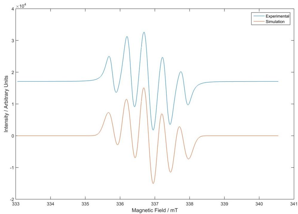
**Figure S42** - EPR spectra of **3f**.  $g$ -value = 2.00453, line width = 0.33 MHz,  $a_{N2}$  = 14.56 MHz,  $a_{N4}$  = 13.23 MHz.
