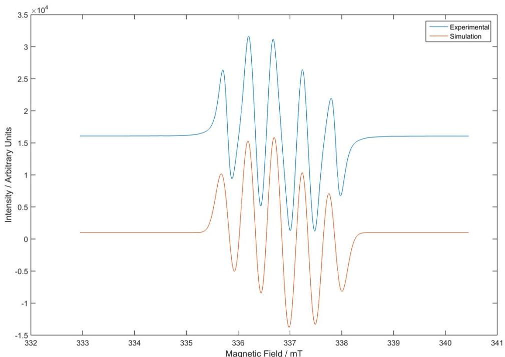
**Figure S45** - EPR spectra of **3i**.  $g$ -value = 2.00410, line width = 0.29 MHz,  $a_{N2}$  = 15.82 MHz,  $a_{N4}$  = 12.89 MHz.
