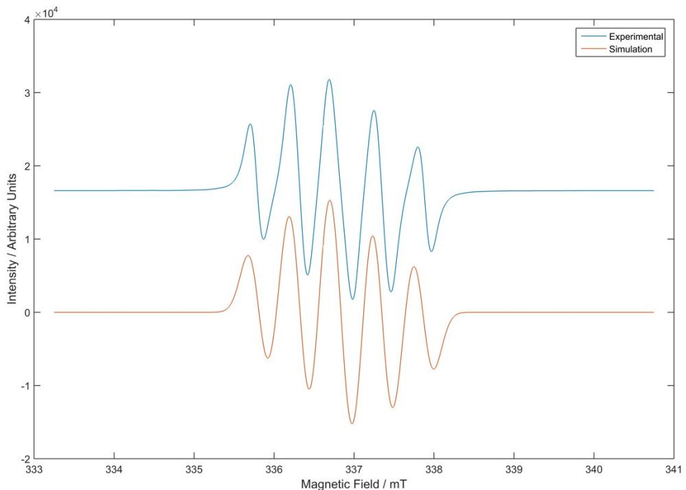
**Figure S37** - EPR spectra of **3a**.  $g$ -value = 2.00369, line width = 0.27 MHz,  $a_{N2}$  = 15.56 MHz,  $a_{N4}$  = 13.13 MHz.
