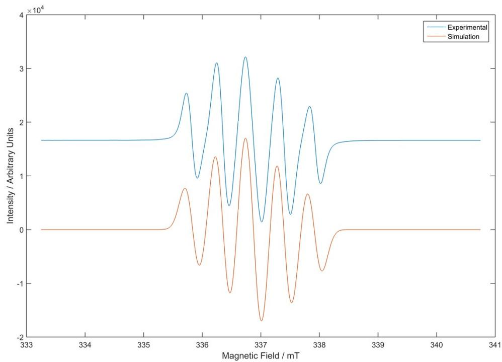
**Figure S38** - EPR spectra of **3b**.  $g$ -value = 2.00346, line width = 0.26 MHz,  $a_{N2}$  = 15.64 MHz,  $a_{N4}$  = 13.51 MHz.
