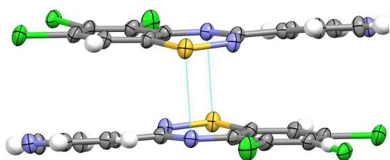
**Figure S34** - Crystal structure of **3k** - Side view of radical dimerisation.
