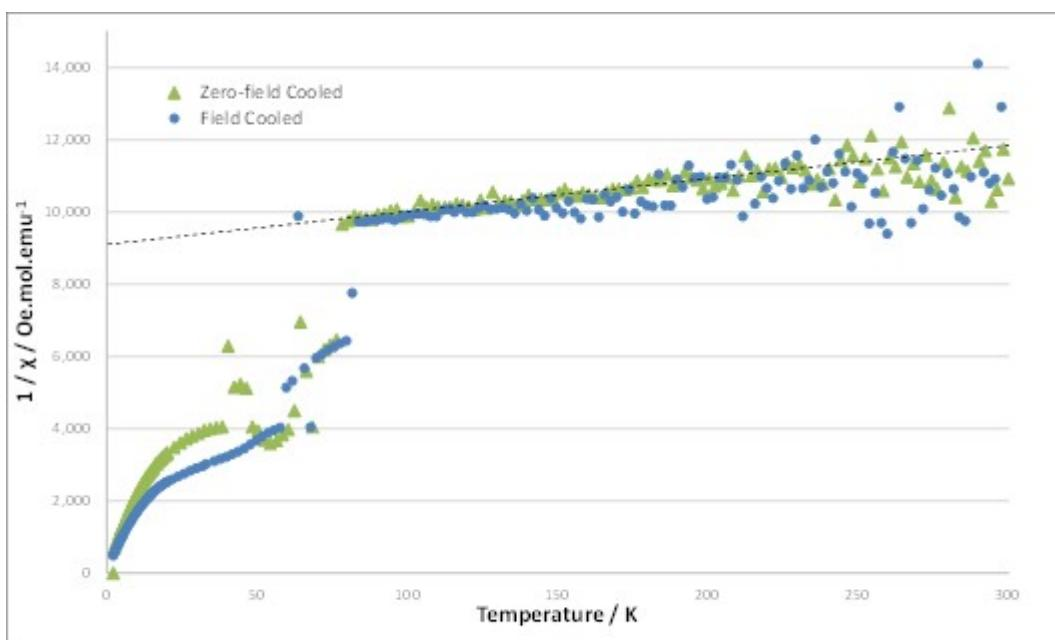
Figure S60 – Curie-Weiss plot for **3c**, recorded in a field of 1000 Oe.
