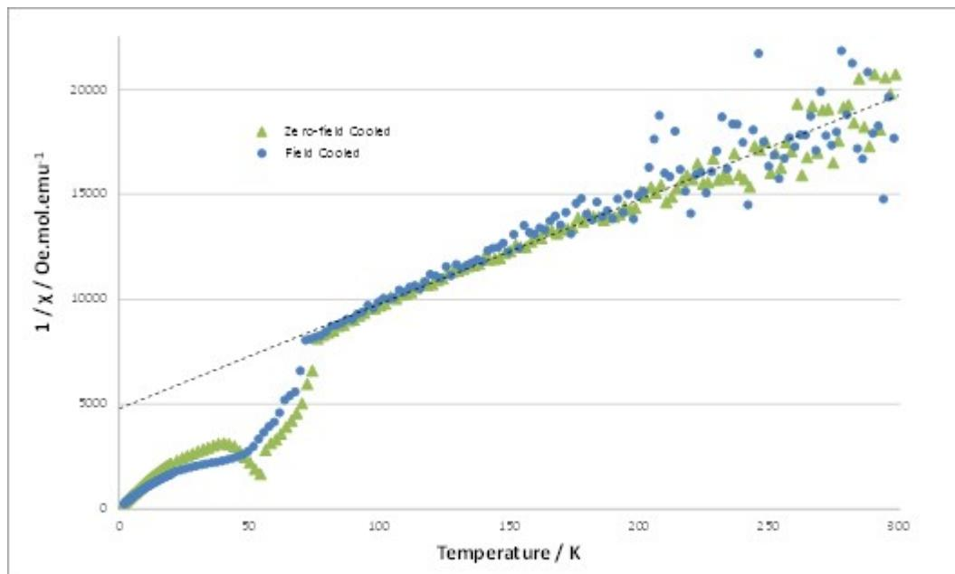
**Figure S61** – Curie-Weiss for **3e**, recorded in a field of 1000 Oe.
