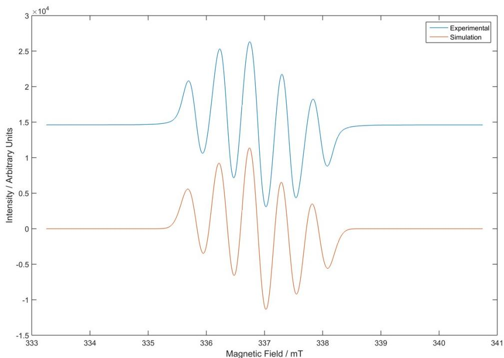
**Figure S39** - EPR spectra of **3c**.  $g$ -value = 2.00341, line width = 0.31 MHz,  $a_{N2}$  = 15.80 MHz,  $a_{N4}$  = 13.60 MHz.
