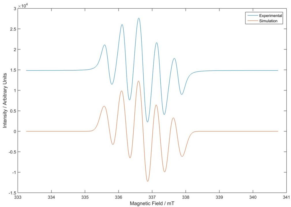
**Figure S40** - EPR spectra of **3d**.  $g$ -value = 2.00431, line width = 0.31 MHz,  $a_{N_2}$  = 15.10 MHz,  $a_{N_4}$  = 13.10 MHz.
