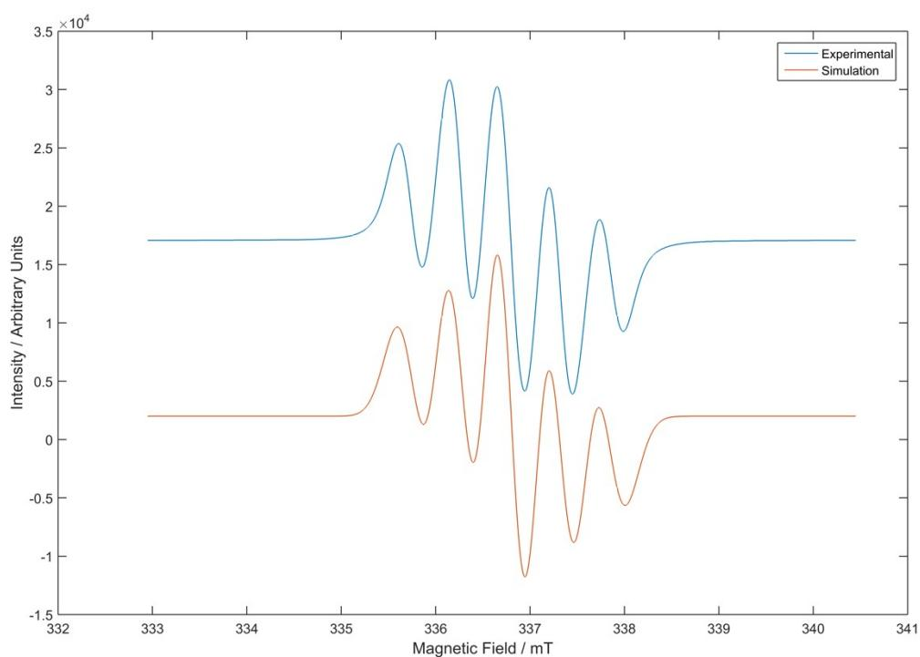
**Figure S46** - EPR spectra of **3j**.  $g$ -value = 2.00411, line width = 0.38 MHz,  $a_{N2}$  = 14.73 MHz,  $a_{N4}$  = 13.98 MHz.
