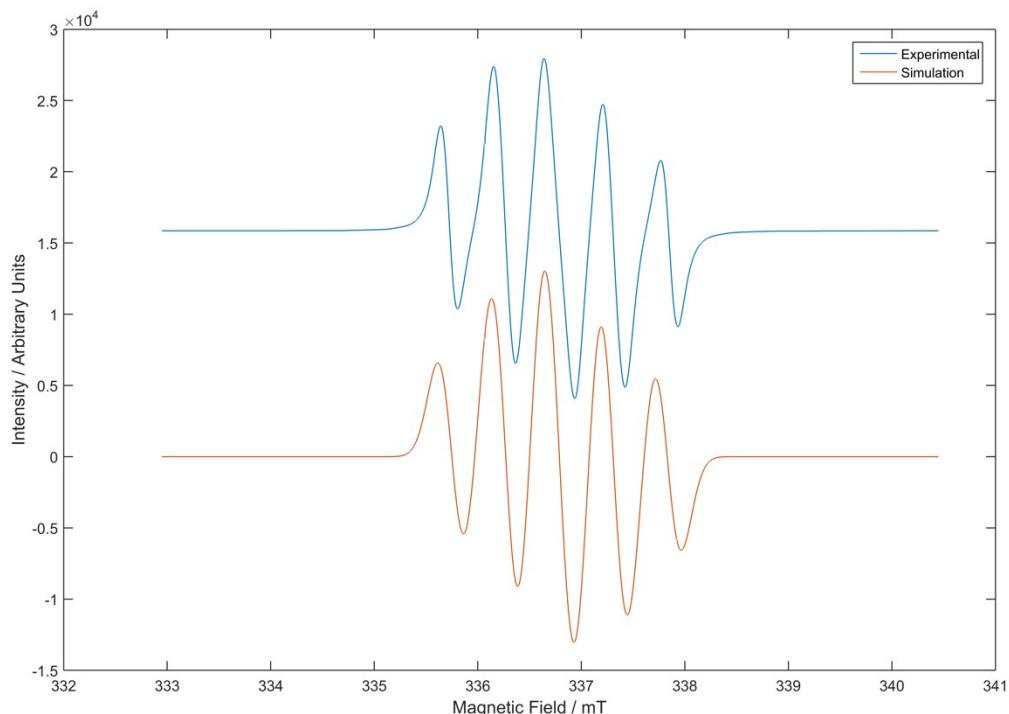
**Figure S43** - EPR spectra of **3g**.  $g$ -value = 2.00461, line width = 0.27 MHz,  $a_{N2}$  = 15.88 MHz,  $a_{N4}$  = 13.35 MHz.
