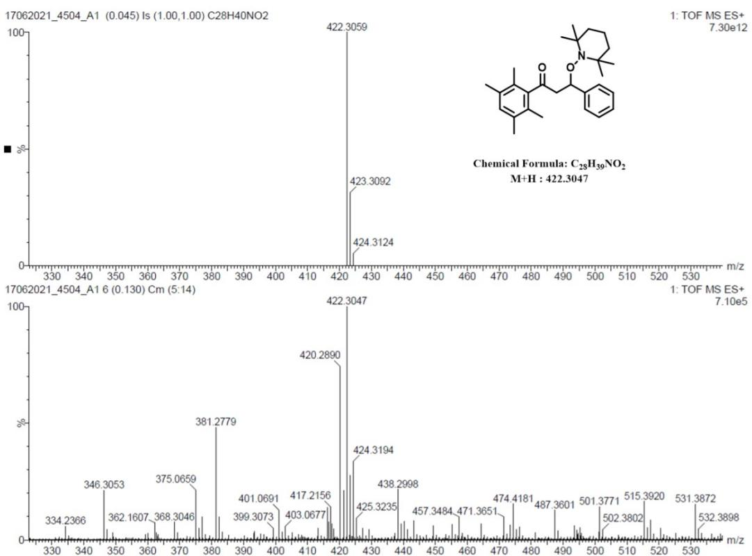
**Figure S3.** Mass spectrum of ketyl-TEMPO adduct. HRMS (ESI) m/z: [M + H]<sup>+</sup> Calcd for C<sub>28</sub>H<sub>39</sub>NO<sub>2</sub> 422.3059; Found 422.3047; (Bottom spectrum is experimentally observed and top one is simulated.)
