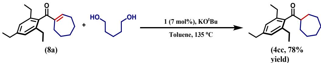
A 15 mL pressure tube was charged with 7 mol% of **1**, 0.5 mmol of cyclohex-1-en-1-yl(2,4,6-triethylphenyl) methanone (**8a**), 1 mmol of 1,5-pentanediol, KO<sup>t</sup>Bu (1 mmol) in 5 mL toluene. The reaction flask was purged with an inert gas for few minutes before closing
