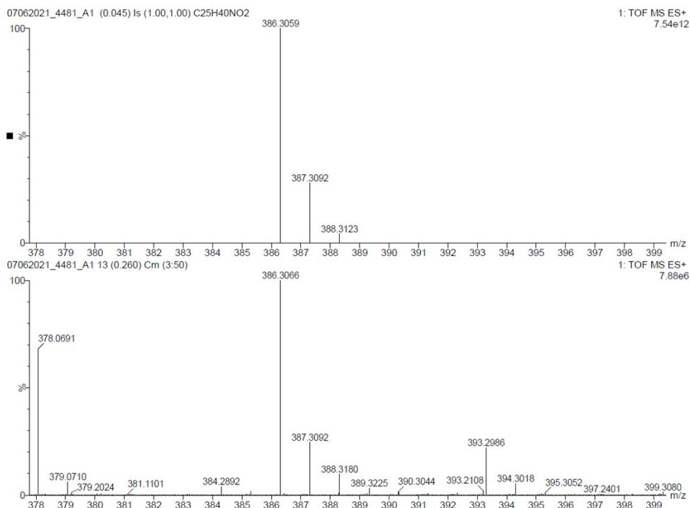
**Figure S1.** Mass spectrum of radical arrested TEMPO intermediate. (Bottom spectrum is experimentally observed and top one is simulated.)
