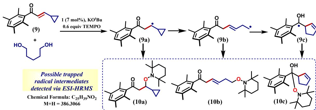
A 15 mL pressure tube was charged with 7 mol% of **1**, 0.5 mmol of **3**-cyclopropyl-1-(2,3,5,6-tetramethylphenyl)prop-2-en-1-one (**10**), 1 mmol of 1,5-pentanediol, KOtBu (0.5 mmol) in 5
