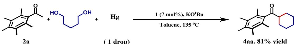
To establish the homogeneity of the **1**, we have carried out a mercury drop experiment.
