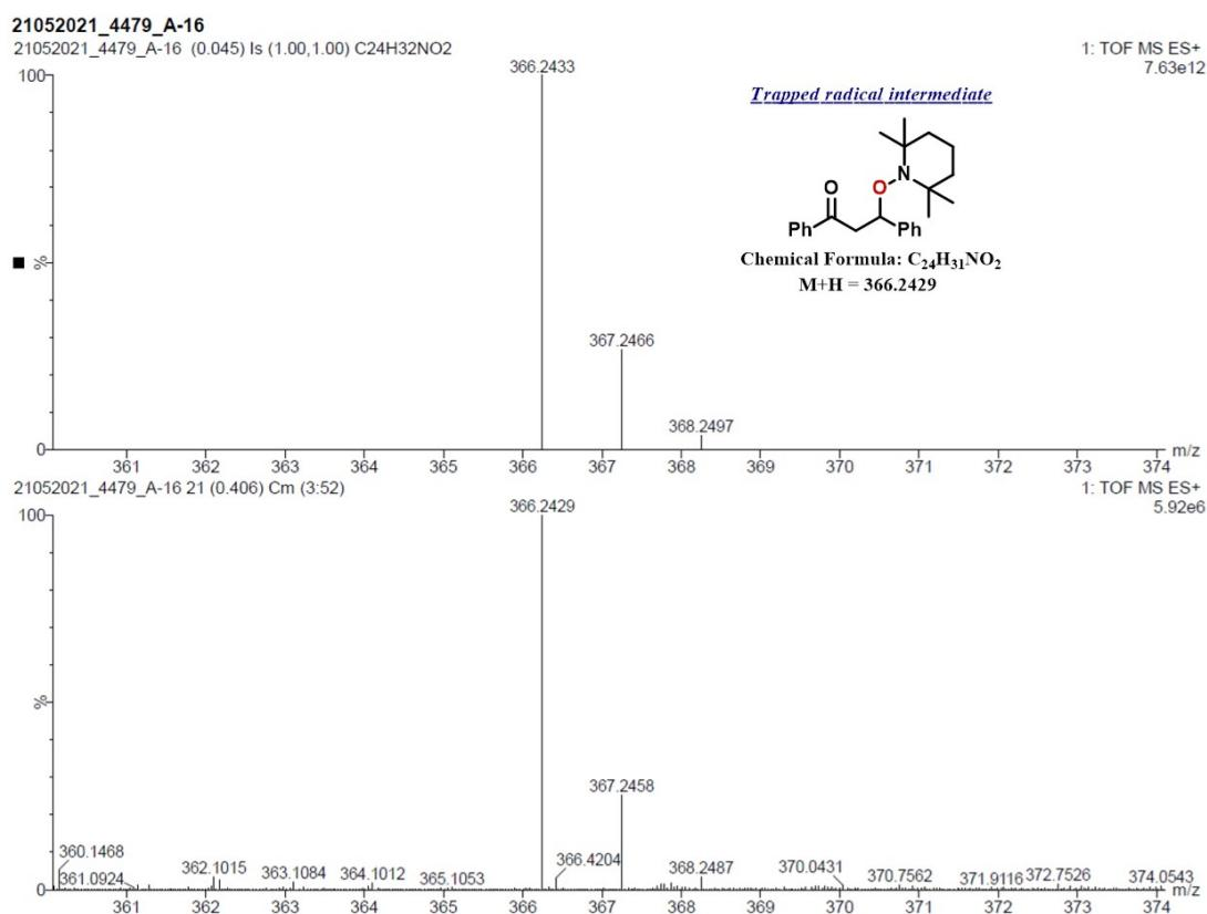
**Figure S2.** Mass spectrum of ketyl-TEMPO adduct. ESI-HRMS m/z: [M + H]<sup>+</sup> Calcd for C<sub>24</sub>H<sub>31</sub>NO<sub>2</sub> 366.2433; Found 366.2429; (Bottom spectrum is experimentally observed and top one is simulated.)
