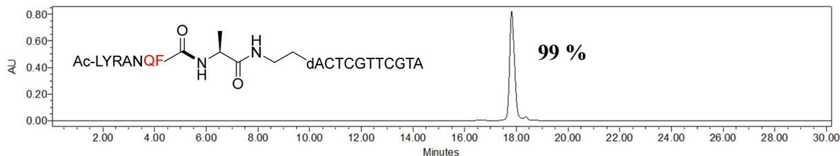
**Figure S28:** IEX HPLC trace of IEX purified LYRANM POC. The column was monitored at 260 nm and eluted at room temperature using a linear gradient of 0-52 % buffer B over 30 minutes (buffer A: 100 mM Tris HCl, pH 7.5, 10 % acetonitrile; buffer B: 100 mM Tris HCl, pH 7.5, 10 % acetonitrile, 1 M NaCl).
