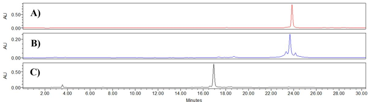
**Figure S25:** IEX HPLC trace of IEX purified LYRANSA POC. The column was monitored at 260 nm and eluted at room temperature using a linear gradient of 0-52 % buffer B over 30 minutes (buffer A: 100 mM Tris HCl, pH 7.5, 10 % acetonitrile; buffer B: 100 mM Tris HCl, pH 7.5, 10 % acetonitrile, 1 M NaCl).
