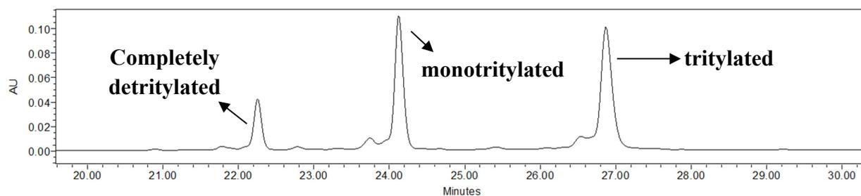
**Figure S5:** IEX HPLC trace of pure detritylated and desalted diselenide oligonucleotide **7**. The column was monitored at 260 nm and eluted at room temperature using a linear gradient of 0-52 % buffer B over 30 minutes (buffer A: 100 mM Tris HCl, pH 7.5, 10 % acetonitrile; buffer B: 100 mM Tris HCl, pH 7.5, 10 % acetonitrile, 1 M NaCl).
