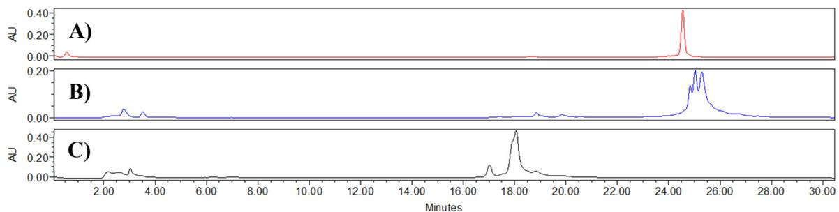
**Figure S23:** IEX HPLC traces of A) pure diselenide oligonucleotide **14** B) 3 hour aliquot of rDSL between diselenide oligonucleotide **14** and selenoester peptide **16** (Ac-LYRANQF-SePh) and C) 3 hour aliquot of deselenization following rDSL. The column was monitored at 260 nm and eluted at room temperature using a linear gradient of 0-52 % buffer B over 30 minutes (buffer A: 100 mM Tris HCl, pH 7.5, 10 % acetonitrile; buffer B: 100 mM Tris HCl, pH 7.5, 10 % acetonitrile, 1 M NaCl).
