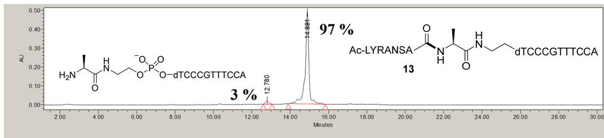
**Figure S14:** IEX HPLC traces of A) crude POC **13** B) RP-purified POC **13** and C) RP and IEX purified POC **13**. The deselenized starting material is identified with an arrow. The column was monitored at 260 nm and eluted at room temperature using a linear gradient of 0-52 % buffer B over 30 minutes (buffer A: 100 mM Tris HCl, pH 7.5, 10 % acetonitrile; buffer B: 100 mM Tris HCl, pH 7.5, 10 % acetonitrile, 1 M NaCl).
