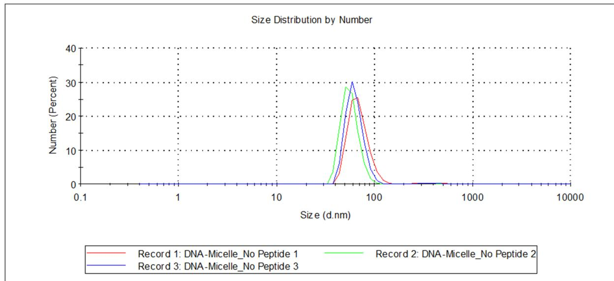
**Figure S37:** DLS measurements of unmodified oligonucleotide dTCCCGTTTCCA. Solution contained oligonucleotide at a concentration of 100  $\mu$ M prepared in a buffer of 0.1 M MES, pH 6.7. Average particle size: 1.5 nm. Average PDI: 0.66.
