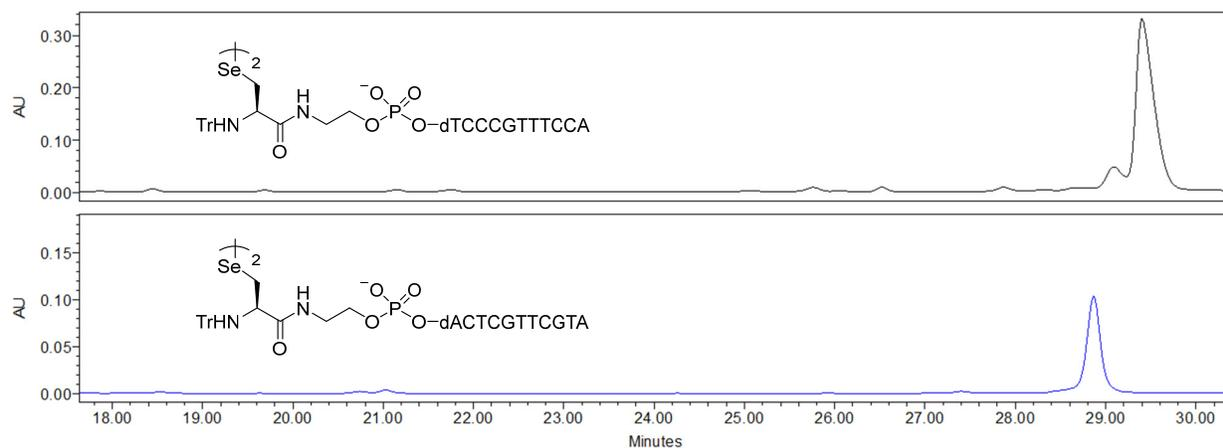
**Figure S8:** IEX HPLC trace of pure detritylated and desalted diselenide oligonucleotide **14**. The column was monitored at 260 nm and eluted at room temperature using a linear gradient of 0-52 % buffer B over 30 minutes (buffer A: 100 mM Tris HCl, pH 7.5, 10 % acetonitrile; buffer B: 100 mM Tris HCl, pH 7.5, 10 % acetonitrile, 1 M NaCl).
