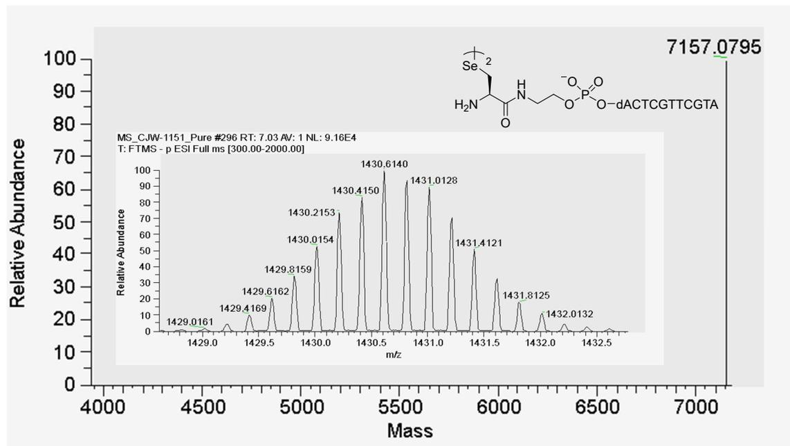
**Figure S10:** ESI-MS spectrum of 1 hour aliquot of rDSL between diselenide oligonucleotide **7** and selenoester peptide **8**. Intermediates **9-12** are identified.
