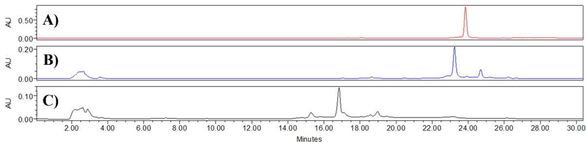
**Figure S22:** IEX HPLC traces of A) pure diselenide oligonucleotide **14** B) 3 hour aliquot of rDSL between diselenide oligonucleotide **14** and selenoester peptide **15** (Ac-LYRANYF-SePh) and C) 3 hour aliquot of deselenization following rDSL. The column was monitored at 260 nm and eluted at room temperature using a linear gradient of 0-52 % buffer B over 30 minutes (buffer A: 100 mM Tris HCl, pH 7.5, 10 % acetonitrile; buffer B: 100 mM Tris HCl, pH 7.5, 10 % acetonitrile, 1 M NaCl).
