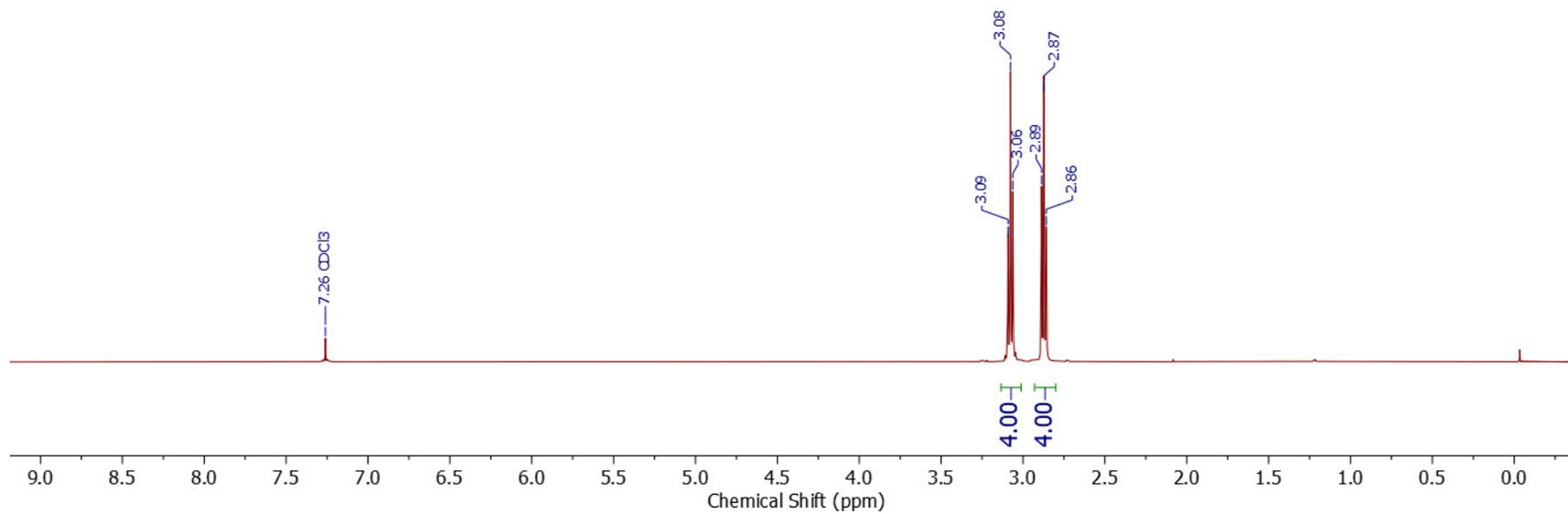
**Figure S51:** 95.3 MHz  $^{77}\text{Se}$  NMR spectrum of di-2-cyanoethyl diselenide (in  $\text{CDCl}_3$ )
