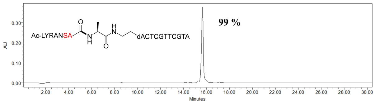
**Figure S26:** IEX HPLC trace of IEX purified LYRANYF POC. The column was monitored at 260 nm and eluted at room temperature using a linear gradient of 0-52 % buffer B over 30 minutes (buffer A: 100 mM Tris HCl, pH 7.5, 10 % acetonitrile; buffer B: 100 mM Tris HCl, pH 7.5, 10 % acetonitrile, 1 M NaCl).
