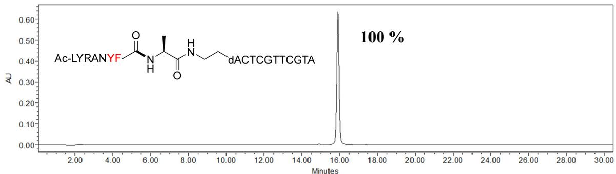
**Figure S27:** IEX HPLC trace of IEX purified LYRANQF POC. The column was monitored at 260 nm and eluted at room temperature using a linear gradient of 0-52 % buffer B over 30 minutes (buffer A: 100 mM Tris HCl, pH 7.5, 10 % acetonitrile; buffer B: 100 mM Tris HCl, pH 7.5, 10 % acetonitrile, 1 M NaCl).
