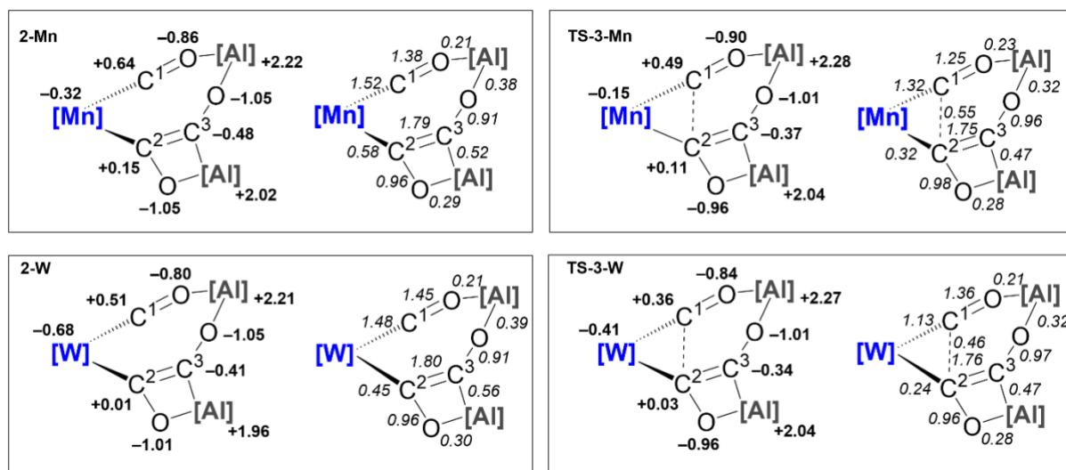
**Figure S18:** Comparison of calculated NBO data of **2-Mn** and **TS-3-Mn** with **2-W** and **TS-3-W**. Natural charges provided in **bold** and Wiberg bond indices provided in *italics*.
