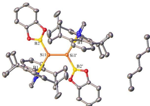
**Figure S13.** OLEX2 drawing of **4** with 50% ellipsoid probability. Hydrogen atoms have been omitted for clarity. Selected bond lengths ( $\text{\AA}$ ) and angles ( $^\circ$ ): Si1–Si1' 2.1654(12), Si1–B1 1.991(3), Si1–B2 1.983(3); B1–Si1–B3 145.82(8), B1–Si1–Si1' 120.49(8), B2–Si1–Si1' 118.70(9), B2–Si1–B1 120.78(10).
