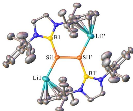
**Figure S1.** OLEX2 drawing of **2** with 50% ellipsoid probability. Hydrogen atoms have been omitted for clarity. Selected bond lengths (Å) and angles (°): Si1–Si1' 2.223(3), Si1–B1 2.022(6), Si1–Li1 2.474(10); Si1'-Si1–Li1 117.3(3), B1–Si1–Si1' 109.6(2), B1–Si1–Li1 132.6(3).
