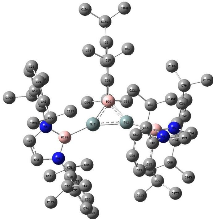
**Figure S10.** Optimized geometry of **3c**. Selected computed bond lengths ( $\text{\AA}$ ) and angles (deg): Si1–Si2 2.16784, Si1–B95 1.94802, Si2–B95 1.94802; B95–Si2–Si1 56.19135, B95–Si1–Si2 56.19127, Si1–B82–Si2 67.61737.
