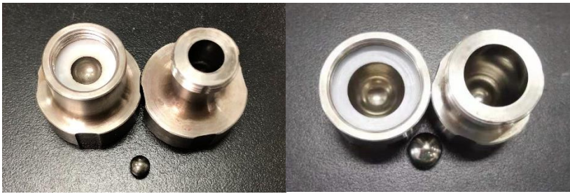
Figure S2. Stainless jar (1.5 mL, left; 5 mL, right) and ball (5 mm, left; 15 mm, right) used in this study.
