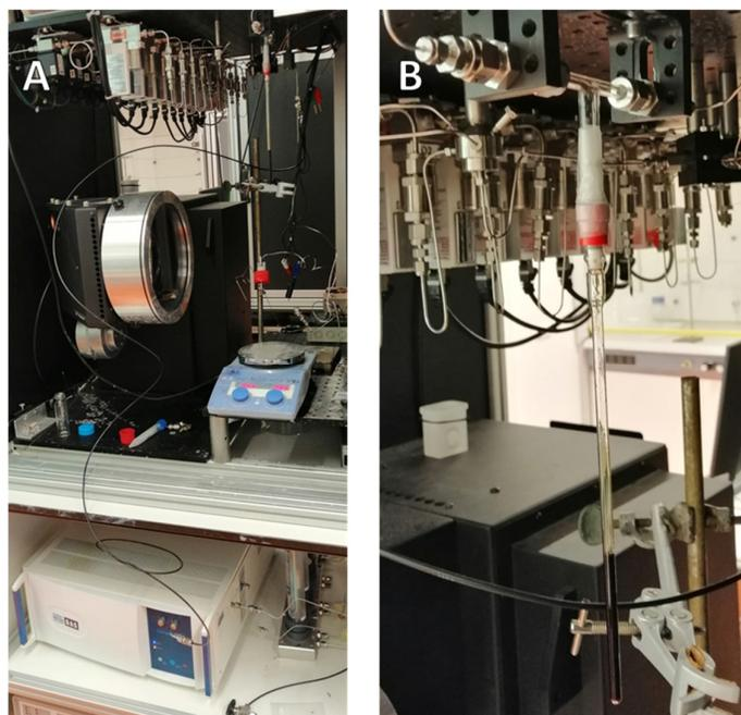
Figure S85: Headspace analysis by GC. (A) set-up showing both the GC (below) and the gas inlets/outlets (up). (B) NMR sample connected to the carrier gas inlet with an adaptor.
